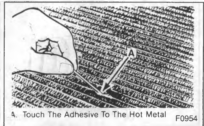
Figure 33—Applying Hot-Melt Adhesive to the Repair Area
