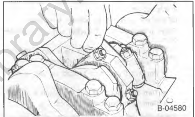
Figure 28 — Checking Connecting Rod Side Clearance
