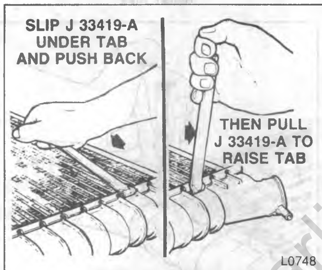
Figure 36—Opening the Clinch Tabs
