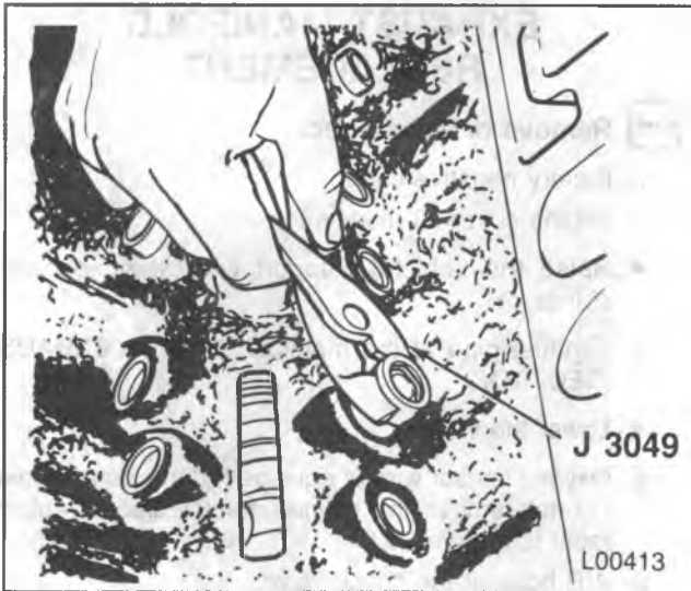
Figure 10 — Removing the Hydraulic Lifter
