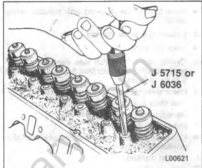
Figure 12 — Reaming the Rocker Arm Stud Bore (Typical)
