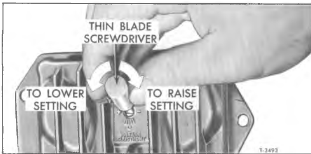
Figure 15—Adjusting Voltage Setting (Typical)
