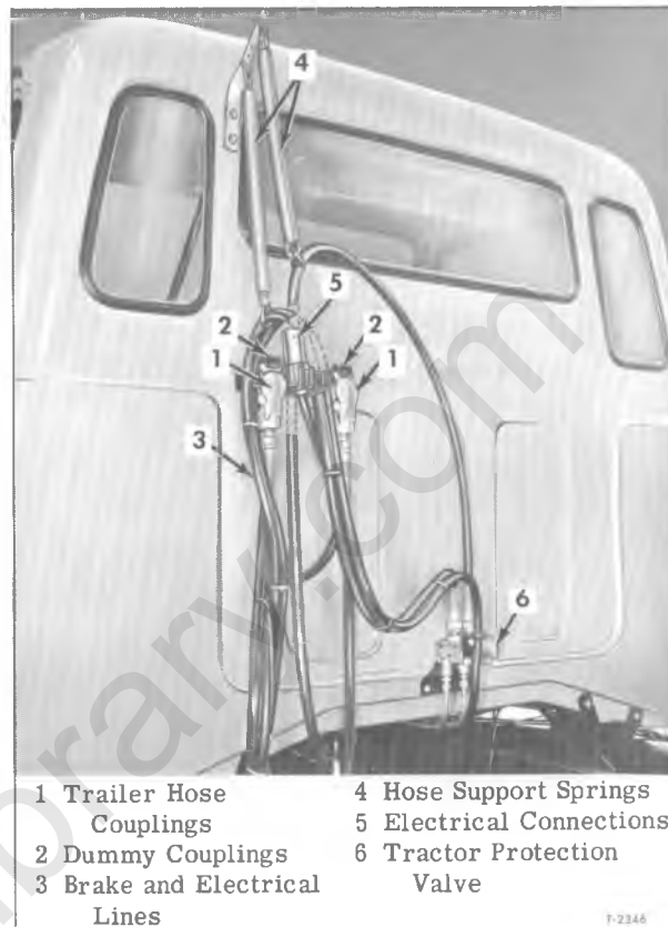
Figure 15—Trailer Brake Connections
