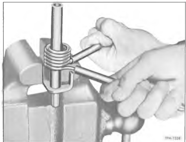
Figure 20—Removing Torsion Spring (Rockwell)
