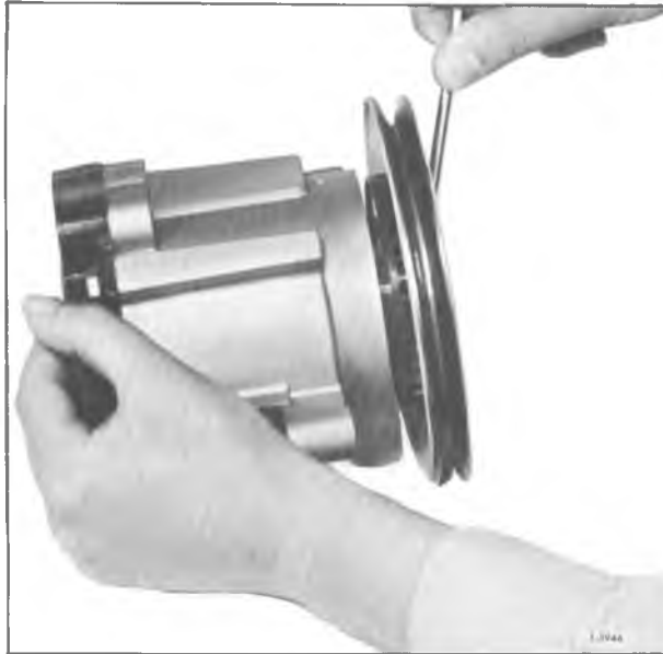
Figure 36—Installing Centrifugal Filter
