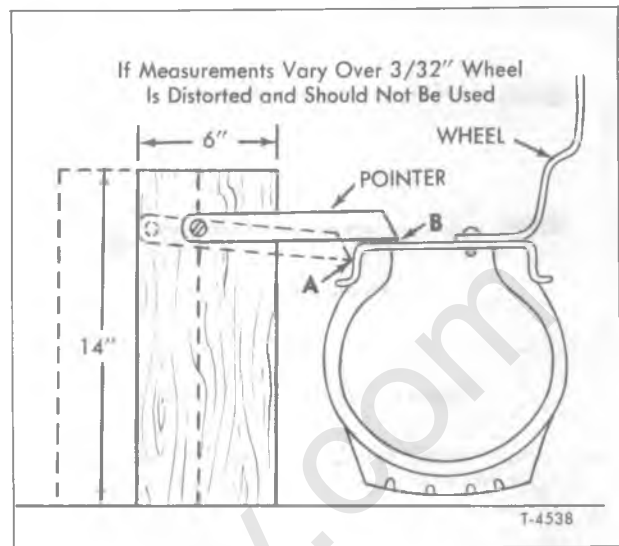
Figure 4—Method of Checking for Distorted Wheels
