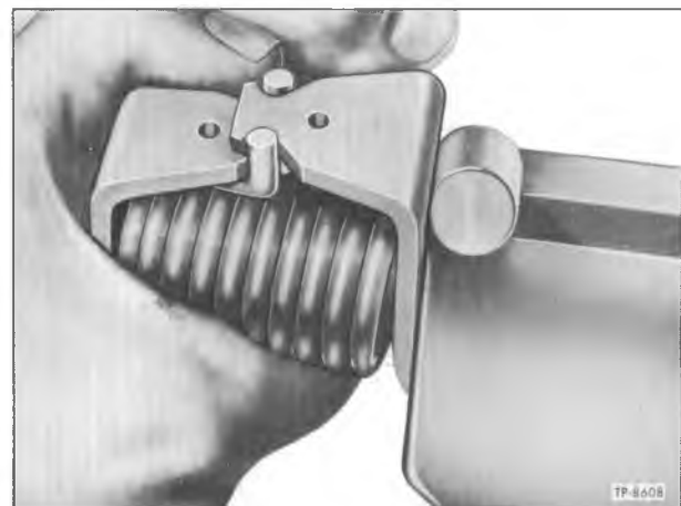
Figure 17—Disassembling Torsion Spring from Lever
