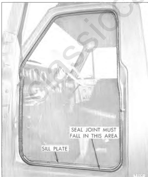
Figure 12—Door Weatherstrip Installed
