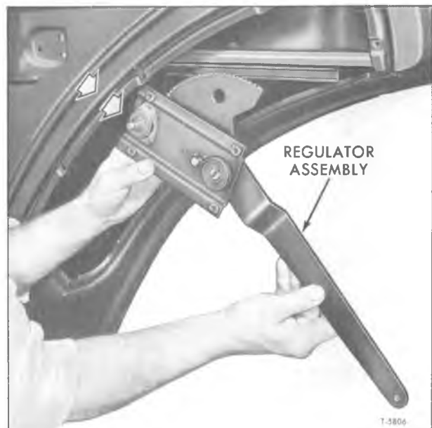
Figure 19—Lowering Regulator from Door
