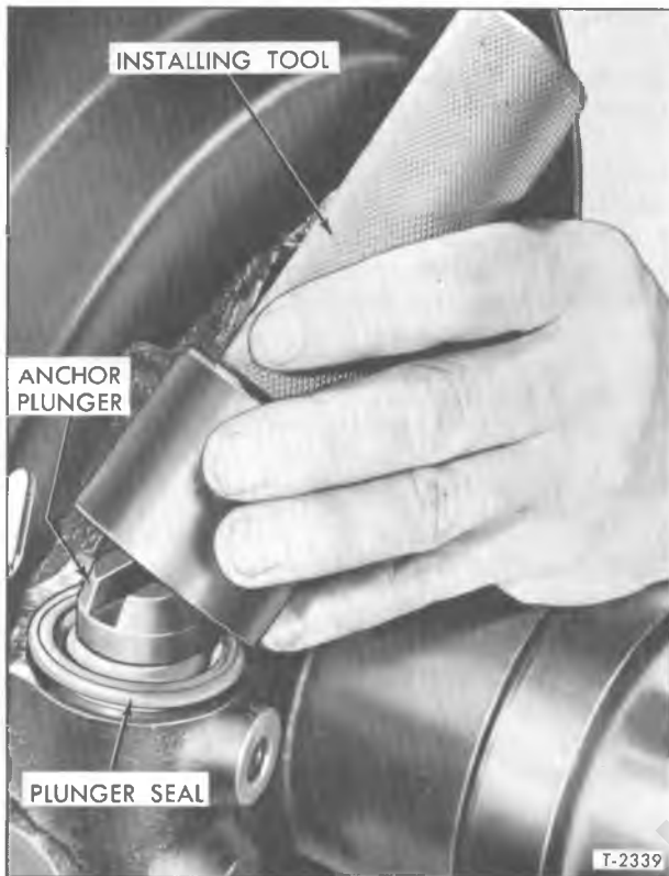
Figure 36—Installing Anchor Plunger and Seal
