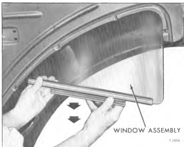
Figure 20—Removing Door Window Glass
