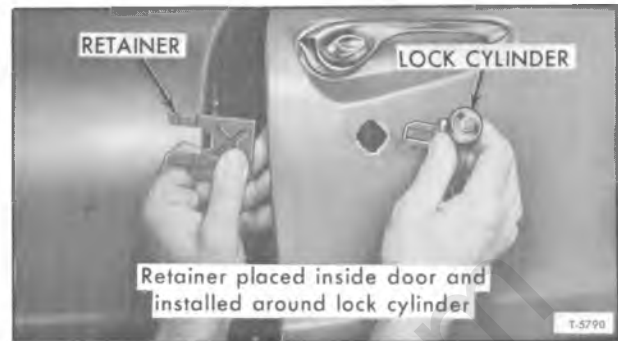
Figure 14—Door Lock Cylinder Replacement
