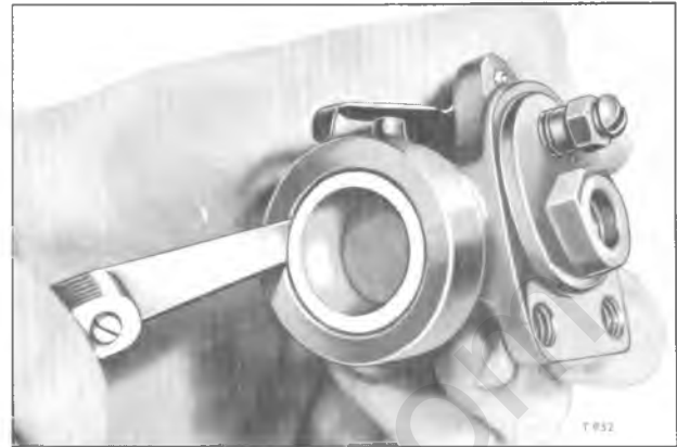
Figure 15—Checking Fit of Piston in Wheel Cylinder
