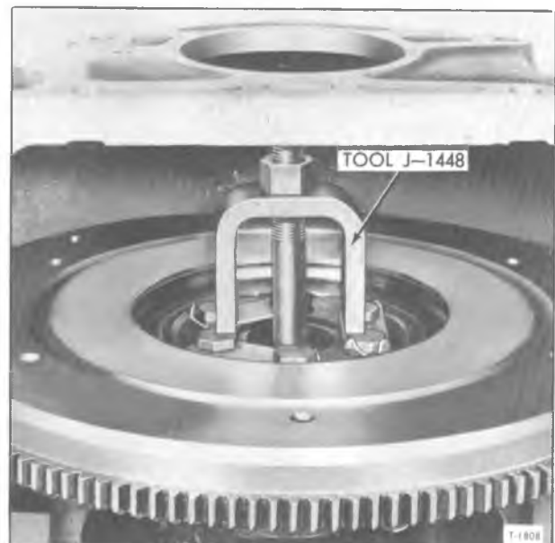
Figure 4—Pilot Bushing Removal
