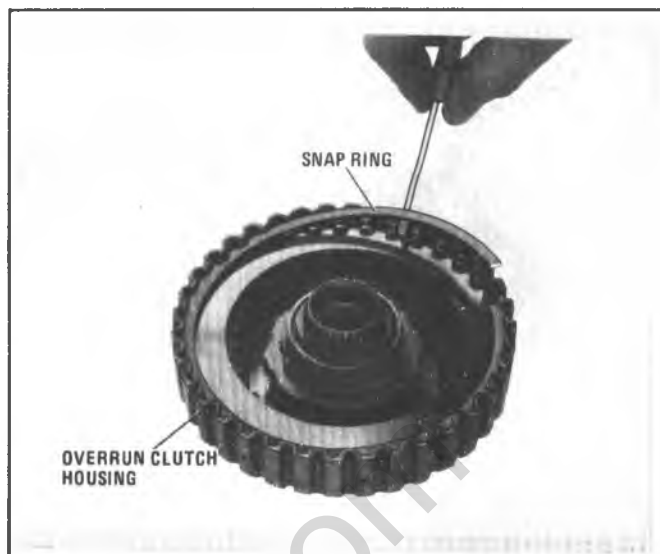
Figure 7A6-175 Removing Overrun Clutch Snap Ring
