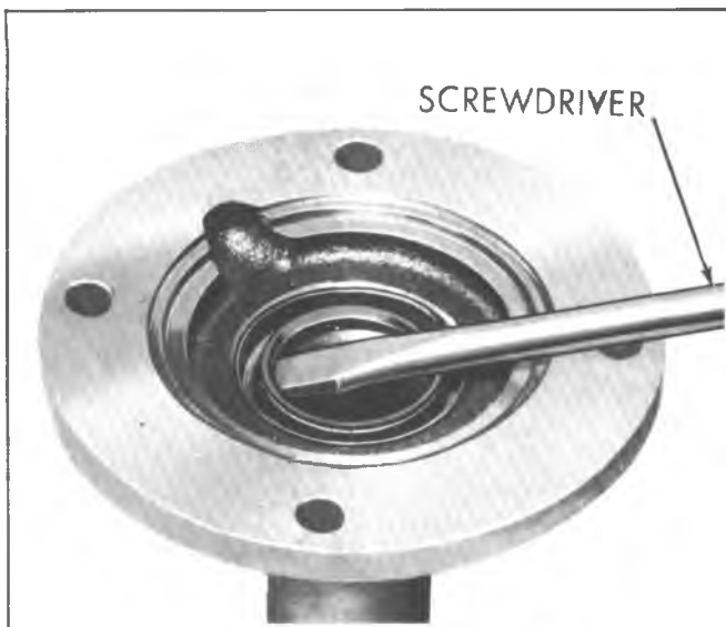
Fig. 7B-14J—Removing Bearing Retainer Oil Seal
