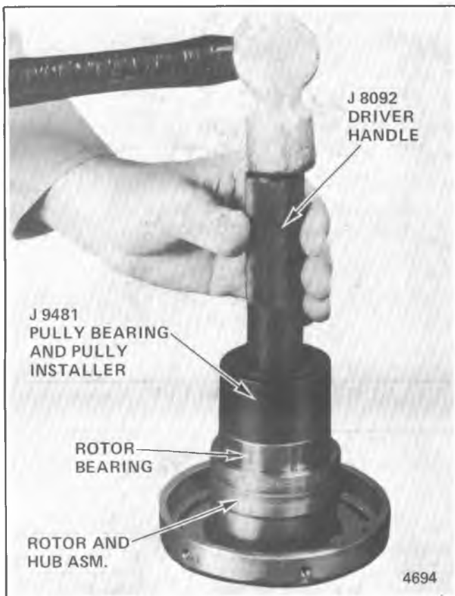
Fig. 1D-81 Installing R-4 Clutch Rotor Bearing
