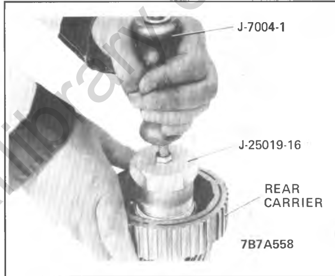
Figure 7A1-212 Removing Rear Carrier Bushing
