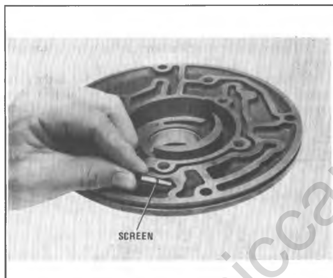
Figure 7A1-146 Removing Screen
