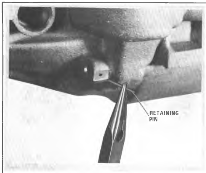
Figure 7A6-76 Removing Parking Pawl Shaft Pin
