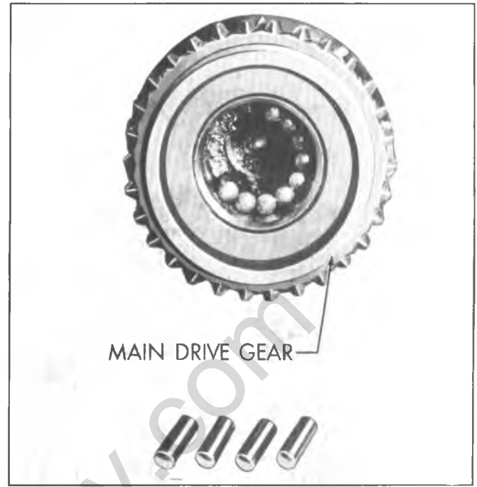
Fig. 7B-20J--Loading Mainshaft Bearings
