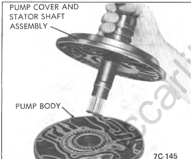
Figure 7A3-68 Pump Cover Removal
