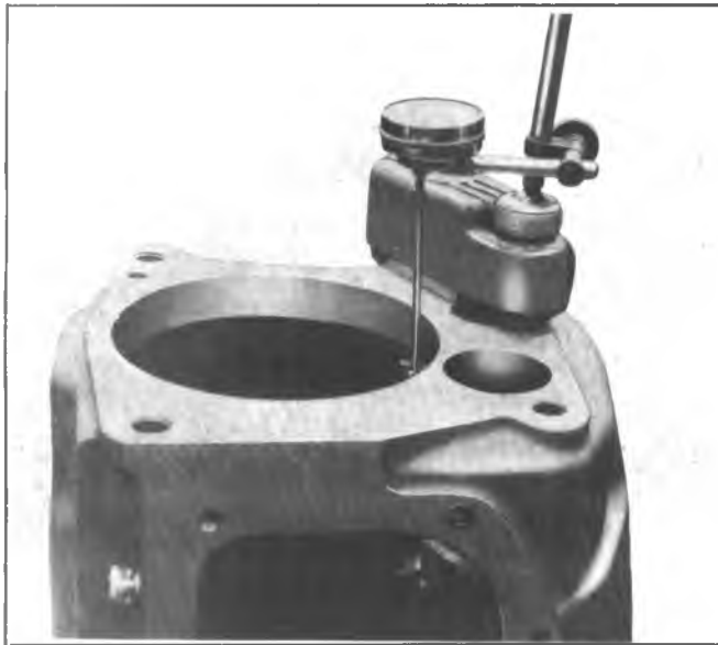
Fig. 7B-20K--Checking Countergear End Play
