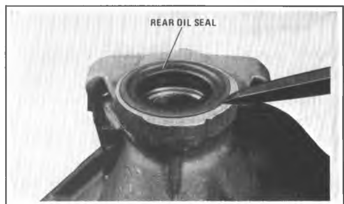
Figure 7A6-70 Removing Rear Oil Seal
