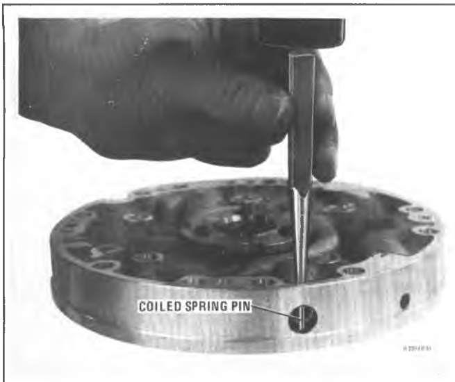
Figure 7A6-205 Removing Pressure Relief Spring Retaining Sleeve
