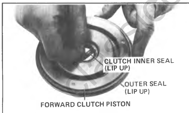
Figure 7A1-124 Removing or Installing Inner Piston Seal
