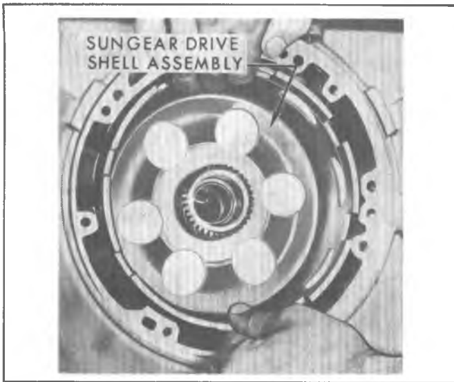
Figure 7A5-30 Sun Gear Drive Shell Removal
