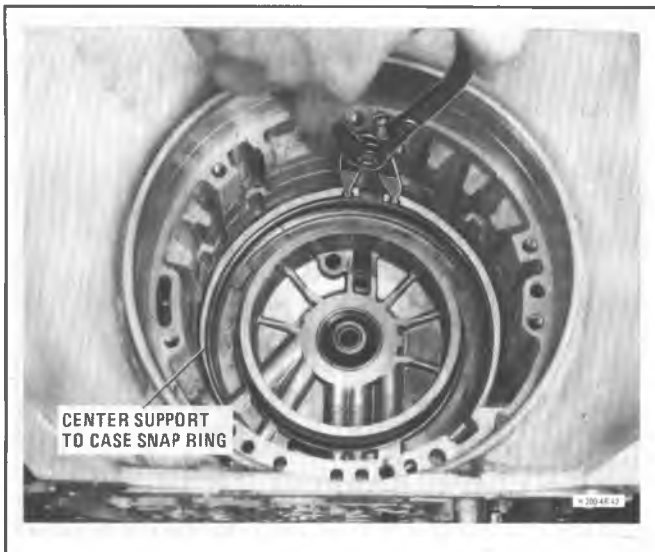
Figure 7A6-159 Installing Center Support Snap Ring
