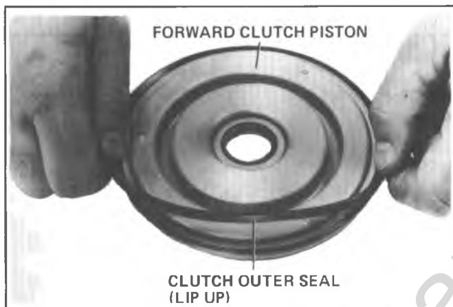
Figure 7A1-123 Removing or Installing Outer Piston Seal
