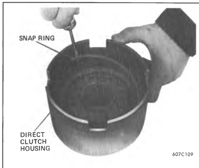
Figure 7A1-110 Removing Direct Clutch Snap Ring
