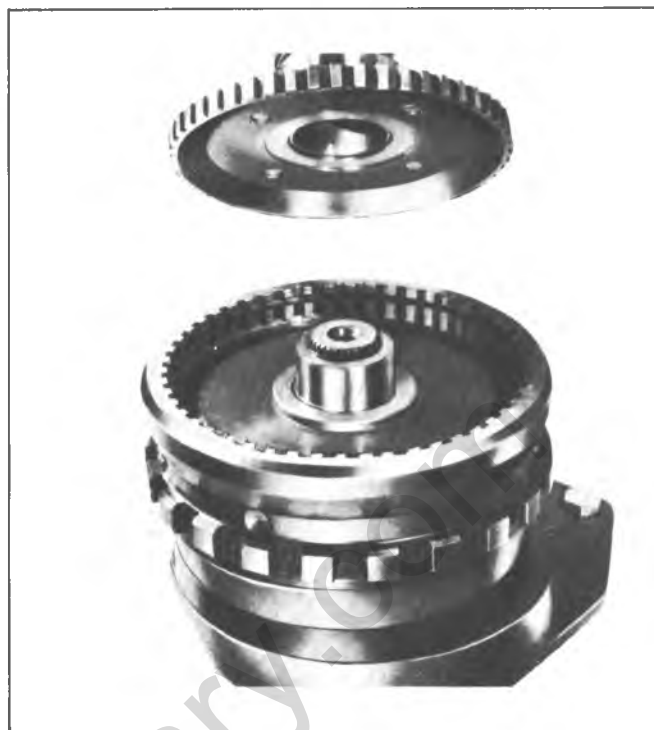
Fig. 7A-145C--Installing Output Shaft
