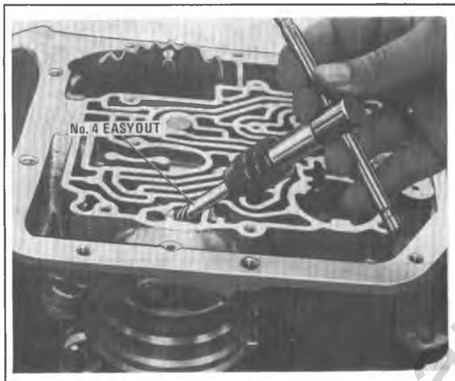
Figure 7A1-25 Removing 3rd Accumulator Check Valve Assy.
