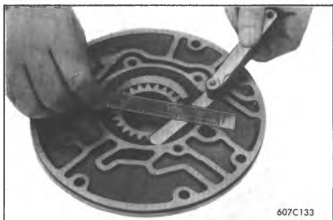
Figure 7A1-151 Checking Pump Body-to-Gear End Clearance
