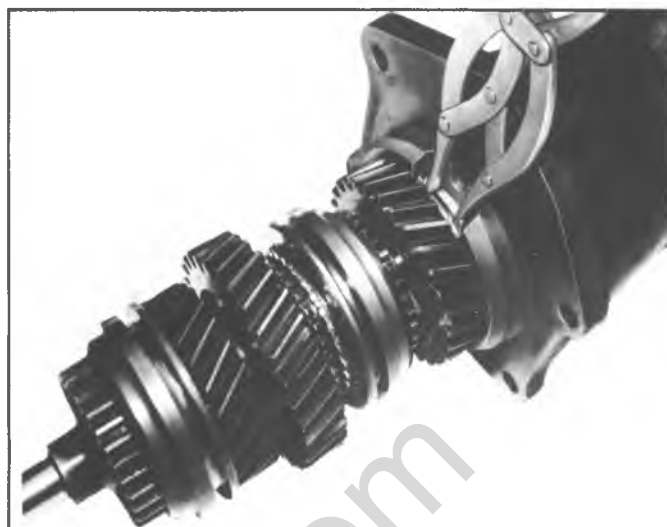
Fig. 7B-4A--Removing Rear Extension From Main Shaft
