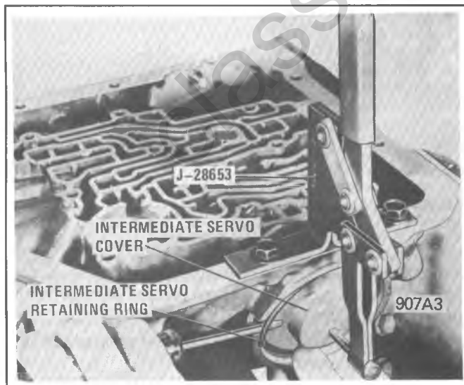
Figure 7A1-174 Installing Intermediate Servo Cover Retaining Ring
