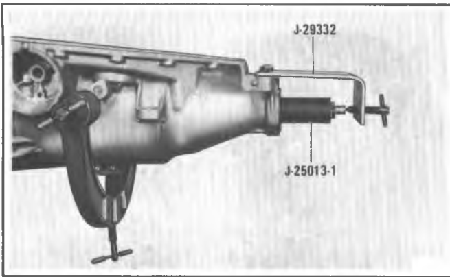
Figure 7A6-56 Installing Tools on Rear of Case
