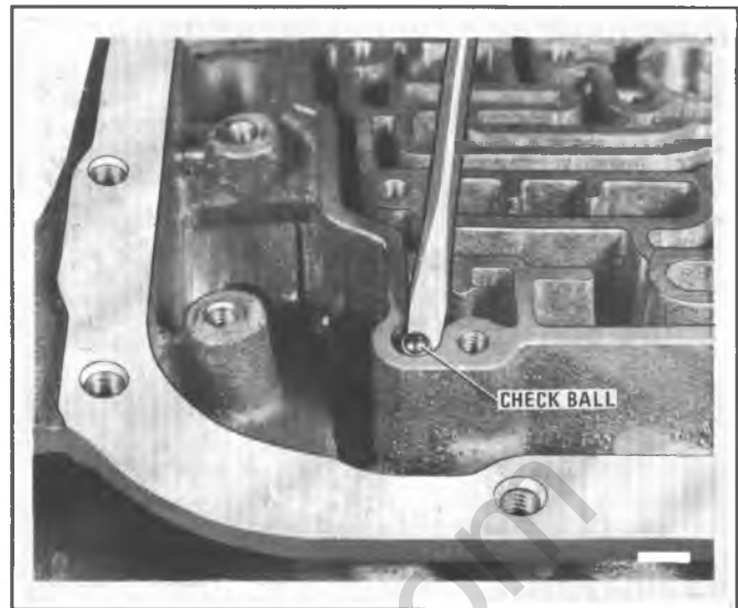
Figure 7A6-19 Removing Check Balls from Case
