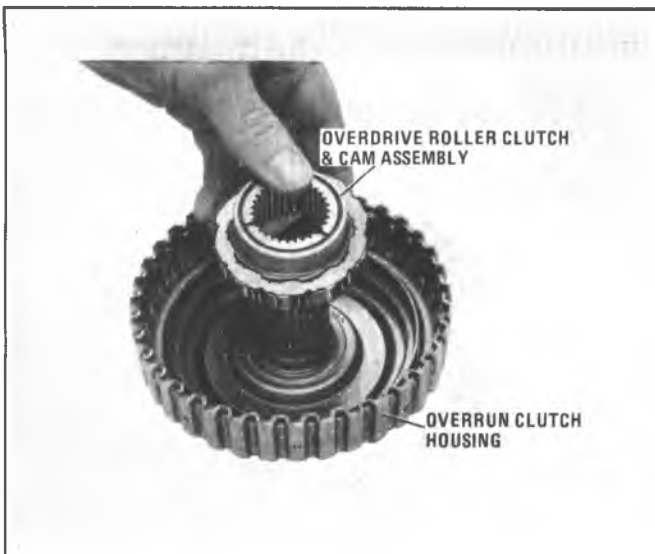
Figure 7A6-178 Removing Overdrive Roller Clutch Cam Assembly
