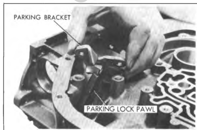
Fig. 7A-23C--Removing Parking Bracket
