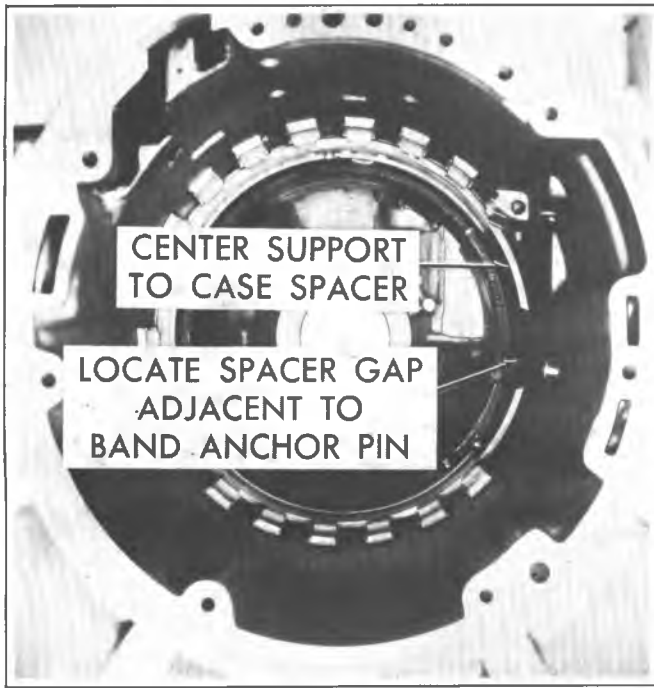
Fig. 7A-44C--Removing Center Support to Case Spacer
