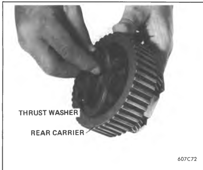
Figure 7A1-76 Installing Thrust Washer Into Rear Carrier
