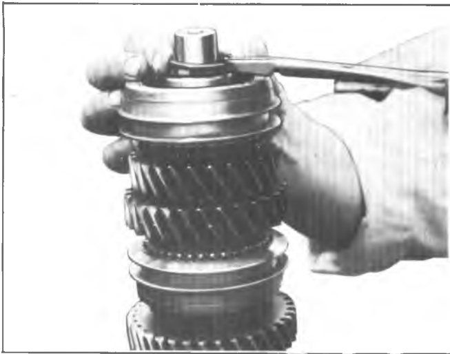
Fig. 7B-9K—Removing 3-4 Clutch Assembly Retainer
