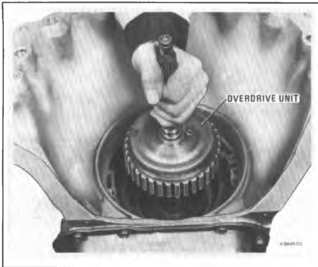
Figure 7A6-197 Installing Overdrive Unit
