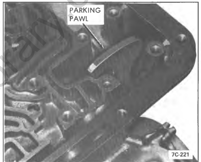
Figure 7A3-139 Install Parking Pawl
