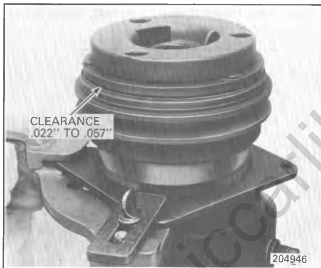
Fig. 1D-8 Checking A-6 Air Gap
