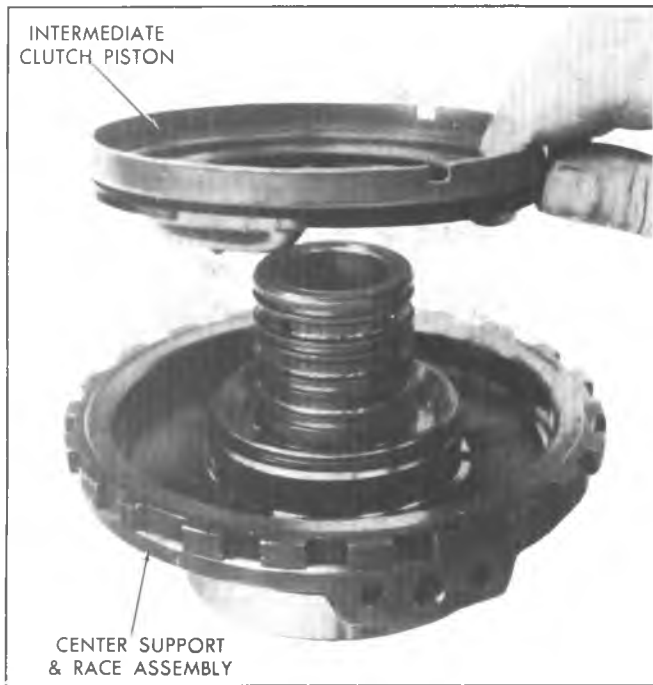
Fig. 7A-117C--Removing Intermediate Clutch Piston
