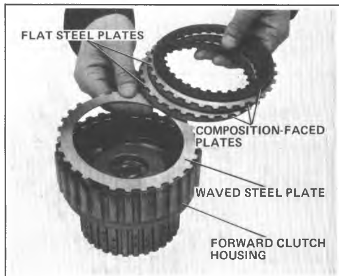
Figure 7A6-144 Installing Clutch Plates Into Forward Clutch Housing
