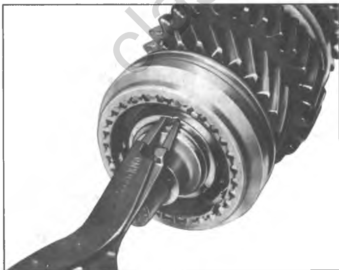
Fig. 7B-7A--Removing 2nd-3rd Clutch Hub Retaining Ring
