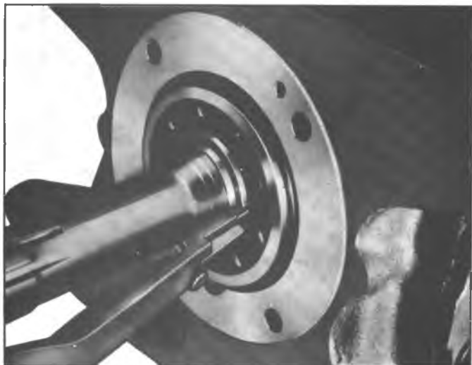
Fig. 7B-2A--Removing Clutch Gear Bearing Retaining Ring
