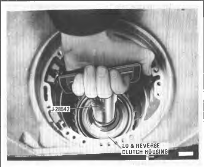
Figure 7A6-109 Installing Lo and Reverse Clutch
