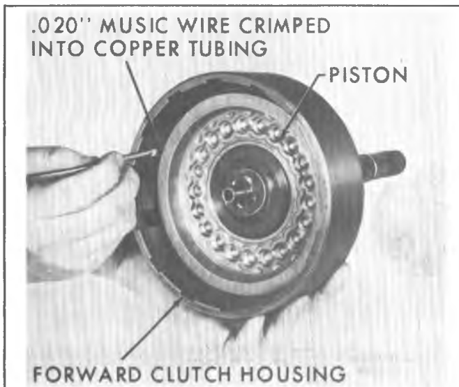
Figure 7A5-67 Installing Forward Clutch Piston
