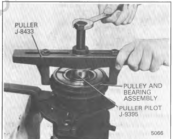
Fig. 1D-10 Removing A-6 Pulley and Bearing Asm.
