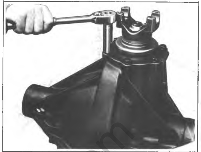
Fig. 7E--Removing Retainer Bolts
