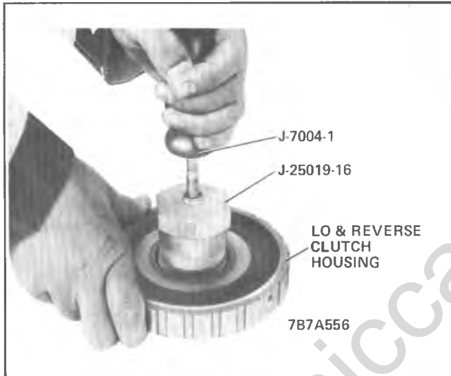
Figure 7A1-210 Removing Lo and Reverse Clutch Housing Bushing
