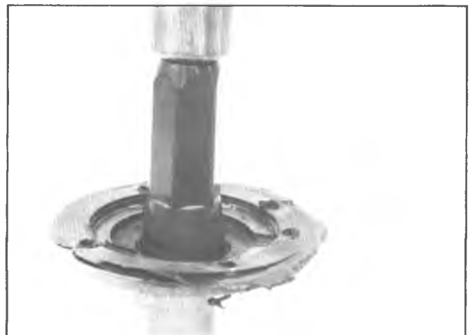
Fig. 16R--Installing Drive Gear Bearing Retainer Seal
