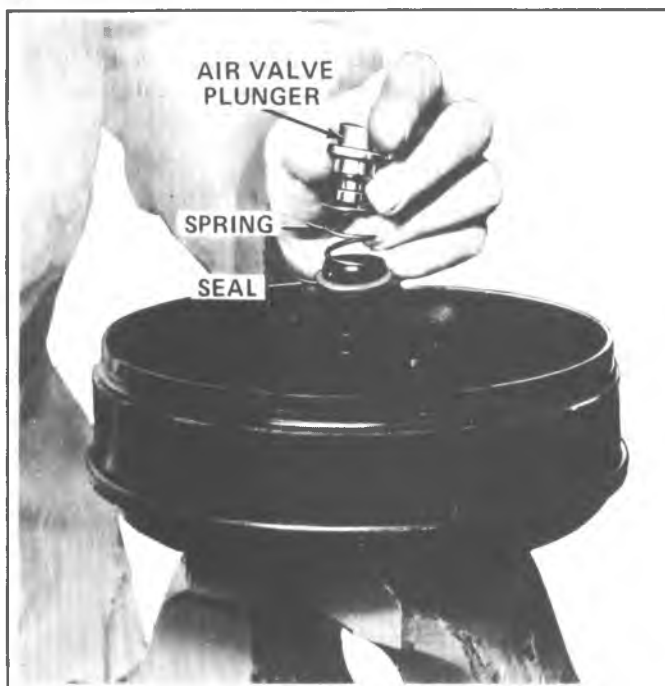
Fig. 5-10B--Installing Air Valve Plunger
