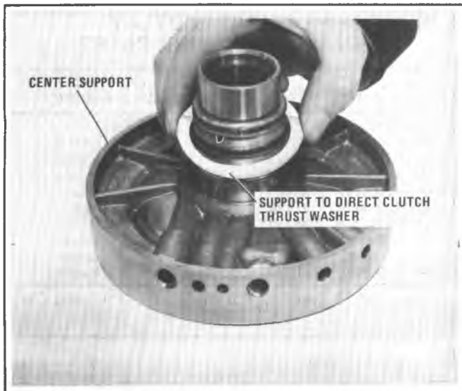
Figure 7A6-51 Removing Support to Direct Clutch Thrust Washer
