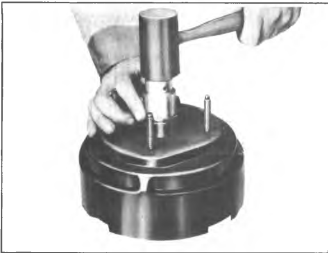
Fig. 5-6B--Removing Rear Seal
