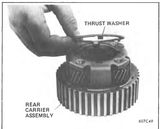
Figure 7A1-80 Installing Thrust Washer
