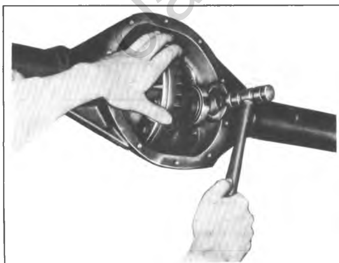
Fig. 9B--Installing Differential Shim
