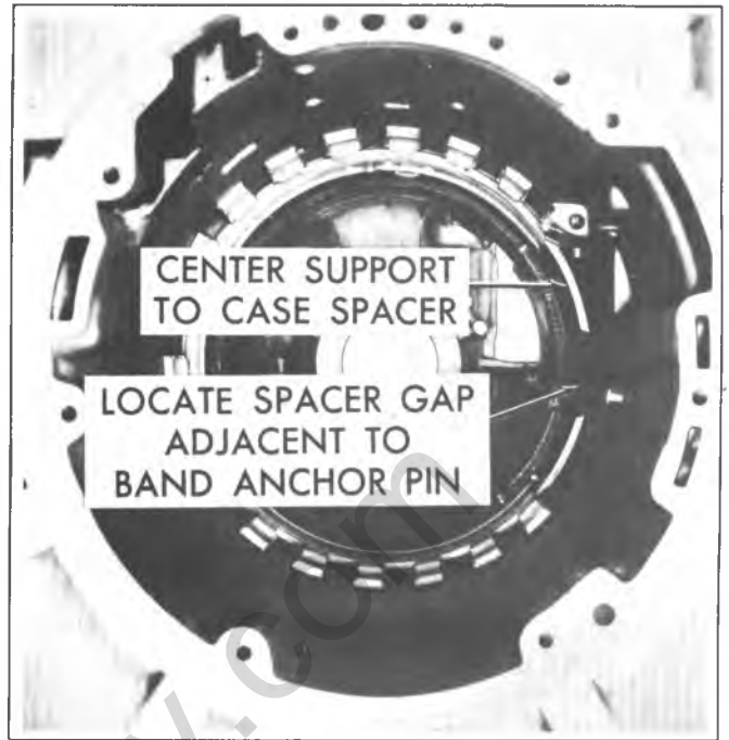
Fig. 7A-157C--Installing Center Support to Case Spacer
