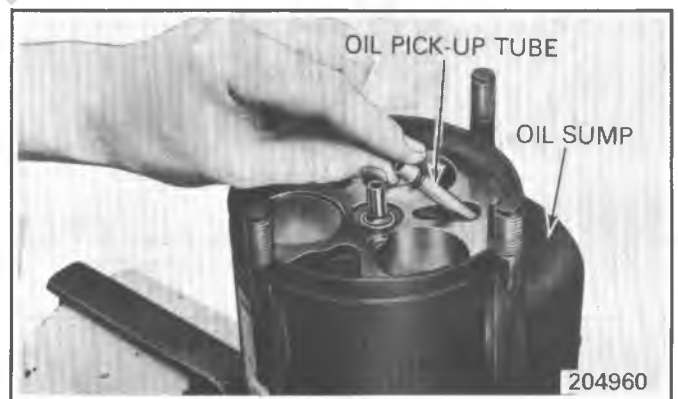
Fig. 1D-64 Installing A-6 Oil Pick-up Tube
