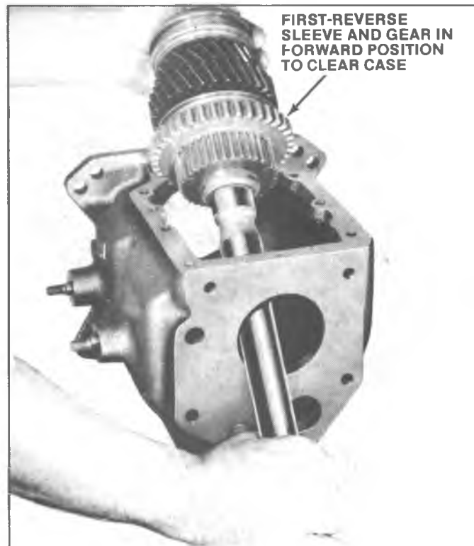
Fig. 7B-10B-Removing Output Shaft Assembly
