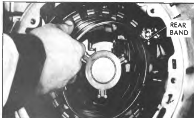
Fig. 7A-156C--Installing Rear Band
