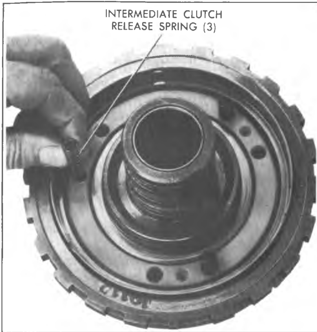
Fig. 7A-123C--Installing Intermediate Clutch Release Springs
