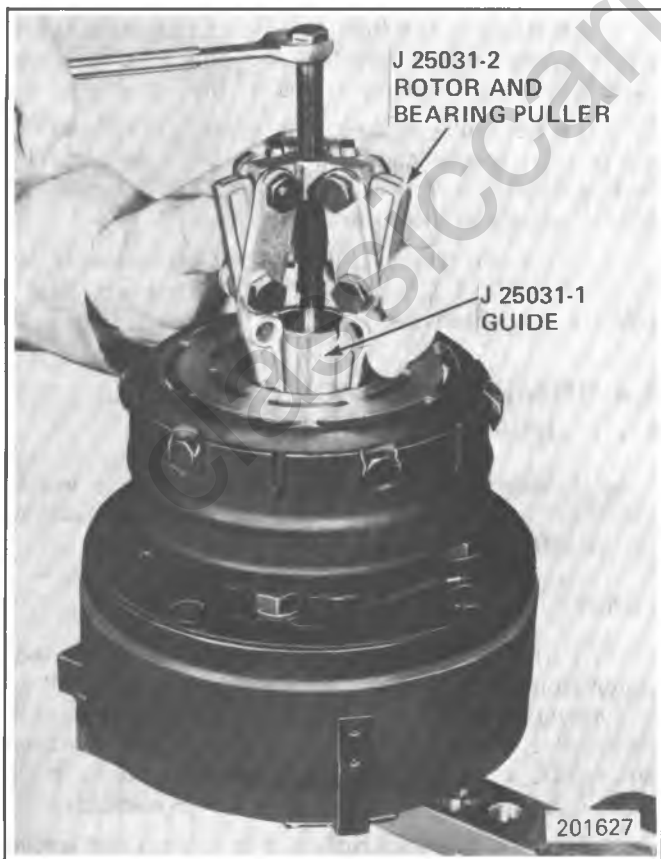
Fig. 1D-78 Removing R-4 Clutch Rotor Asm.
