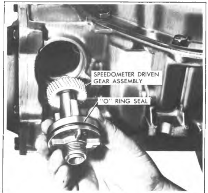
Fig. 7A-188C--Installing Speedometer Driven Gear and Sleeve
