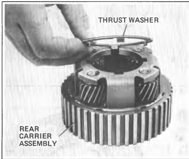
Figure 7A6-97 Installing Thrust Washer
