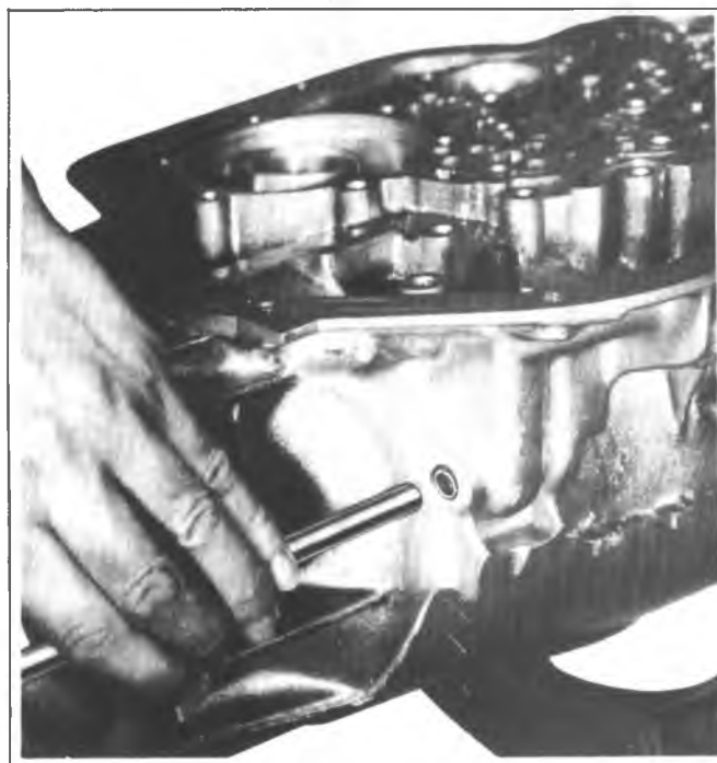
Fig. 7A-154C--Installing Parking Pawl Shaft Cup Plug
