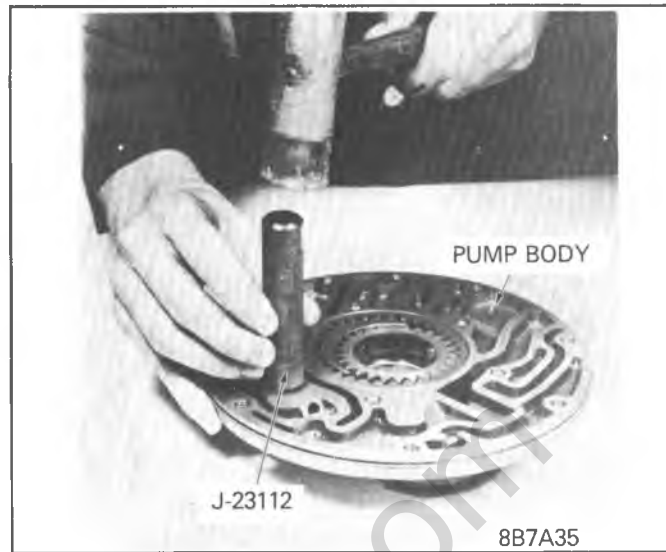
Figure 7A3-74 Installing Cooler By-Pass
