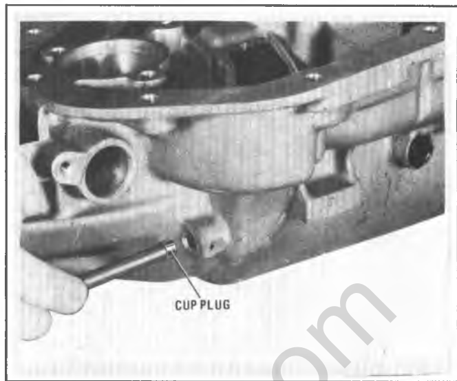
Figure 7A6-85 Installing Parking Pawl Cup Plug
