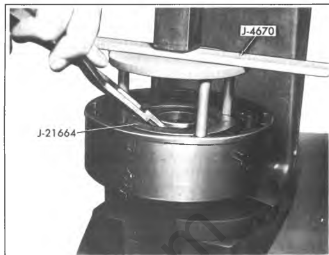
Fig. 7A-94C--Removing or Installing Direct Clutch Snap Ring
