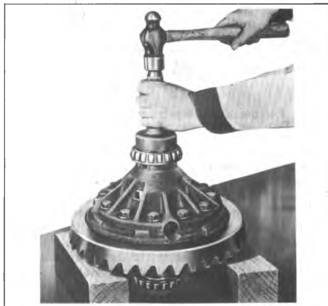
Fig. 5E—Differential Bearing Installation
