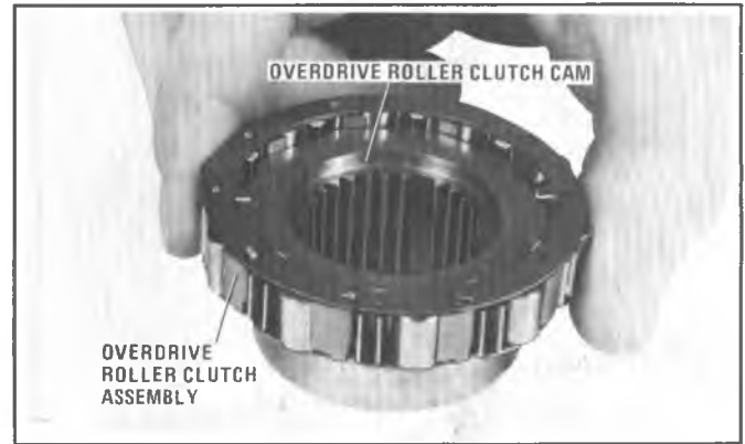
Figure 7A6-185 Installing Overrun Roller Clutch Cam
