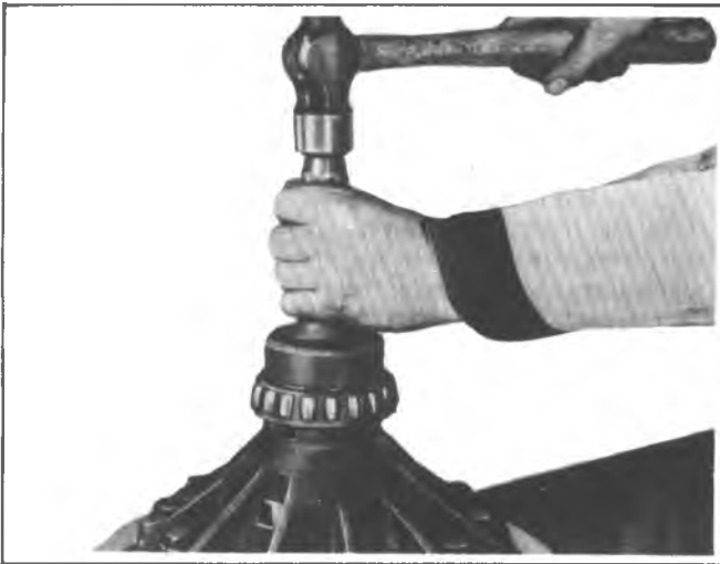
Fig. 8G--Differential Bearing Installation
