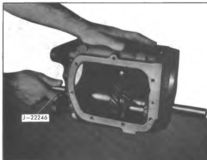
Fig. 7B-5A--Removing Counter Gear Shaft
