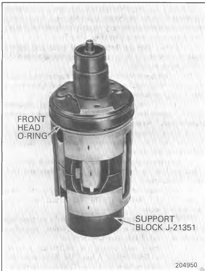
Fig. 1D-62 A-6 Front Head O-Ring Installed
