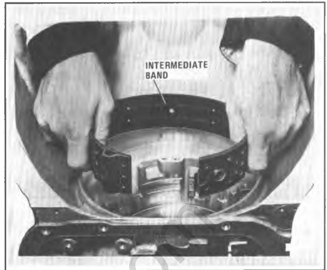
Figure 7A6-53 Removing Intermediate Band Assembly
