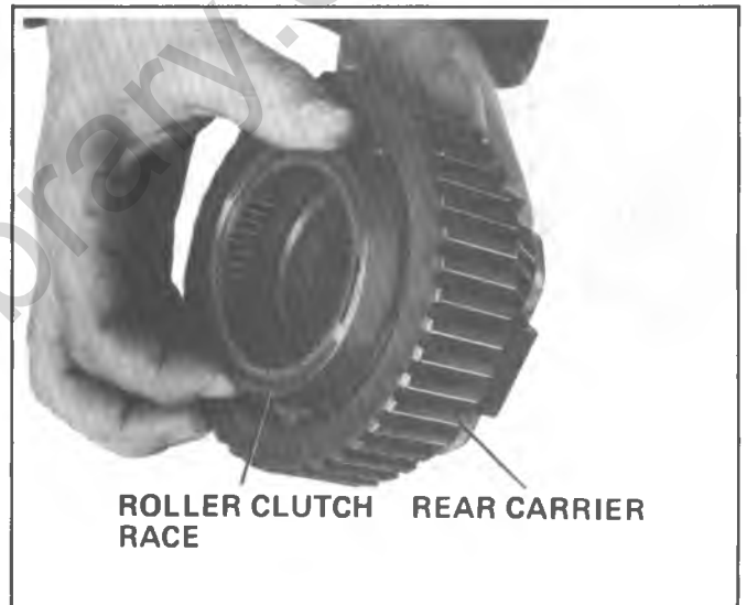
Figure 7A1-79 Installing Roller Clutch Race
