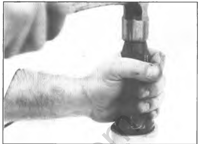
Fig. 15R--Installing Rear Extension Seal
