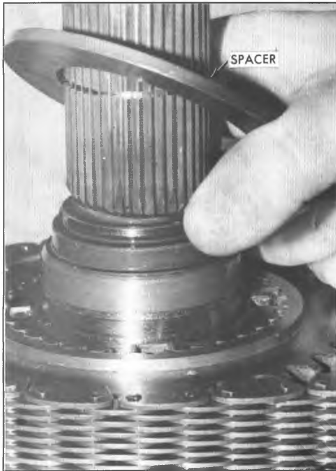
Fig. 7E-7-Drive Sprocket Thrust Washer Removal&Installation
