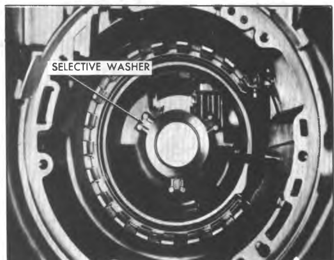
Fig. 7A-43C--Removing Selective Washer
