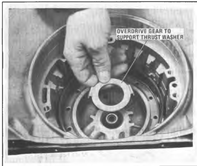
Figure 7A6-41 Removing Overdrive Internal Gear to Support Thrust Washer
