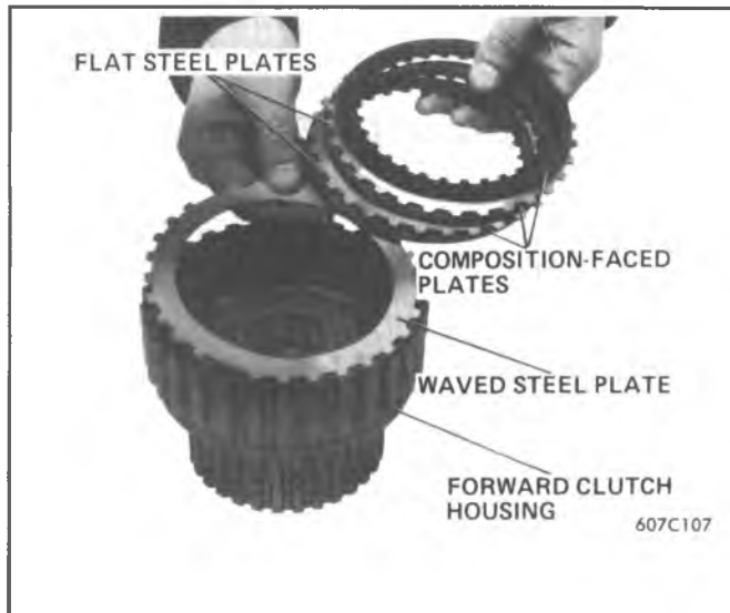
Figure 7A1-127 Installing Clutch Plates Into Forward Clutch Housing
