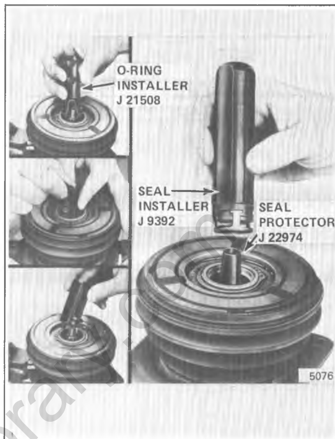
Fig. 1D-20 Replacing A-6 Seal and O-Ring
