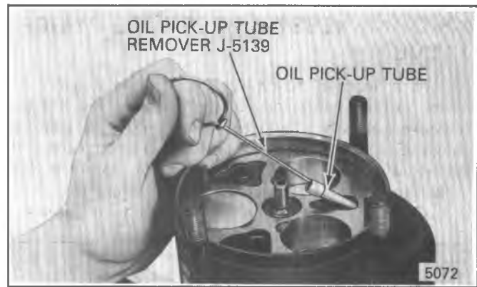
Fig. 1D-28 Removing A-6 Oil Pick-Up Tube
