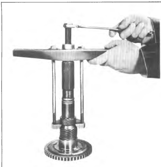
Fig. 7A-55C--Removing Steel Speedometer Drive Gear
