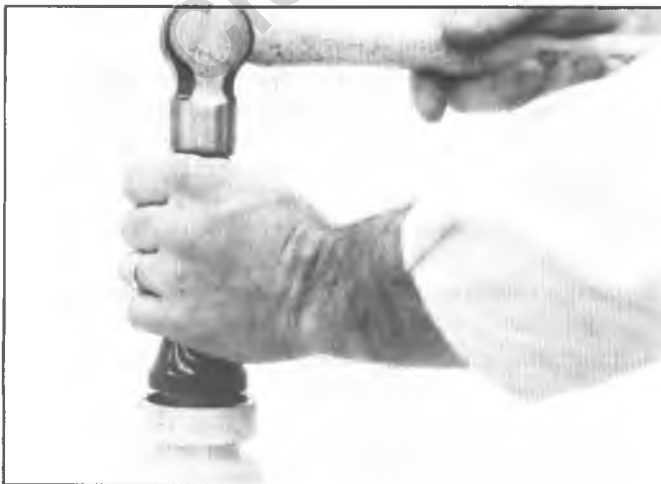
Fig. 14R--Installing Rear Extension Bushing
