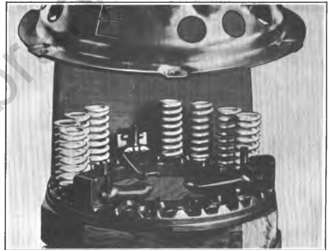
Fig. 7C-10E-Assembling Cover and Pressure Plate
