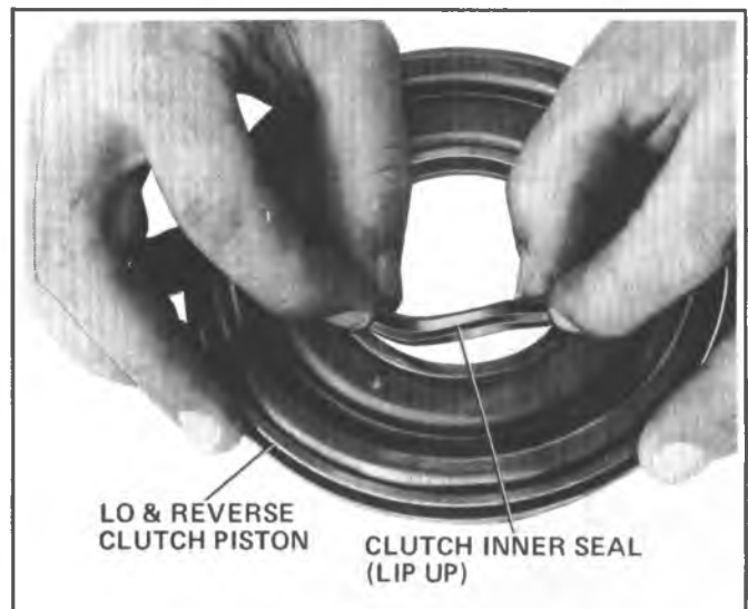
Figure 7A6-105 Removing Lo and Reverse Clutch Inner Seal
