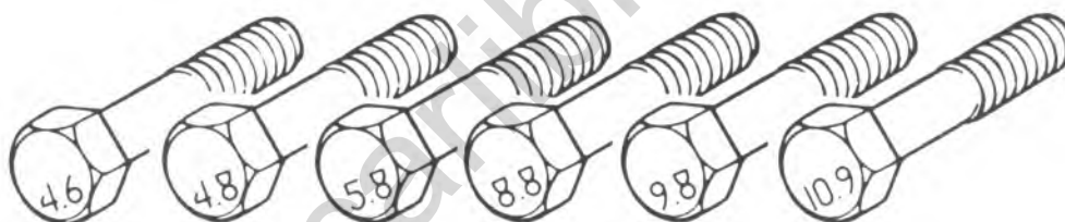
Metric Bolts - Identification class numbers correspond to bolt strength - Increasing numbers represent increasing strength.
