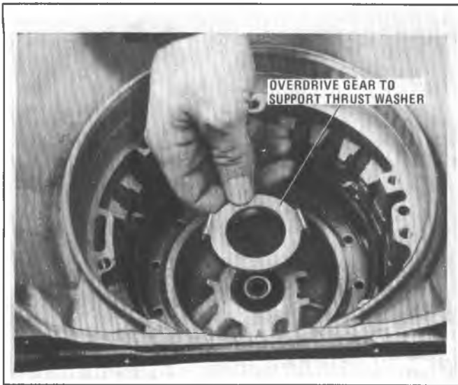
Figure 7A6-168 Installing Overdrive Internal Gear to Center Support Thrust Washer
