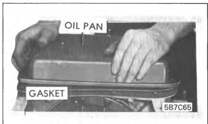
Figure 7A3-158 Install Oil Pan
