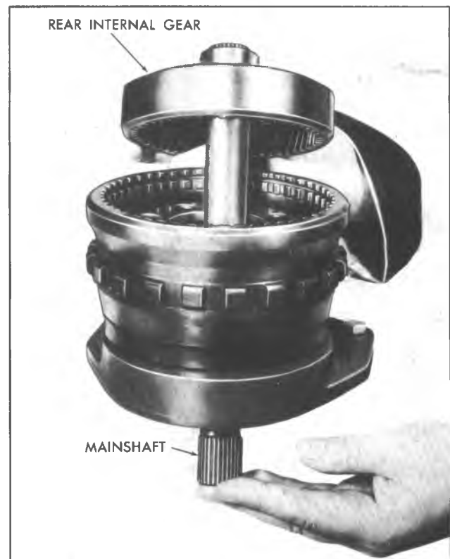
Fig. 7A-51C--Removing Rear Internal Gear and Mainshaft
