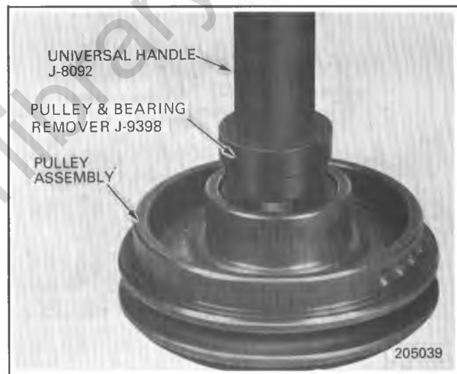
Fig. 1D-13 Removing Bearing From A-6 Pulley Asm.
