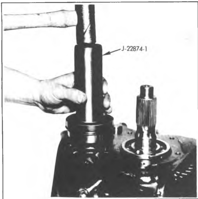
Fig. 7B-25L—Installing Countergear Rear Bearing
