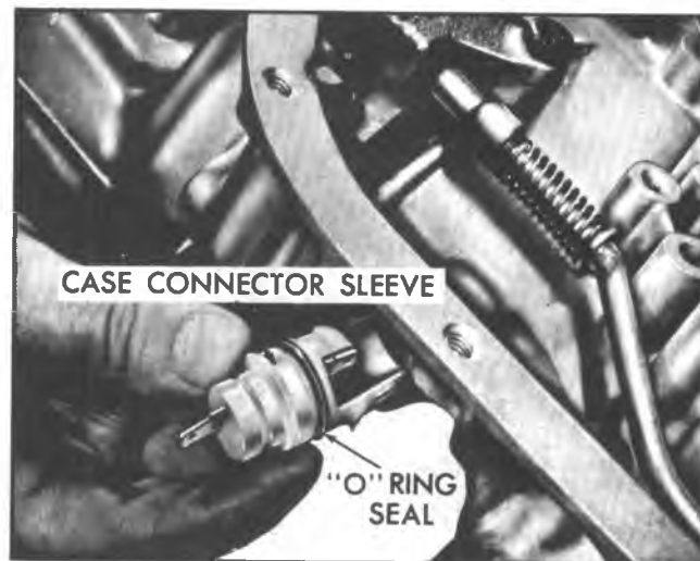
Fig. 7A-178C--Installing Electrical Connector and "O" Ring Seal
