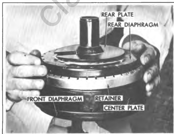
Fig. 5-11B--Installing Rear Diaphragm Retainer
