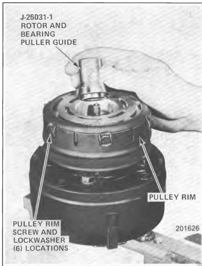
Fig. 1D-77 Installing R-4 Rotor & Bearing Puller Guide
