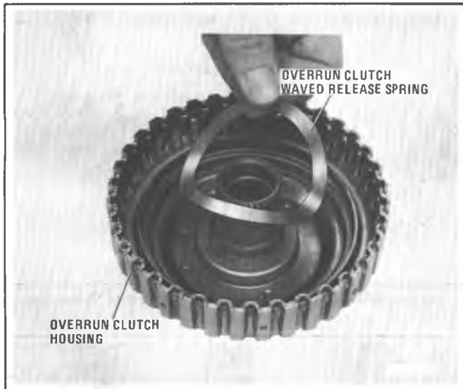
Figure 7A6-183 Installing Overrun Clutch Waved Release Spring
