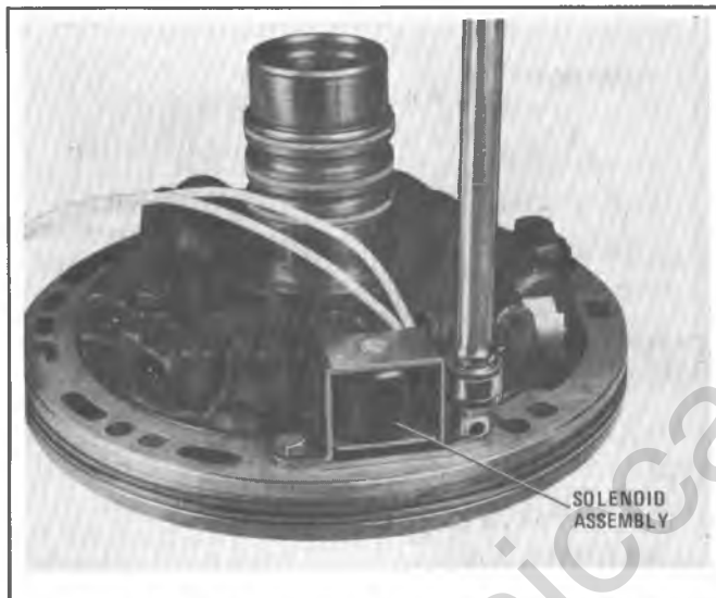
Figure 7A1-137 Removing Solenoid Attaching Bolts
