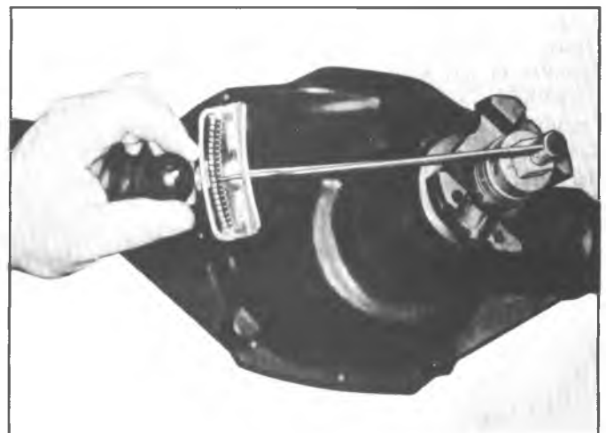
Fig. 26B--Measuring Rotating Torque
