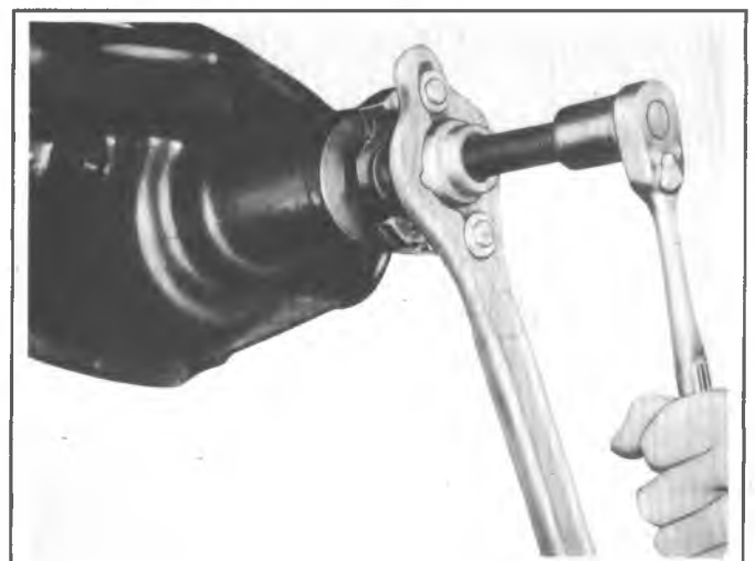
Fig. 15B--Drive Pinion Flange Removal
