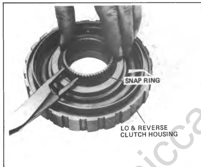
Figure 7A1-91 Installing Lo and Reverse Clutch Retaining Snap Ring
