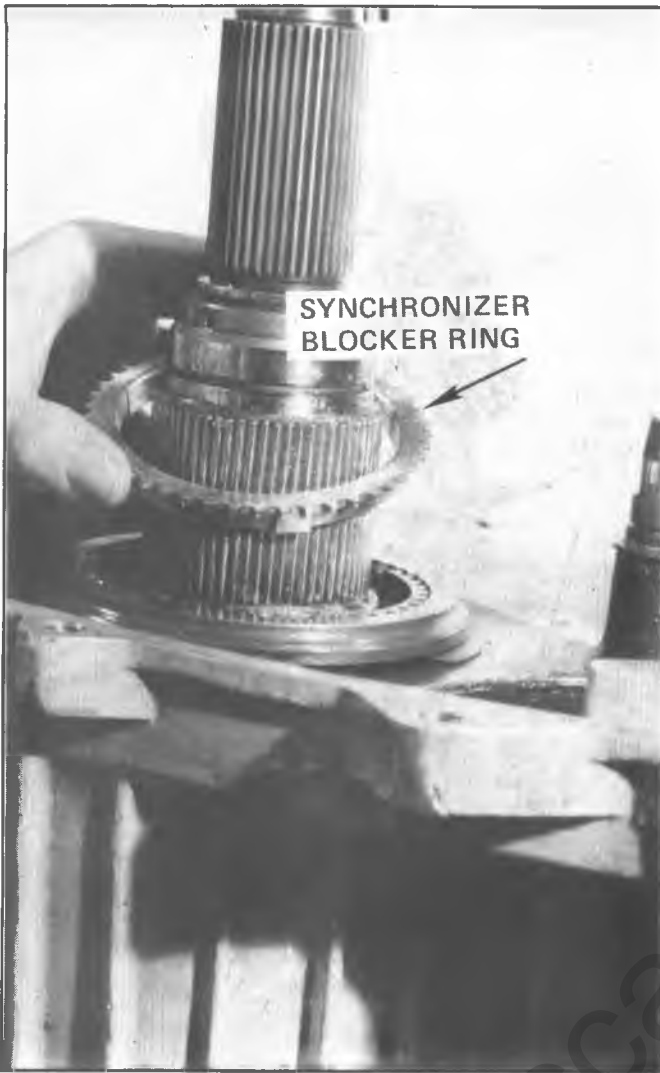
Fig. 7E-10-Synchronizer Blocker Ring Removal & Installation
