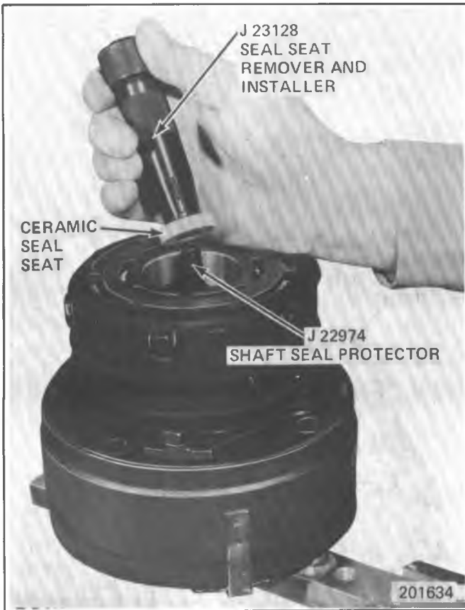
Fig. 1D-91 Removing & Installing R-4 Seal Seat (Off Car)
