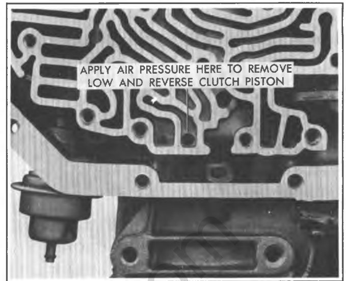
Figure 7A5-38 Removing Low & Reverse Piston
