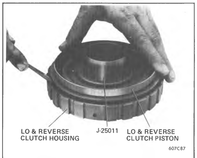
Figure 7A1-89 Installing Lo and Reverse Clutch Piston
