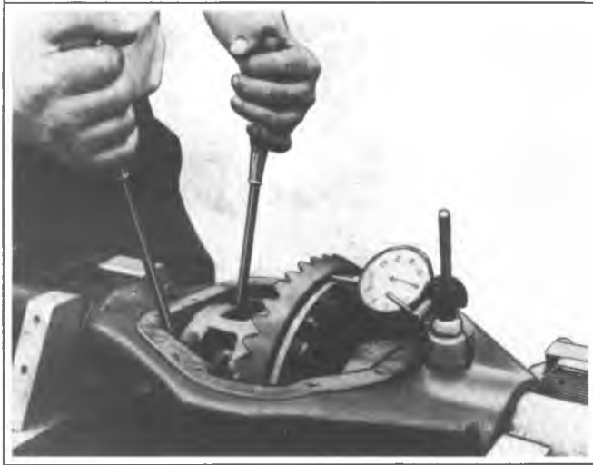
Fig. 8F -Screwdrivers Against Case
