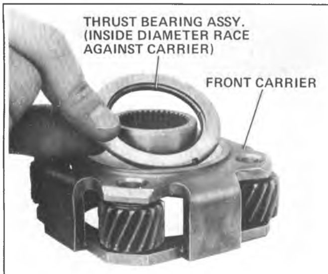
Figure 7A6-118 Installing Thrust Bearing Assembly Onto Front Carrier
