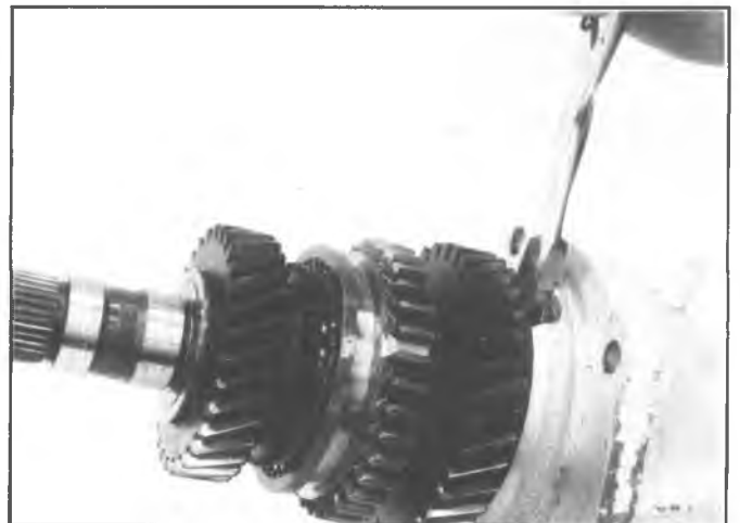
Fig. 9R--Remove or Install Mainshaft Bearing Snap Ring
