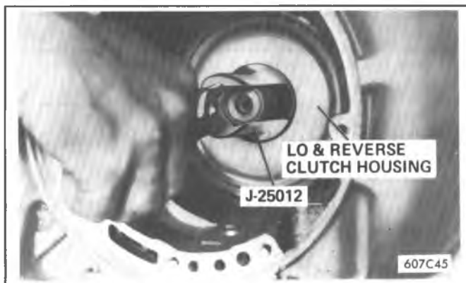
Figure 7A1-45 Removing Low and Reverse Clutch Housing
