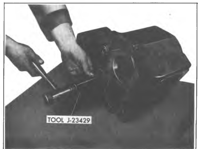
Fig. 7E-8R--Removing Idler Gear Shaft
