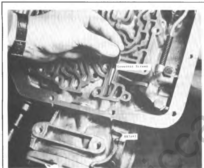
Figure 7A3-150 Installing Governor Feed Screen
