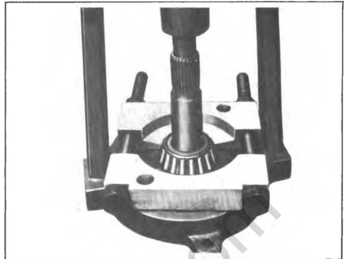
Fig. 17B--Removing Drive Pinion Rear Bearing and J-0270-14 for the 8-7/8" ring gear or J-22306 for the 9 1/2" ring gear as shown in figure 18B.
