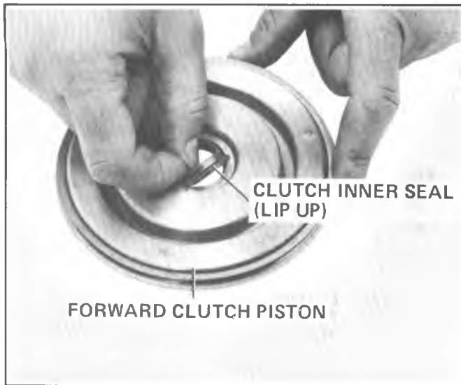
Figure 7A6-141 Removing or Installing Inner Piston Seal
