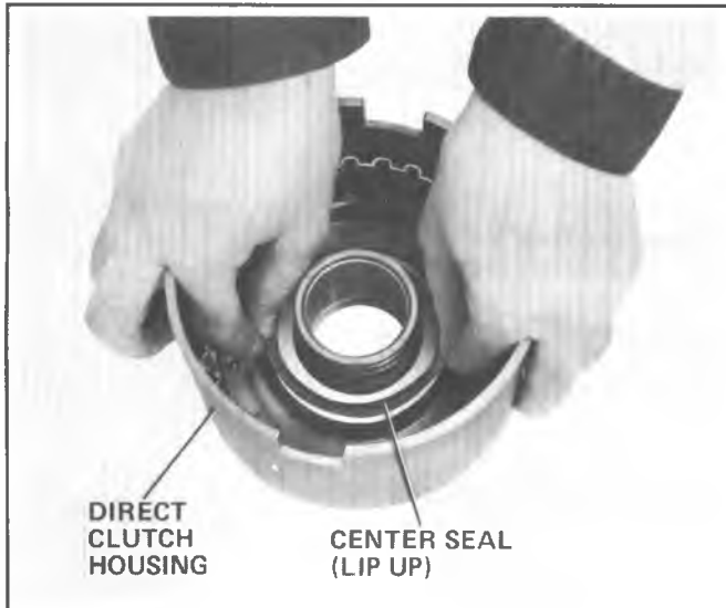
Figure 7A6-130 Removing or Installing Center Seal on Direct Clutch Housing
