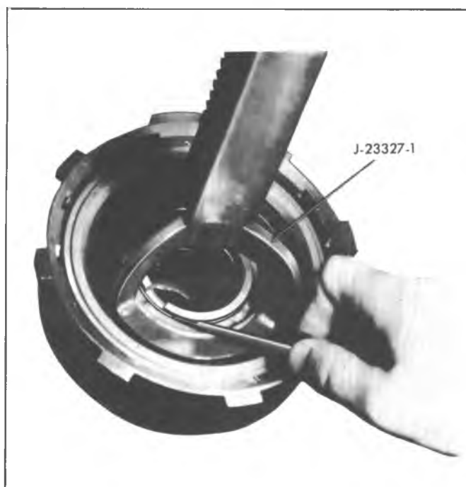
Fig. 7A-76B--Removing Direct Clutch Outer and Inner Seals
