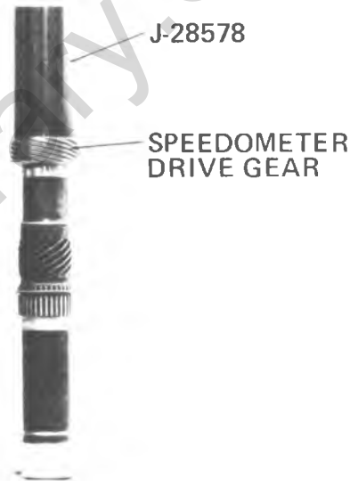
Figure 7A1-74 Installing Speedo Gear (Steel)
