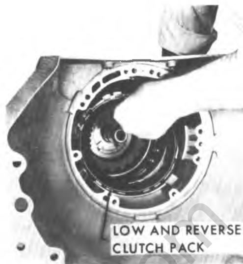
Figure 7A5-34 Low & Reverse Clutch Plate Removal
