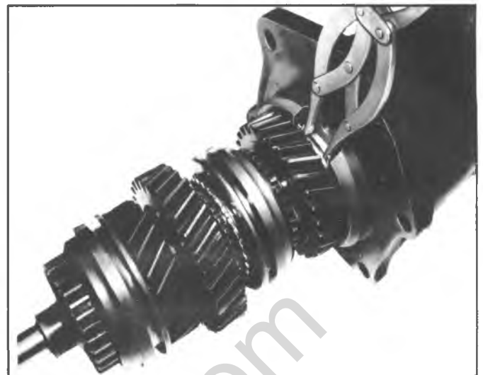
Fig. 7B-4A--Removing Rear Extension From Main Shaft
