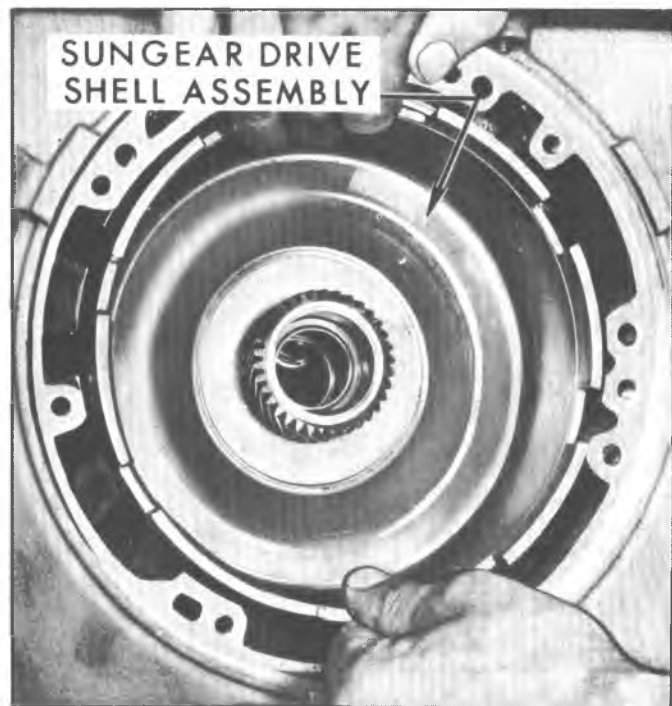
Fig. 7A-41B--Removing Sun Gear Drive Shell
