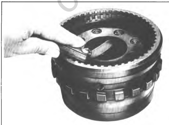
Fig. 7A-129C--Checking Output Carrier Pinion End Play
