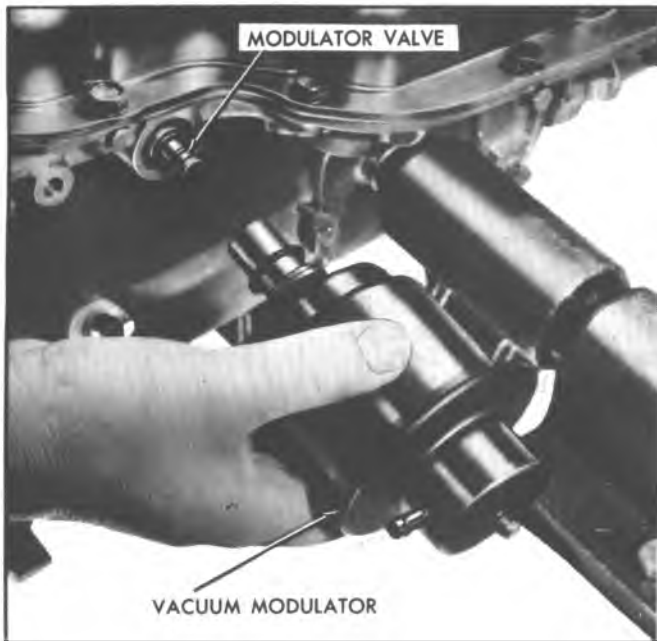
Fig. 7A-186C--Installing Vacuum Modulator and Valve
