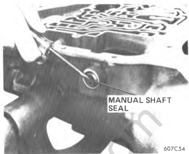
Figure 7A1-57 Removing Manual Shaft Seal From Case
