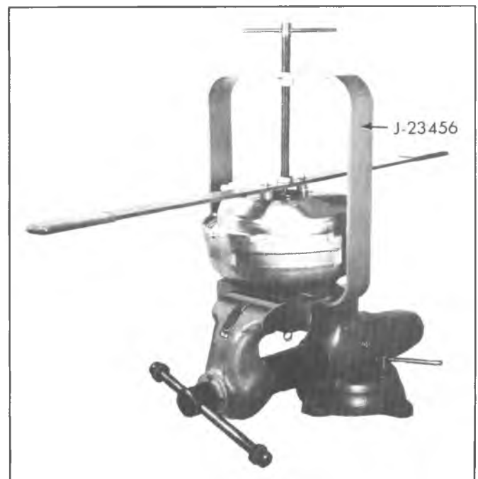
Fig. 5-1A—Unlocking Front and Rear Housings
