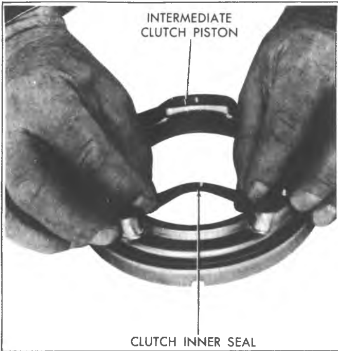
Fig. 7A-119C--Installing Intermediate Clutch Inner Seal
