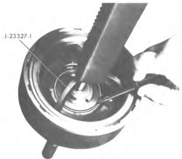
Figure 7A5-64 Compressing Forward Clutch Spring Retaining Seat
