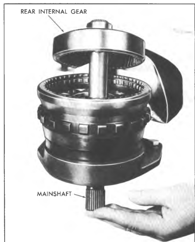
Fig. 7A-51C--Removing Rear Internal Gear and Mainshaft
