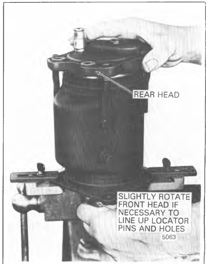
Figure 1D-72 Installing A-6 Rear Head
