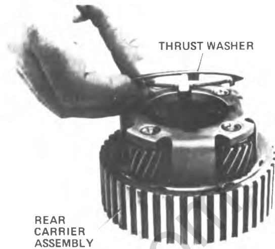
Figure 7A1-83 Installing Thrust Washer
