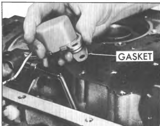
Fig. 7A-18C--Removing Detent Solenoid and Gasket
