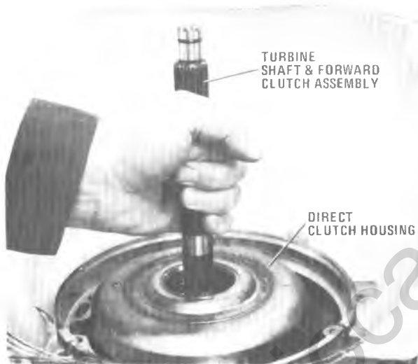
Figure 7A1-35 Removing Forward and Direct Clutch Assemblies
