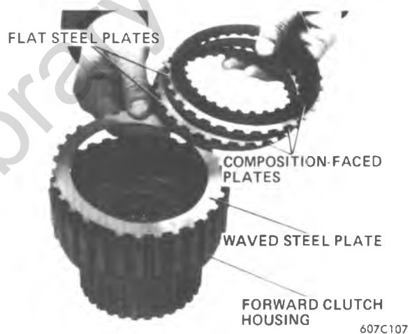
Figure 7A1-131 Installing Clutch Plates Into Forward Clutch Housing
