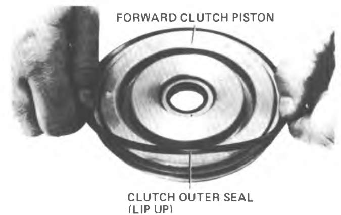
Figure 7A1-126 Removing or Installing Outer Piston Seal
