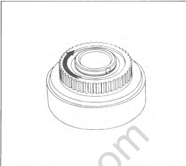
Fig. 7A-152C--Checking Roller Clutch Rotation
