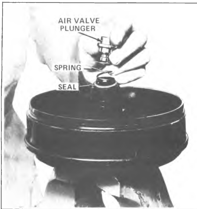
Fig. 5-10B—Installing Air Valve Plunger
