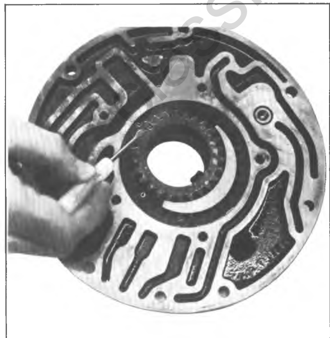
Fig. 7A-66B--Installing Pump Drive and Driven Gears
