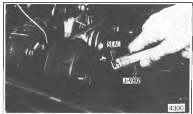
Figure 1D-94 Removing R-4 Seal (On Car)
