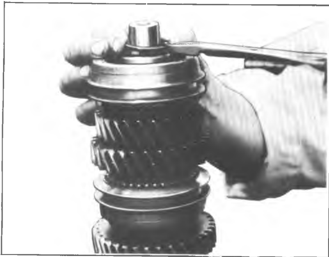
Fig. 7B-9K—Removing 3-4 Clutch Assembly Retainer
