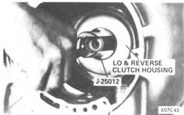
Figure 7A1-48 Removing Low and Reverse Clutch Housing
