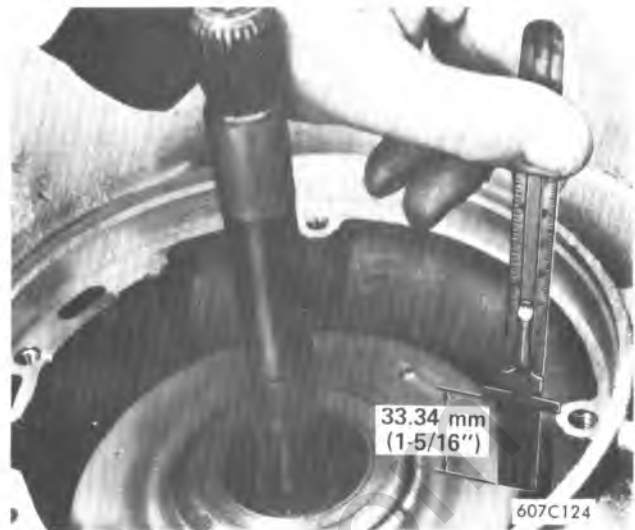
Figure 7A1-136 Direct and Forward Clutch Assemblies Properly Installed
