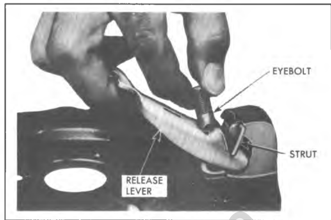
Fig. 7C-5E-Removing or Installing Lever
