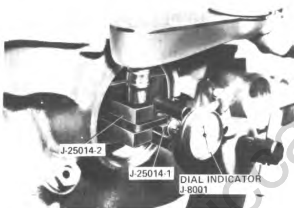
Figure 7A1-28 Checking for Proper Intermediate Band Apply Pin
