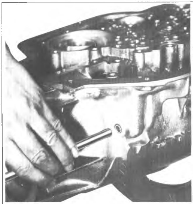
Fig. 7A-154C--Installing Parking Pawl Shaft Cup Plug
