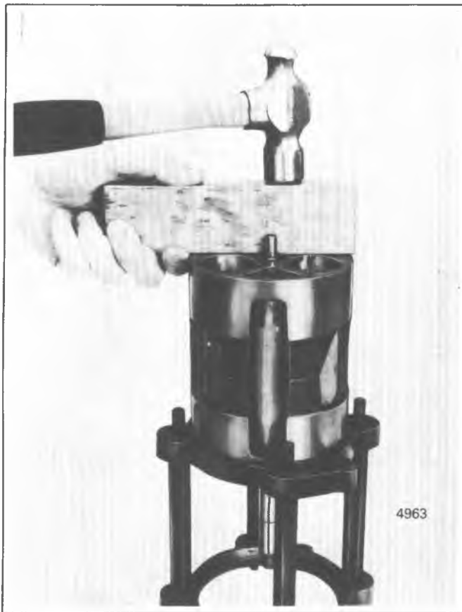
Figure 1D-44 Assembling A-6 Cylinder Halves
