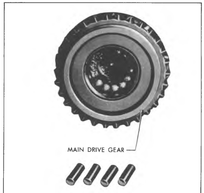
Fig. 7B-17A--Loading Pilot Bearings
