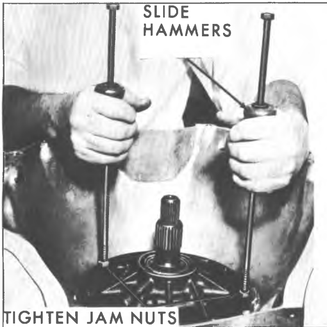
Fig. 7A-30B--Removing Pump from Case
