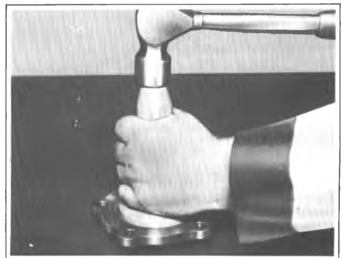
Fig. 4G--Pinion Oil Seal Installation
