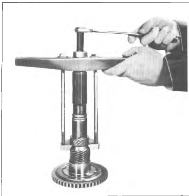
Fig. 7A-55C--Removing Steel Speedometer Drive Gear
