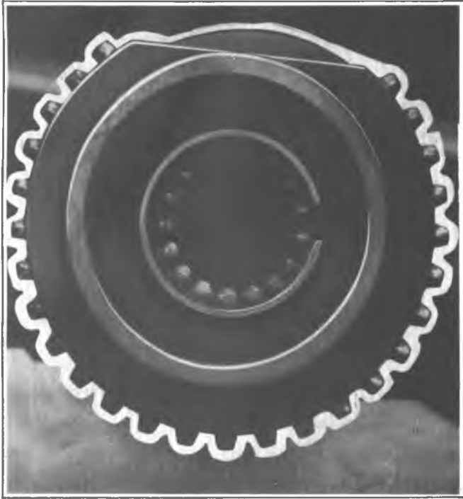
Fig. 7B-12L—Pilot Roller Bearing Installed
