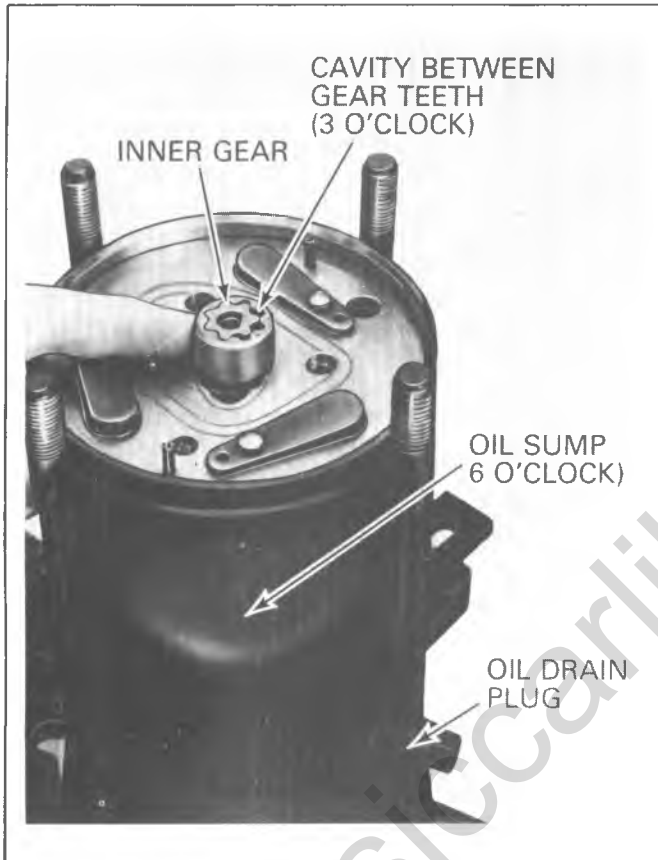
Figure 1D-70 Positioning A-6 Oil Pump Gears
