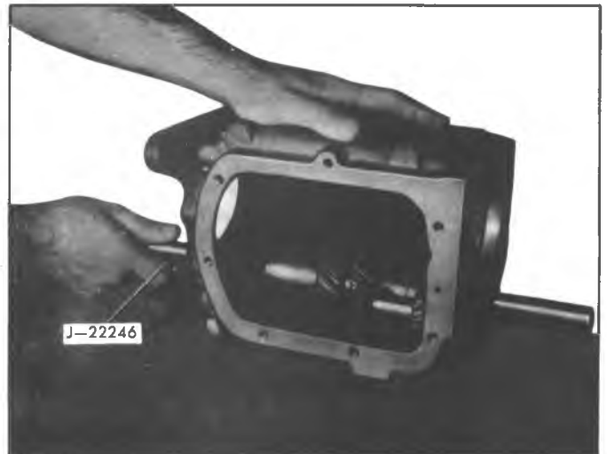
Fig. 7B-5A--Removing Counter Gear Shaft
