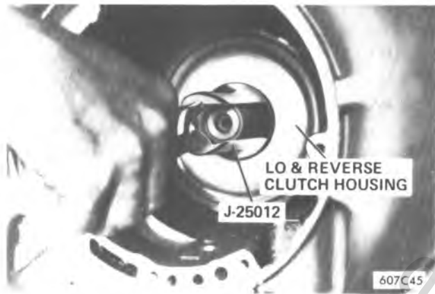
Figure 7A1-97 Installing Low and Reverse Clutch
