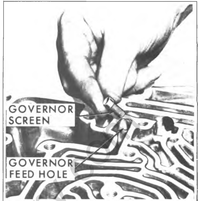
Fig. 7A-20B--Removing Governor Feed Screen
