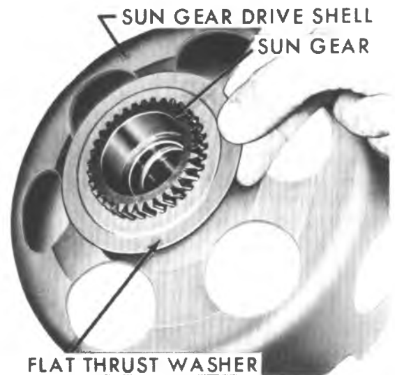
Figure 7A5-71 Removing Sun Gear to Drive Shell
