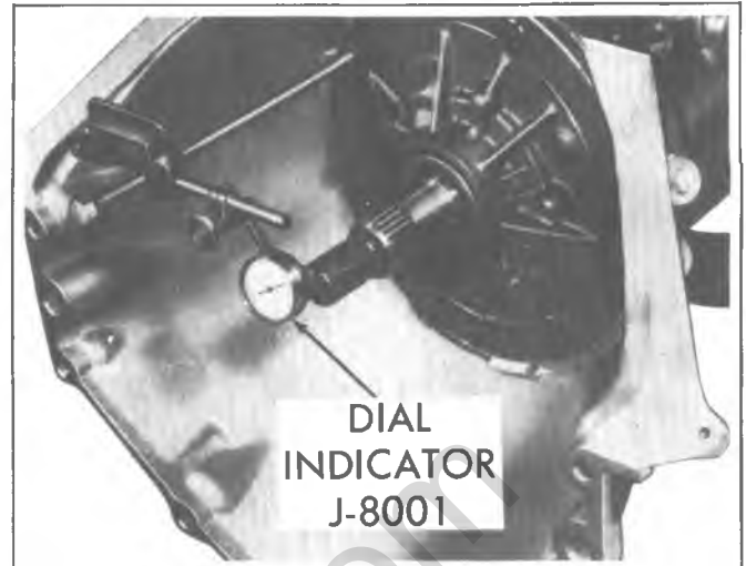
Fig. 7A-29C--Checking Front Unit End Play
