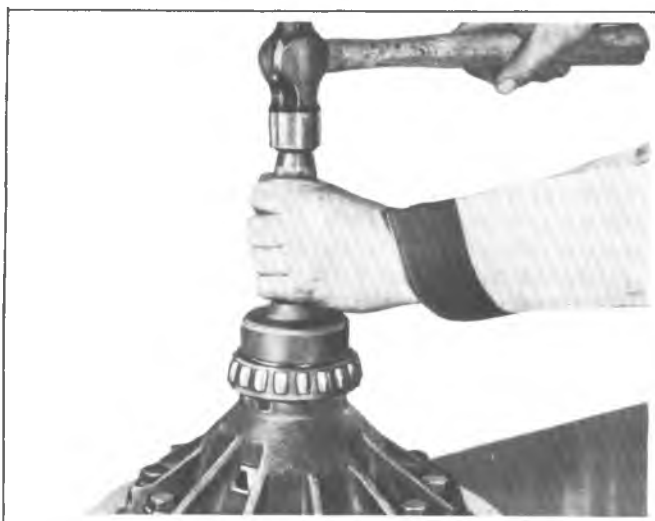
Fig. 8G--Differential Bearing Installation
