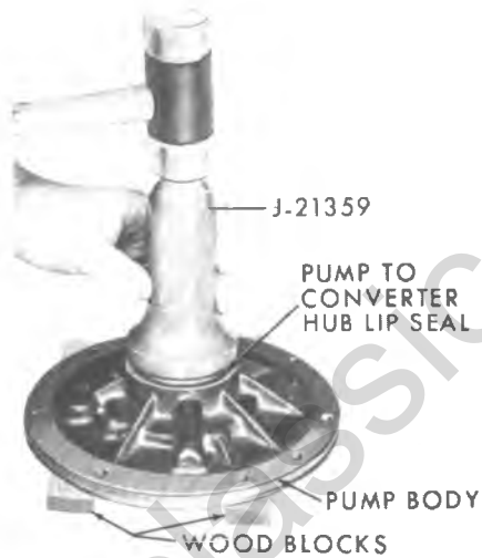
Figure 7A5-48 Installing Hub Lip Seal
