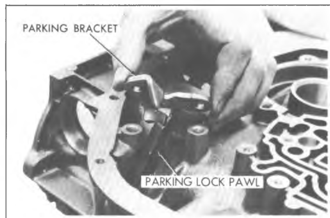
Fig. 7A-23C--Removing Parking Bracket
