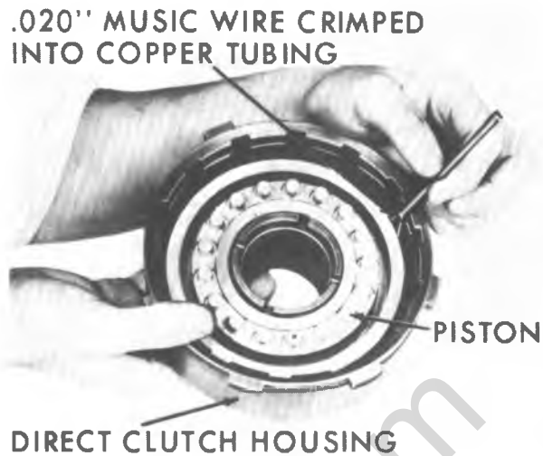
Figure 7A5-58 Installing Direct Clutch Piston
