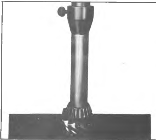
Fig. 22B—Installing Rear Bearing
