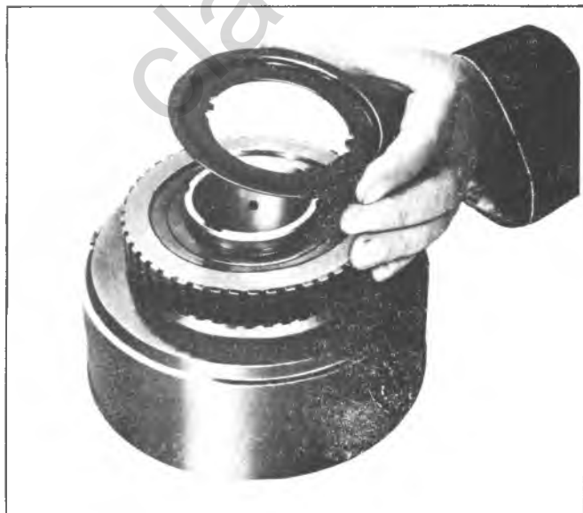
Fig. 7A-109C--Installing Intermediate Clutch Retainer
