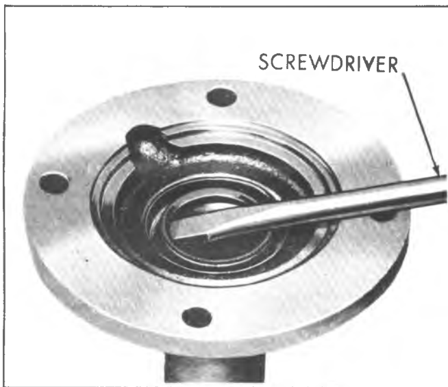
Fig. 7B-14J—Removing Bearing Retainer Oil Seal
