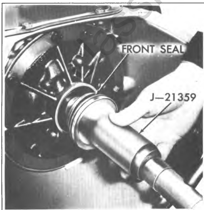
Fig. 7A-168C--Installing Pump Seal
