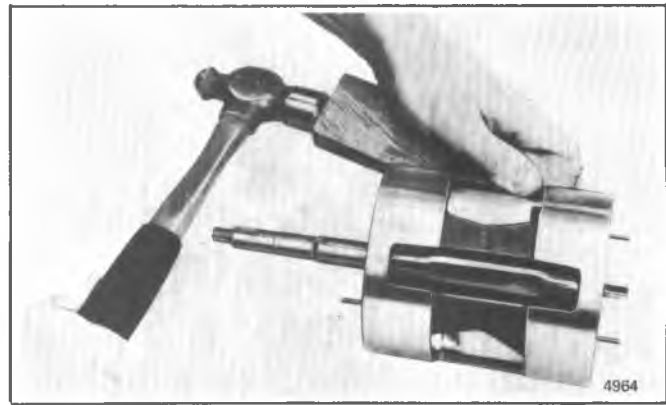
Figure 1D-36 Separating A-6 Cylinder Halves
