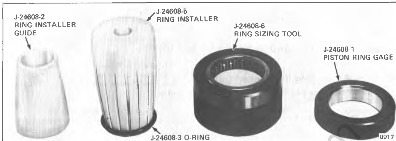
Figure 1D-50 A-6 Teflon Piston Ring Installing, Sizing and Gaging Tools
