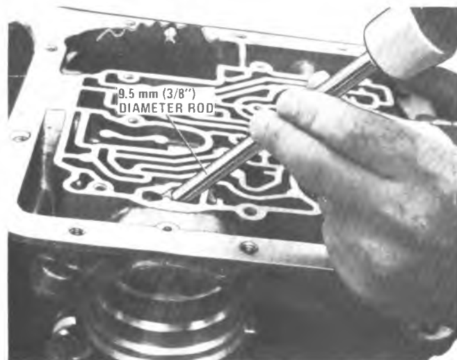
Figure 7A1-29C Installing 3rd Accumulator Check Valve Assy.
