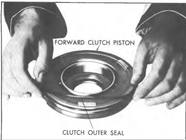
Fig. 7A-84C--Removing Forward Clutch Piston Outer Seal
