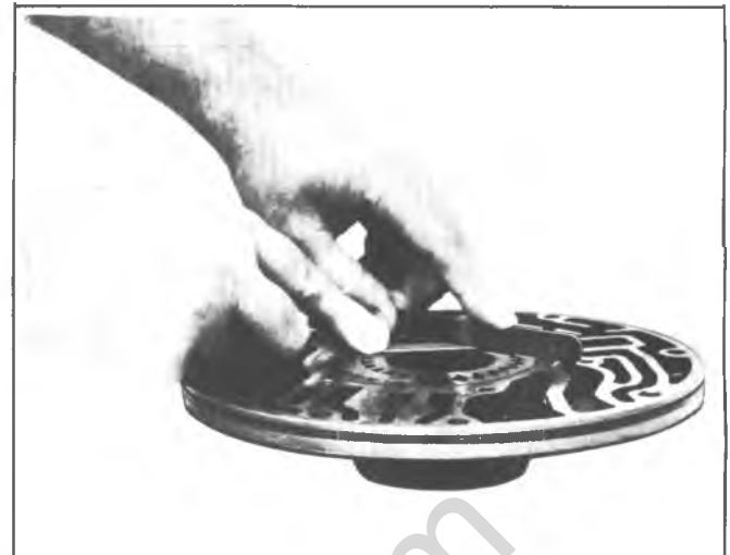
Fig. 7A-63B--Checking Pump Body to Gear Face Clearance
