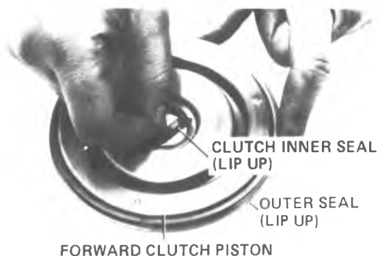
Figure 7A1-127 Removing or Installing Inner Piston Seal
