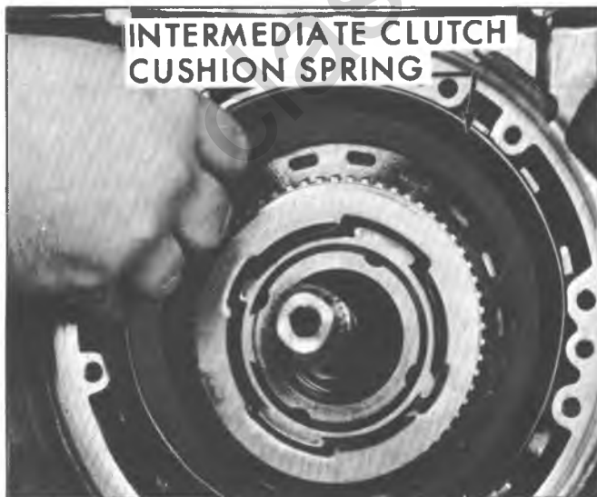
Fig. 7A-31B--Removing Intermediate Clutch Cushion Spring
