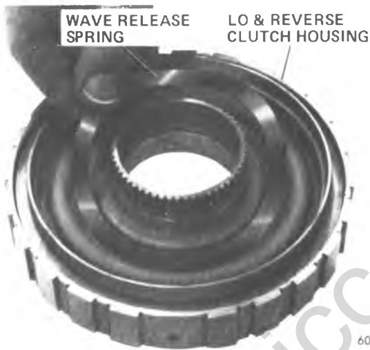
Figure 7A1-89 Removing Lo and Reverse Clutch Wave Release Spring.
