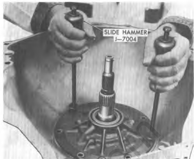
Figure 7A5-23 Pump Removal
