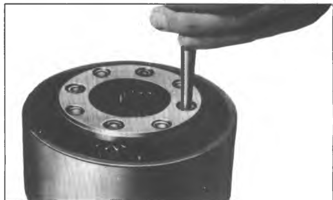
Fig. 7A-130C--Removing Planet Pinion Pin
