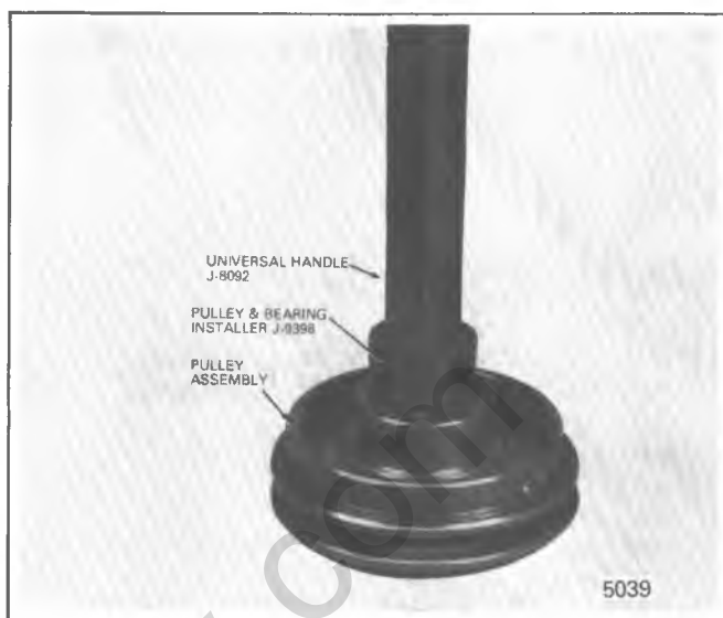
Figure 1D-16 Removing Bearing From A-6 Pulley Assembly
