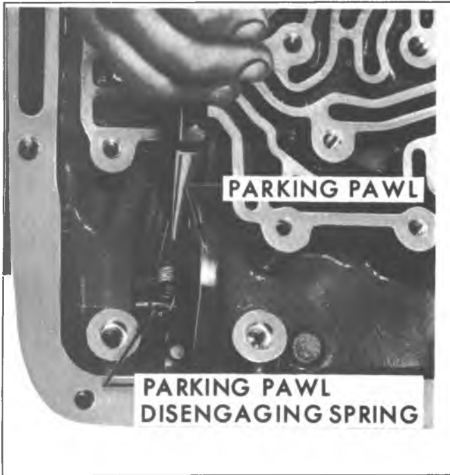
Fig. 7A-26B--Removing Parking Pawl Disengaging Spring
