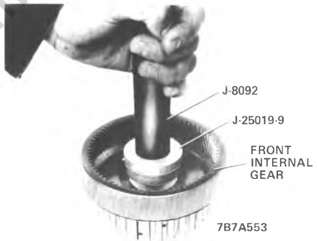
Figure 7A1-192 Installing Front Internal Gear Bushing
