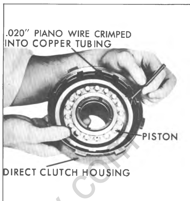
Fig. 7A-78B--Installing Direct Clutch Piston
