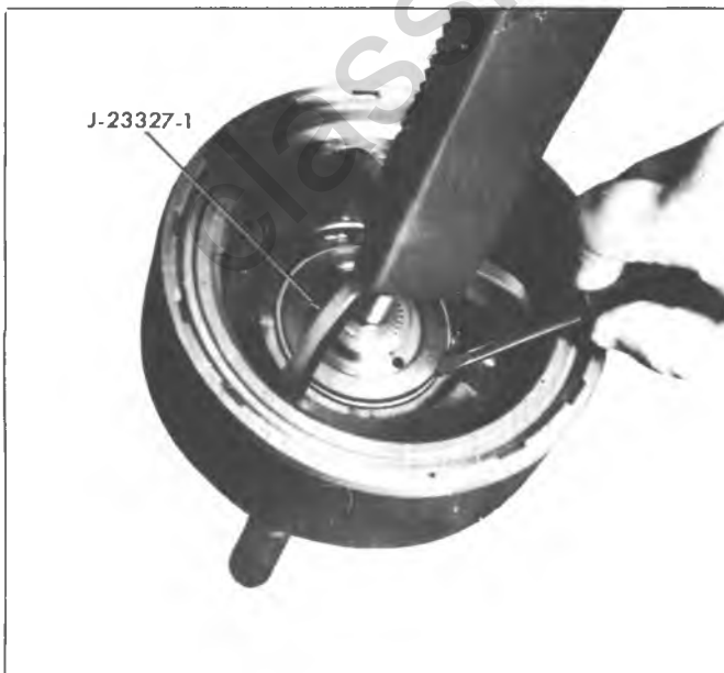
Fig. 7A-84B--Compressing Forward Clutch Piston Return Seat
