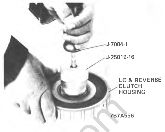
Figure 7A1-195 Removing Lo and Reverse Clutch Housing Bushing
