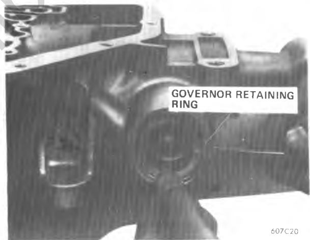
Figure 7A1-23 Removing Governor Cover Retaining Ring
