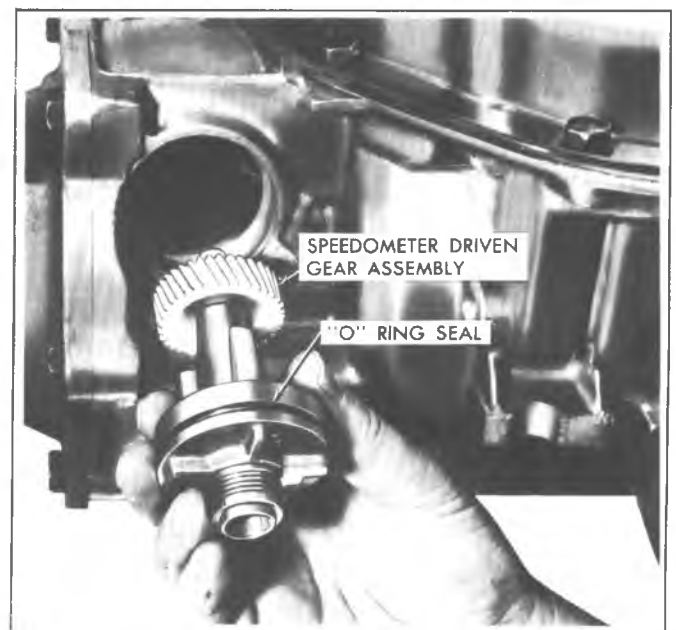
Fig. 7A-188C--Installing Speedometer Driven Gear and Sleeve
