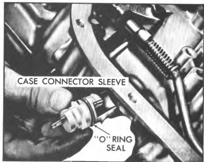
Fig. 7A-178C--Installing Electrical Connector and "O" Ring Seal
