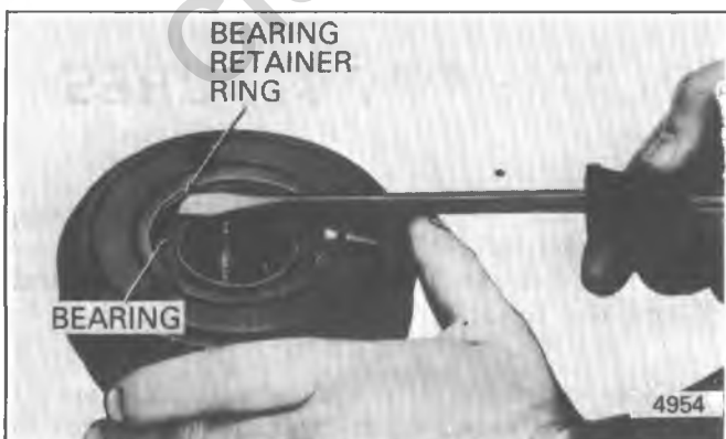
Figure 1D-15 Removing A-6 Pulley and Bearing Retainer Ring
