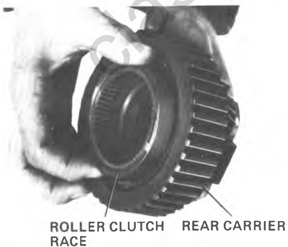
Figure 7A1-82 Installing Roller Clutch Race
