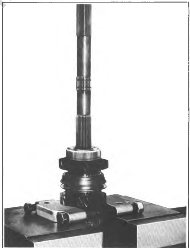
Fig. 7B-12K—Pressing Rear Bearing From Mainshaft
