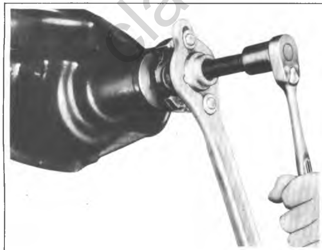
Fig. 13B--Drive Pinion Flange Removal
