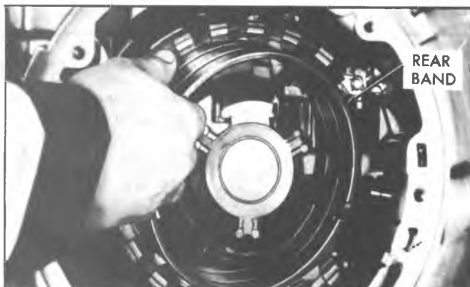
Fig. 7A-156C--Installing Rear Band
