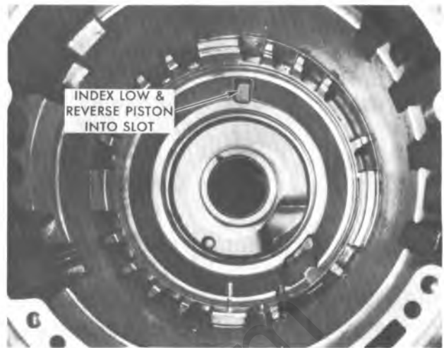
Figure 7A5-80 Low & Reverse Piston Indexing Slot
