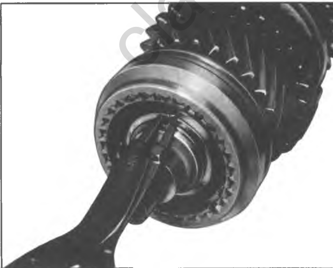
Fig. 7B-7A—Removing 2nd-3rd Clutch Hub Retaining Ring
