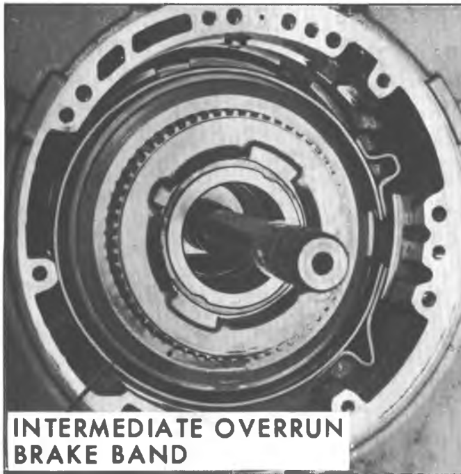
Fig. 7A-34B--Removing Intermediate Overrun Brake Band
