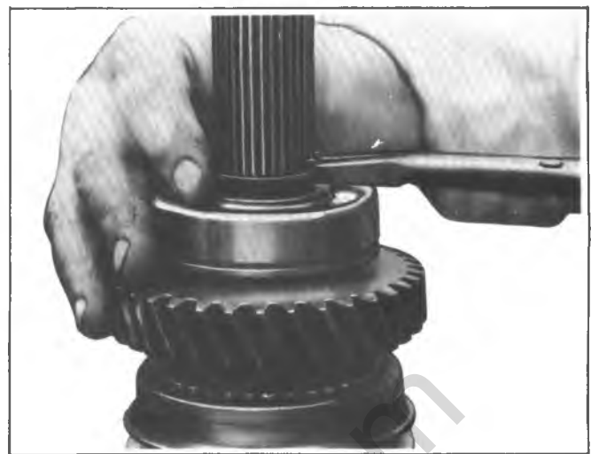
Fig. 7B-11K—Removing Rear Bearing Snap Ring
