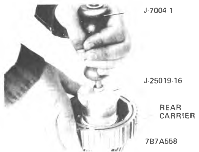
Figure 7A1-197 Removing Rear Carrier Bushing
