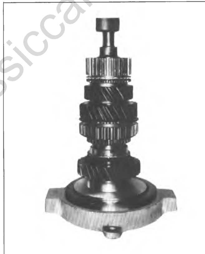
Fig. 7B-17J-Installing Rear Bearing
