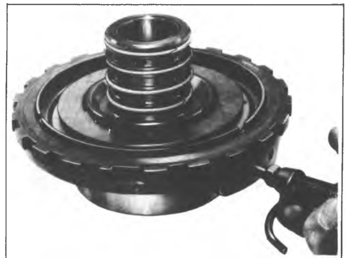
Fig. 7A-126C--Air Checking Intermediate Clutch Piston
