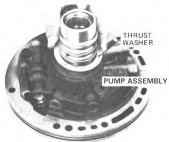
Figure 7A1-138 Removing Thrust Washer from Pump
