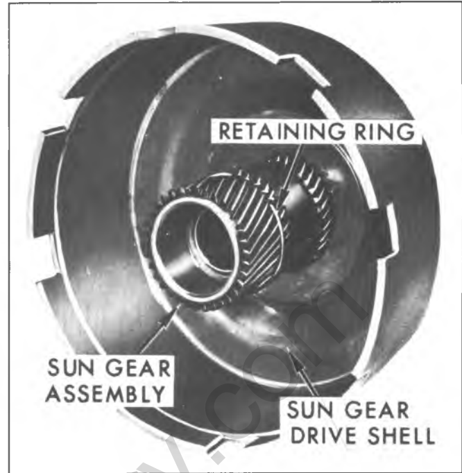
Fig. 7A-92B--Removing Sun Gear to Drive Shell Front Steel Thrust Washer
