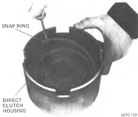
Figure 7A1-113 Removing Direct Clutch Snap Ring
