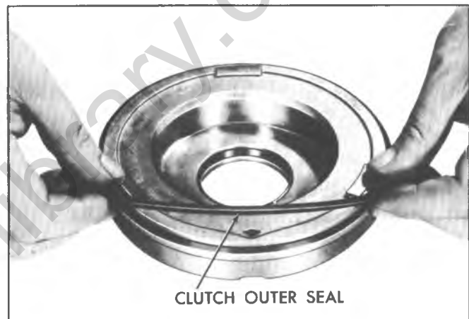
Fig. 7A-97C--Installing Direct Clutch Outer Seal
