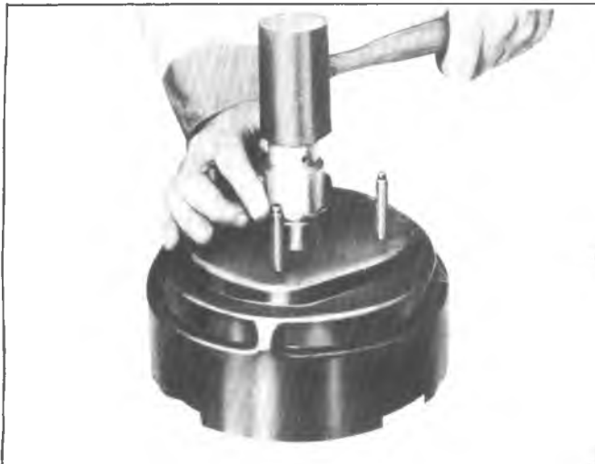
Fig. 5-6B--Removing Rear Seal
