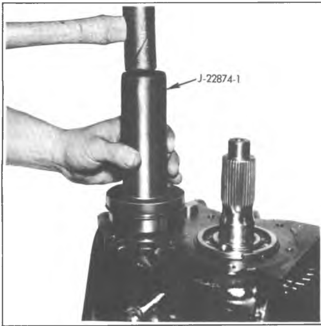
Fig. 7B-25L—Installing Countergear Rear Bearing
