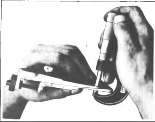
Fig. 8B--Measuring Gage Plate Thickness
