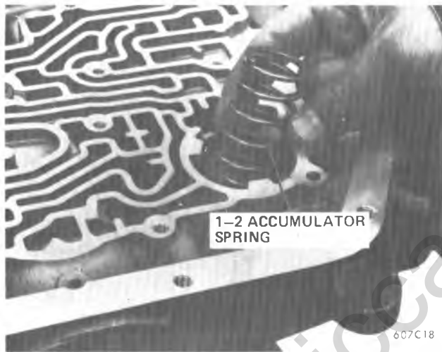
Figure 7A1-21 Removing 1-2 Accumulator Spring
