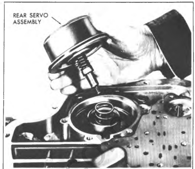
Fig. 7A-181C--Installing Rear Servo Assembly
