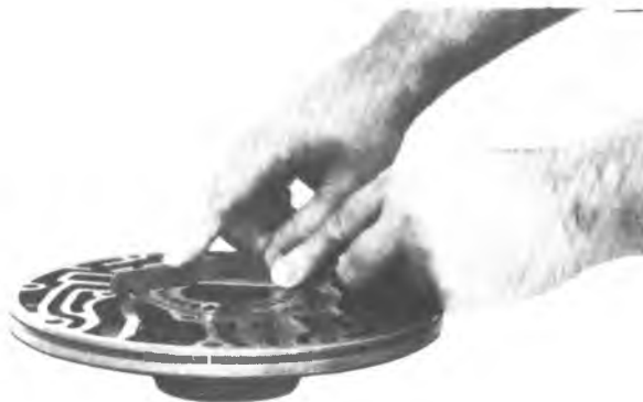
Figure 7A5-49 Checking Pump Body to Gear Face Clearance
