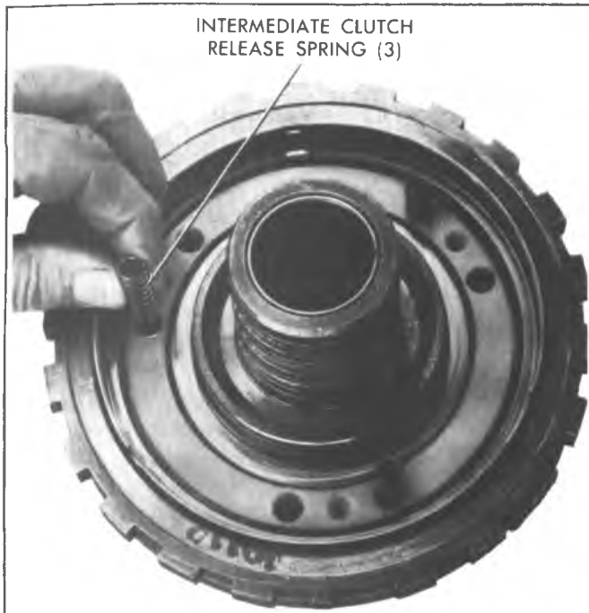
Fig. 7A-123C--Installing Intermediate Clutch Release Springs
