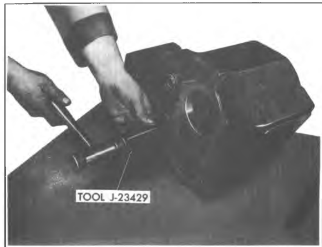
Fig. 7E-8R-Removing Idler Gear Shaft
