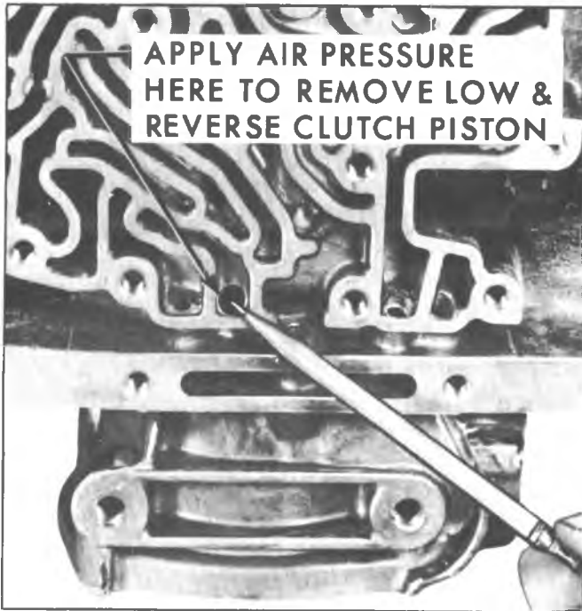
Fig. 7A-50B--Removing Low and Reverse Clutch Piston
