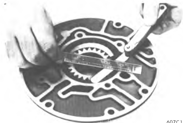
Figure 7A1-145 Checking Pump Body-to-Gear End Clearance
