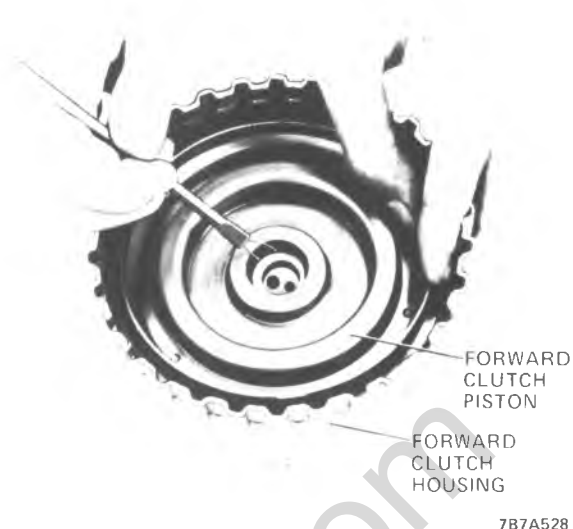
Figure 7A1-130 Installing Forward Clutch Piston
