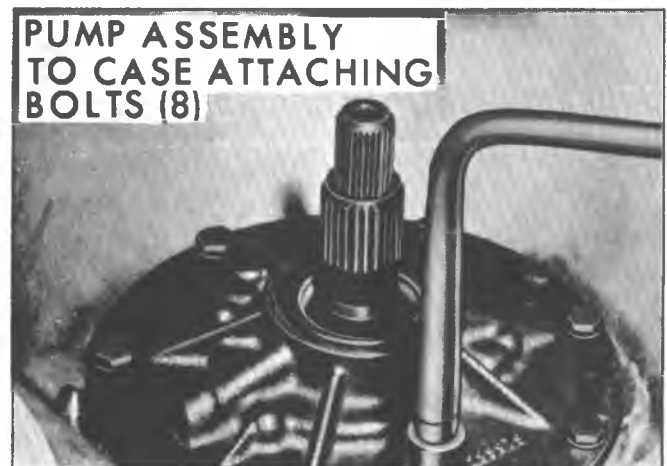
Fig. 7A-29B--Removing Pump Attaching Bolts
