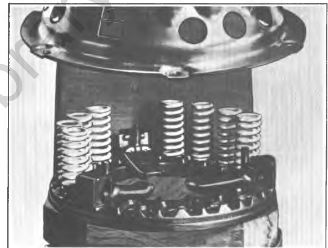
Fig. 7C-10E-Assembling Cover and Pressure Plate
