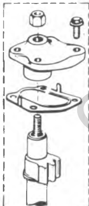
Separate pitman shaft and gasket seal from side cover if required.
