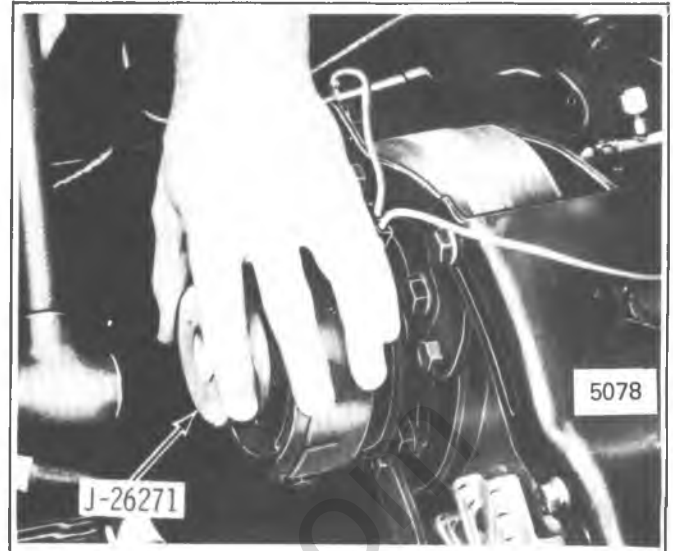
Figure 1D-87 Installing R-4 Rotor and Bearing Assembly (On Car)
