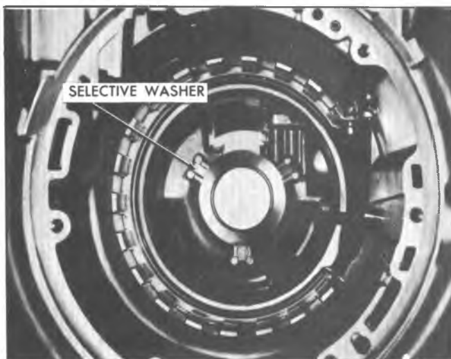
Fig. 7A-43C--Removing Selective Washer
