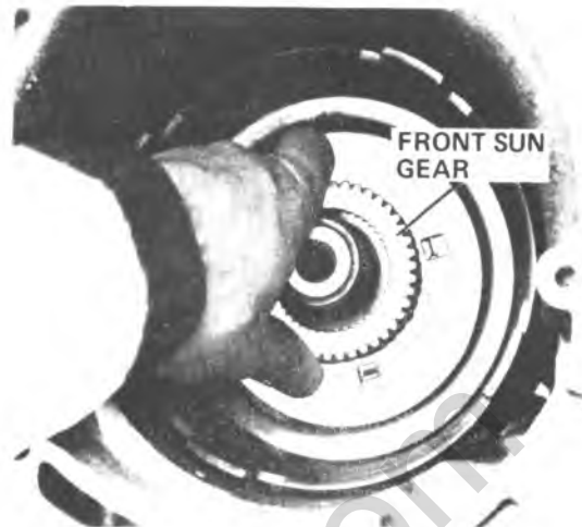
Figure 7A1-102 Installing Front Sun Gear
