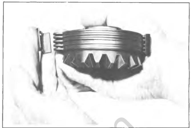
Fig. 9D-Assembling Clutch Pack
