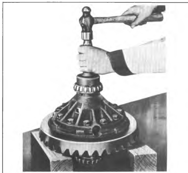
Fig. 5E-Differential Bearing Installation
