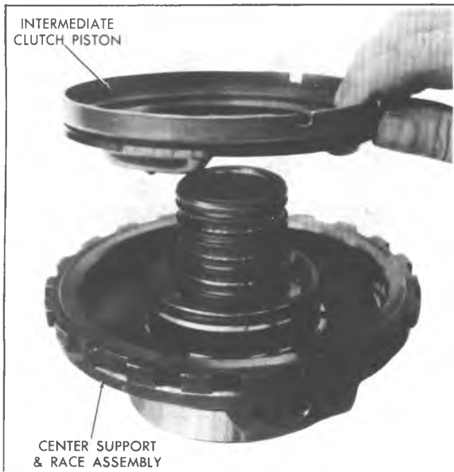
Fig. 7A-117C--Removing Intermediate Clutch Piston
