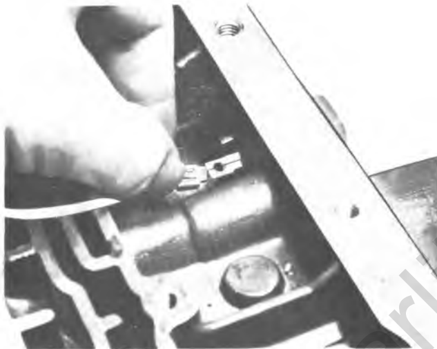
Figure 7A1-24A Removing Lead Wire
