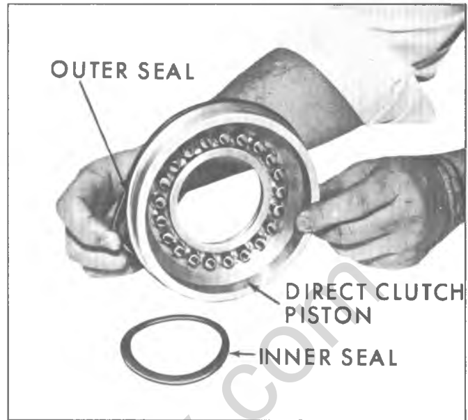
Fig. 66N--Removing Direct Clutch Outer and Inner Seals
