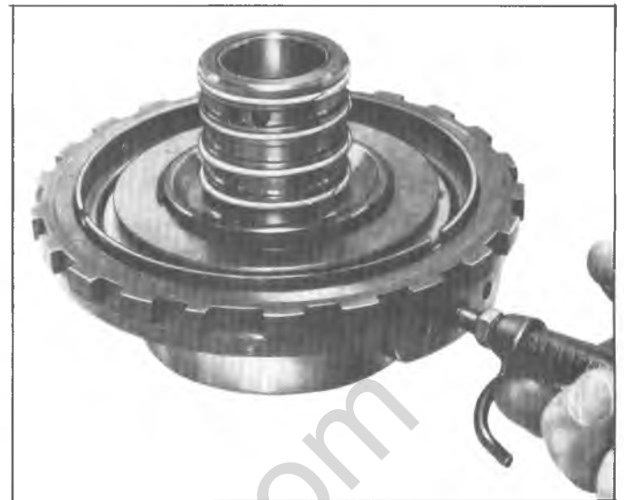
Fig. 104T—Air Checking Intermediate Clutch Piston
