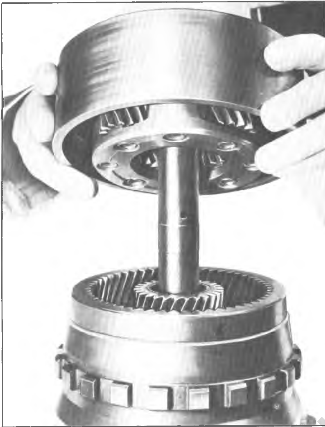
Fig. 121T--Installing Reaction Carrier
