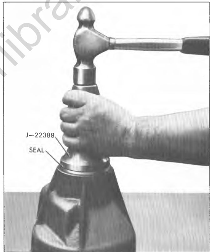
Fig. 18F—Installing Rear Output Housing Seal
