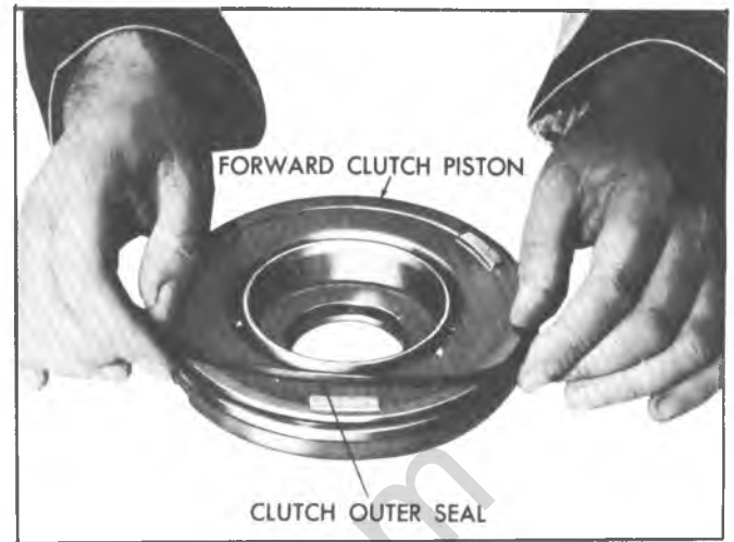
Fig. 71T--Removing Forward Clutch Piston Outer Seal
