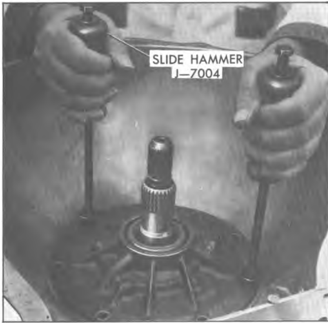
Fig. 26N--Removing Pump from Case
