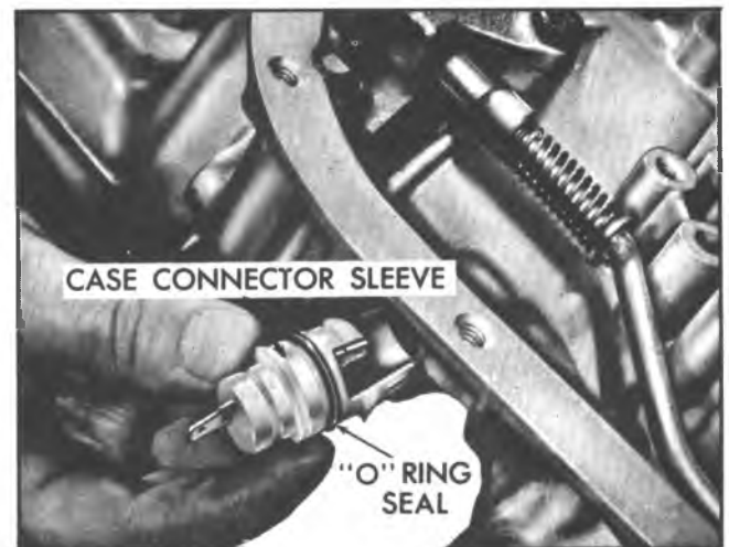
Fig. 15T--Removing Electrical Connector and "O" Ring Seal
