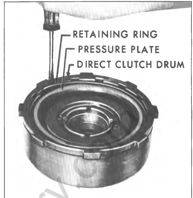
Fig. 63N--Removing Direct Clutch Pressure Plate
