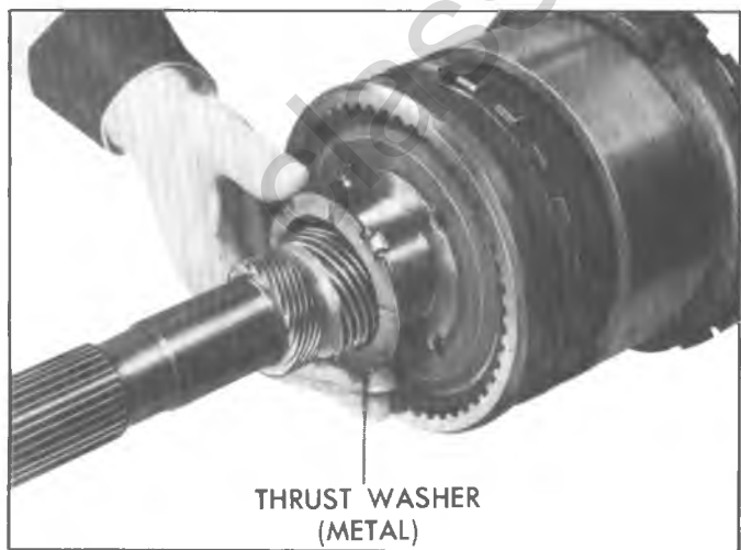
Fig. 126T--Installing Case to Output Shaft Thrust Washer
