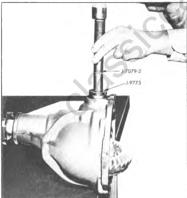
Fig. 6C—Installing Side Gear Yoke Bearings
