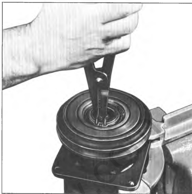
Fig. 6--Removing Pulley and Bearing Assembly Retainer Ring
