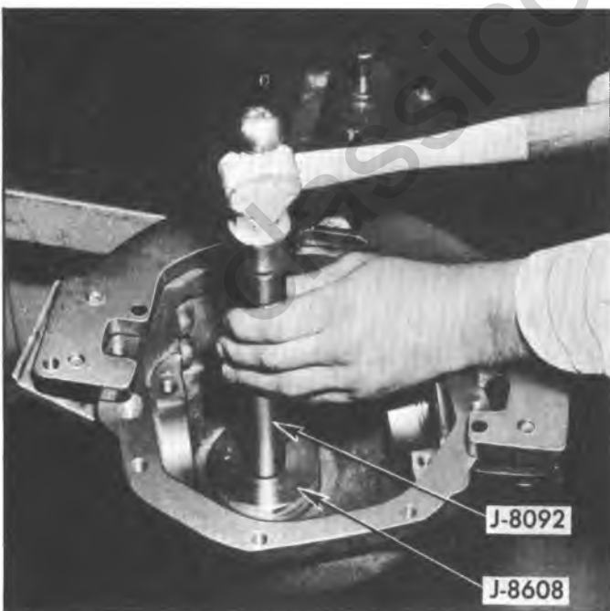
Fig. 18C—Installing Pinion Rear Bearing Cup
