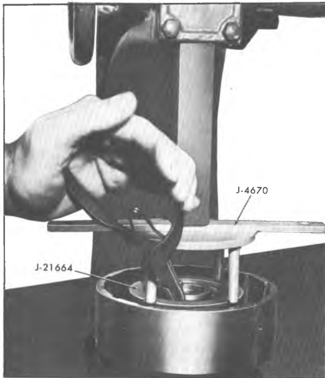
Fig. 70T--Removing Forward Clutch Spring Retaining Snap Ring
