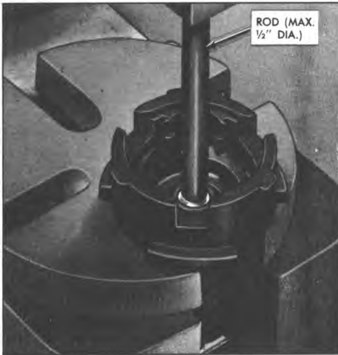
Fig. 9A--Removing Air Valve Assembly from Power Piston
