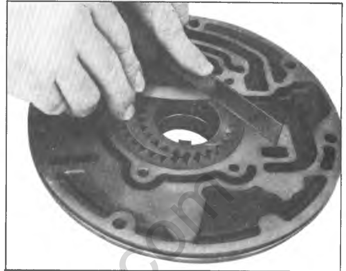
Fig. 65T-Checking Pump Body Face to Gear Face Clearance
