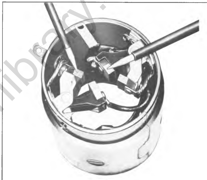
Fig. 7S--Field Coil Ground Test
