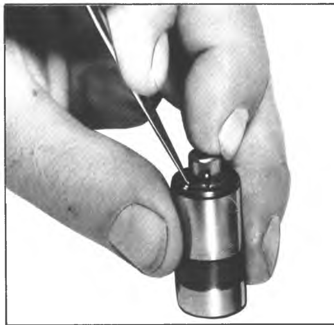
Fig. 32—Installing Ball Check Valve
