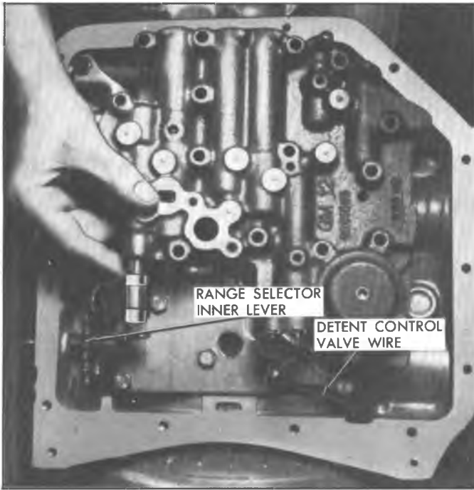
Fig. 12M--Removing Manual Control Valve Link, Valve Body and Detent Actuating Lever
