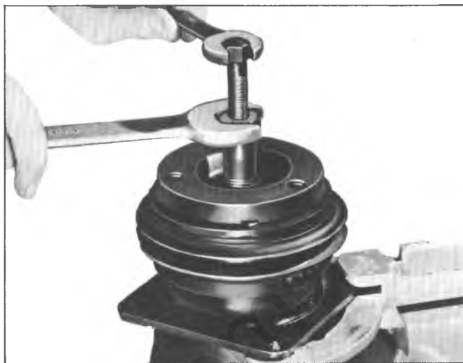
Fig. 3--Removing Hub and Drive Plate Assembly
