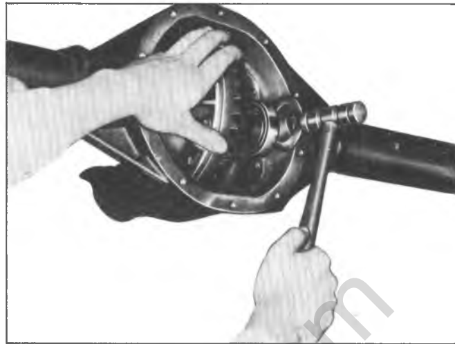
Fig. 9B—Installing Differential Shim
