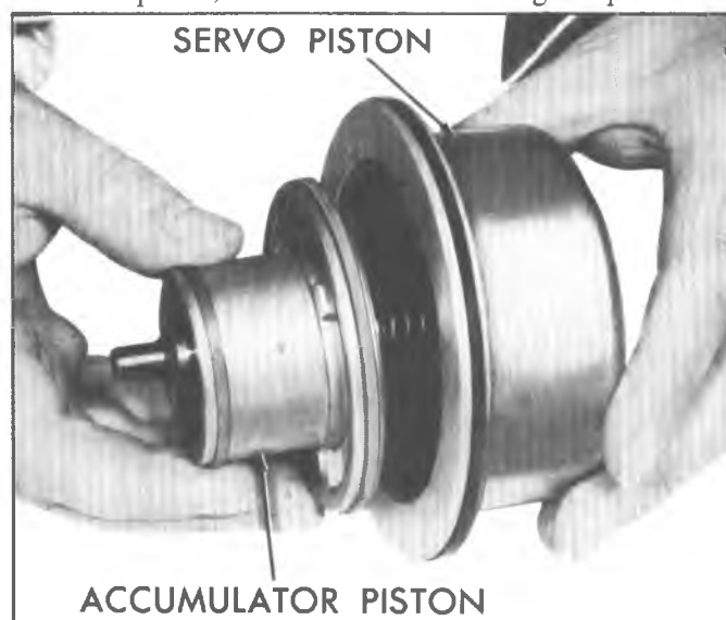
Fig. 50T-A--Removing Rear Accumulator Piston from Rear Servo Piston
