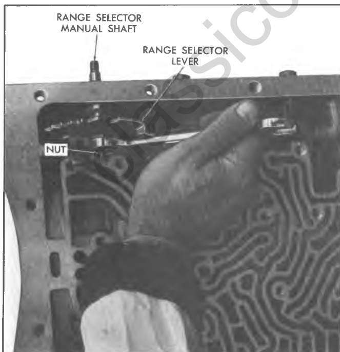
Fig. 19N--Loosening Nut Holding Range Selector Lever to Manual Shaft
