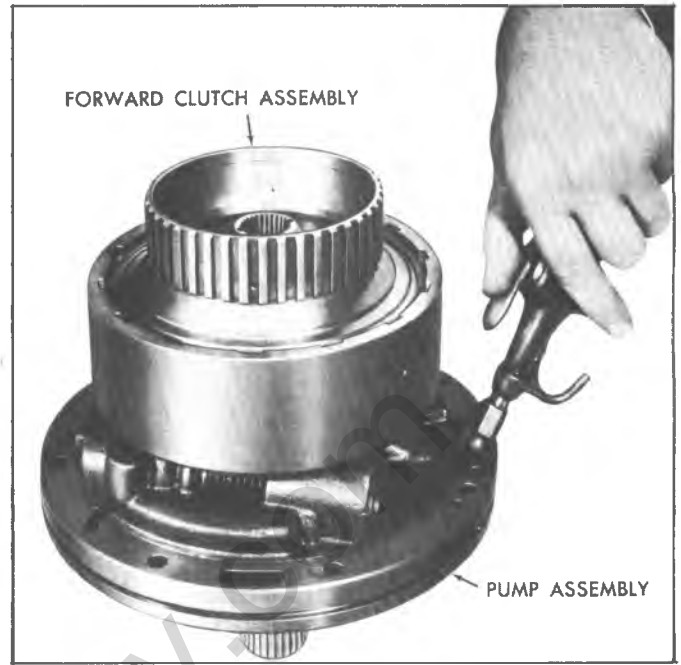
Fig. 77T--Air Checking Forward Clutch Assembly
