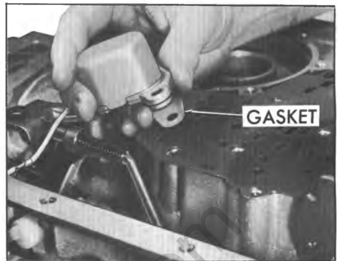
Fig. 14T--Removing Detent Solenoid and Gasket
