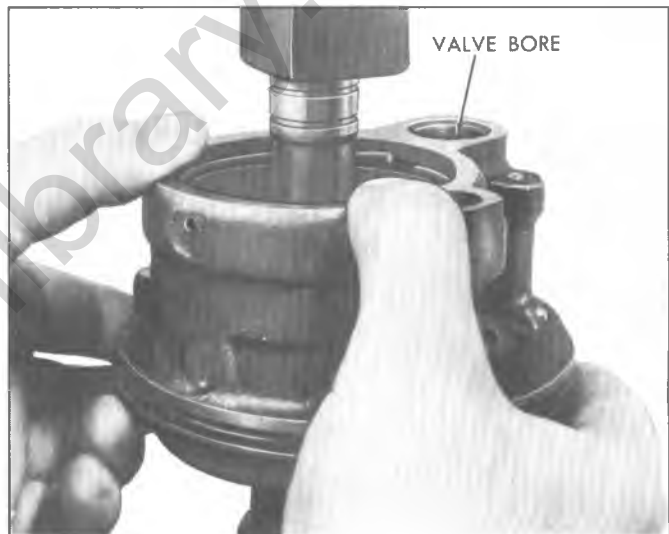
Fig. 29--Installing End Plate Retaining Ring
