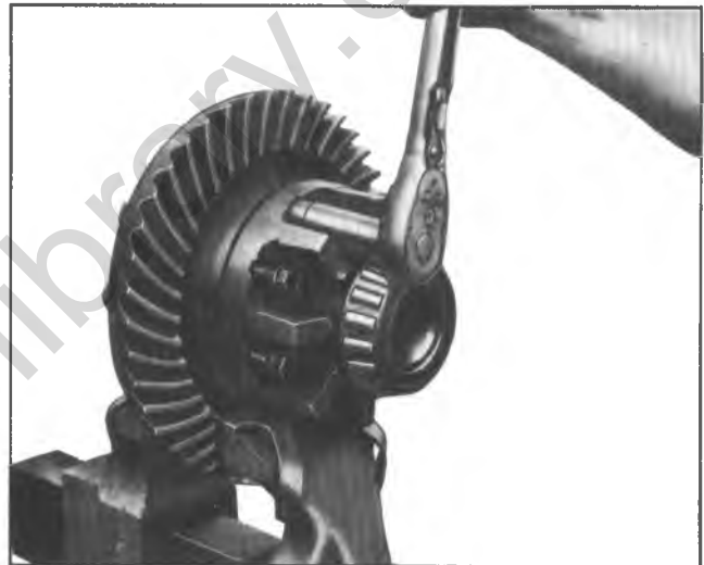
Fig. 3F—Separating Case Halves
