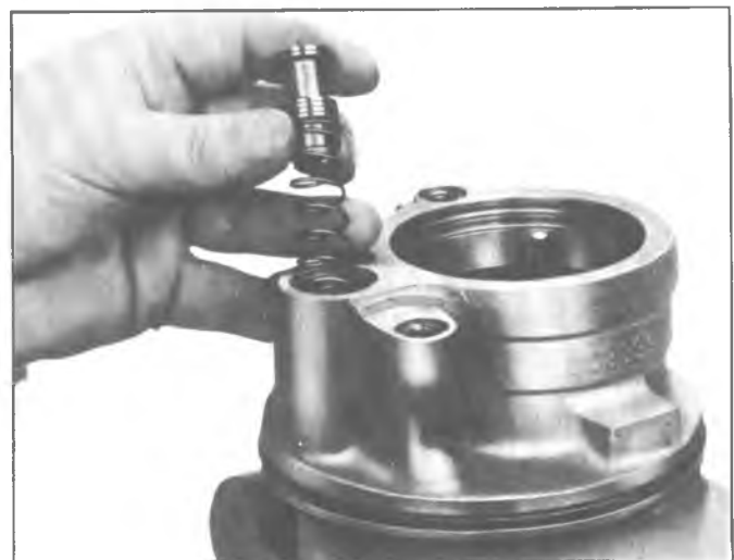
Fig. 30--Installing Flow Control Valve
