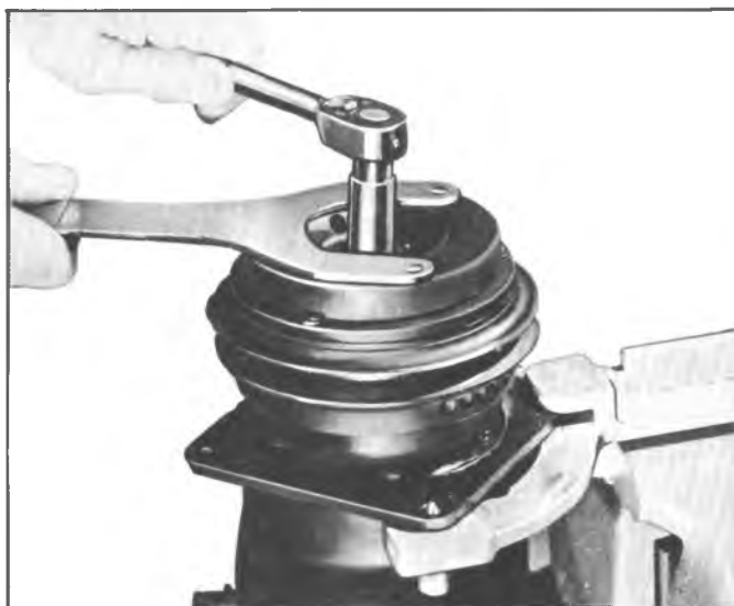
Fig. 2--Removing Shaft Locknut
