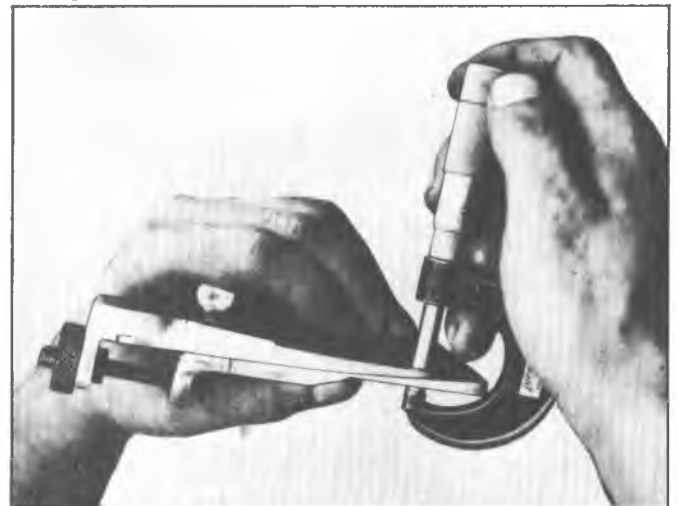
Fig. 10C—Measuring Gauge Plate Thickness
