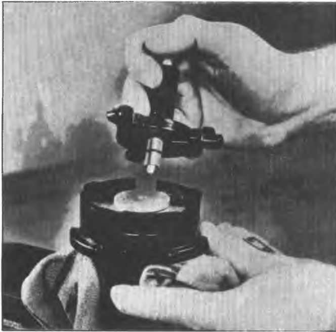
Fig. 12A-Installing Reaction Retainer on Power Piston
