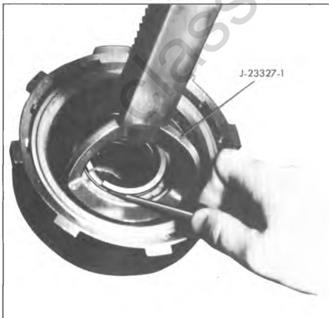
Fig. 65N--Compressing Direct Clutch Spring Seat
