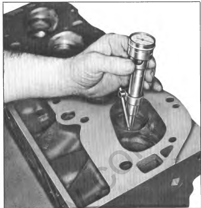
Fig. 24—Measuring Valve Seat Concentricity
