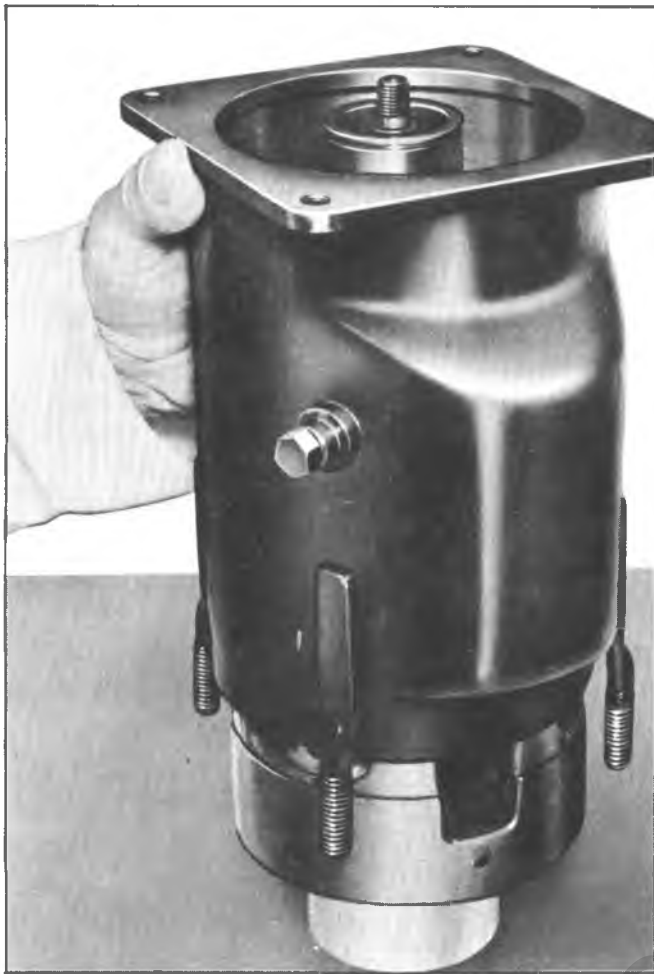
Fig. 27--Installing Shell Over Internal Mechanism
