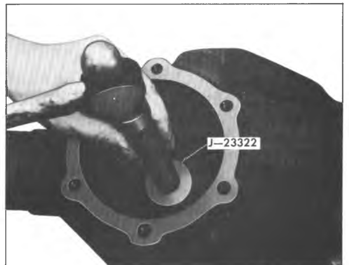
Fig. 14E—Installing Straddle Bearing
