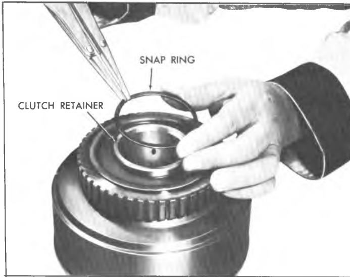
Fig. 95T--Installing Intermediate Clutch Retainer Snap Ring
