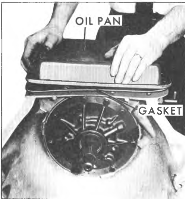
Fig. 9M--Removing Transmission Oil Pan
