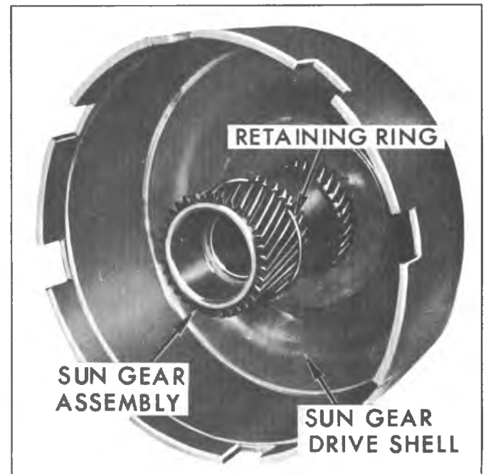
Fig. 82N--Removing Sun Gear to Drive Shell Front Steel Thrust Washer
