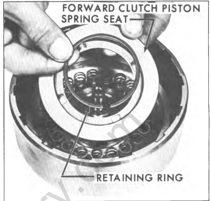
Fig. 69N--Installing Direct Clutch Springs, Spring Seat and Retaining Ring
