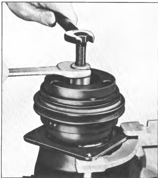
Fig. 5--Installing Hub and Drive Plate Assembly
