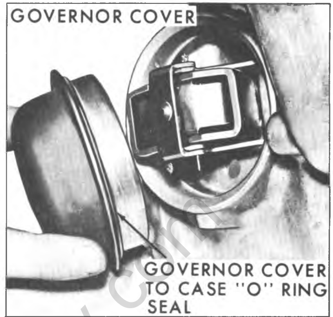
Fig. 7M-Governor Cover and "O" Ring Seal
