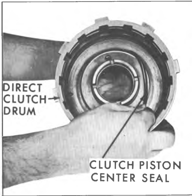
Fig. 74M--Removing Direct Clutch Piston Center Seal
