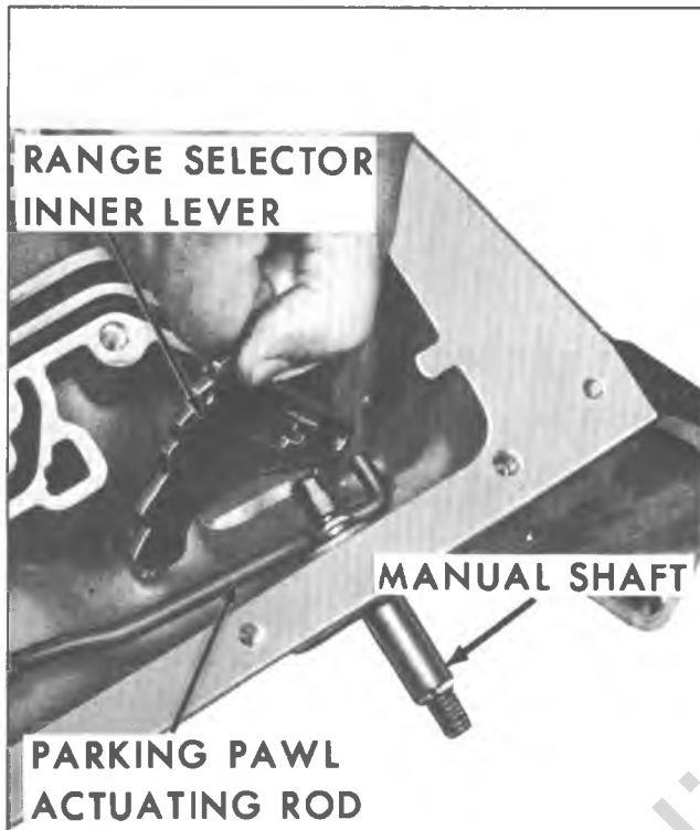
Fig. 20M--Removing Manual Shaft and Inner Lever and Parking Pawl Actuator Rod from Case
