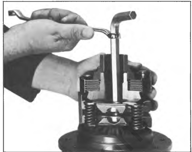
Fig. 5D—Removing Preload Spring Pack (Corvette)
