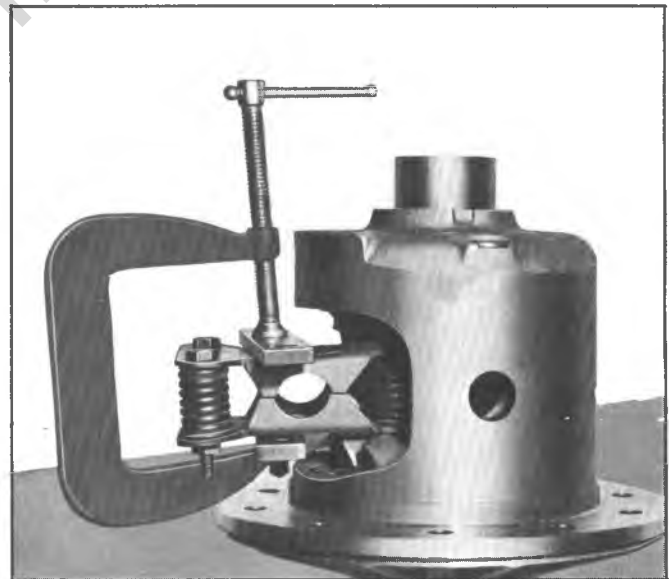
Fig. 6D— C-Clamp and Bar Stock Installed for Spring Removal
