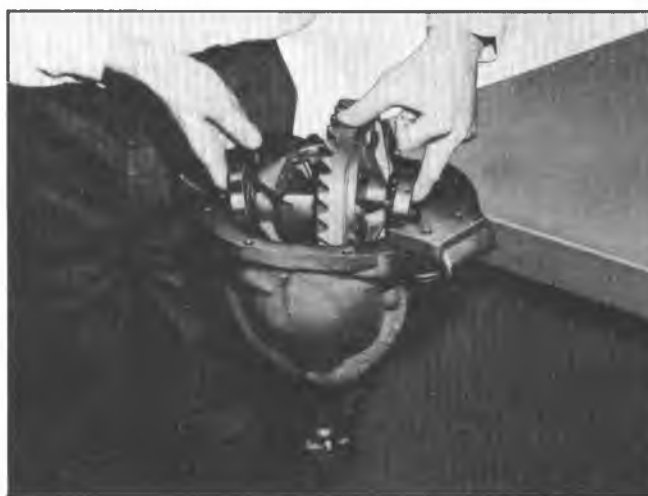
Fig. 8C—Installing Differential Assembly
