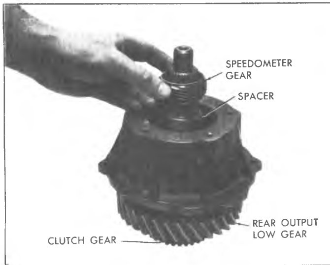
Fig. 18C-Installing Rear Output Shaft Spacer and Speedometer Gear
