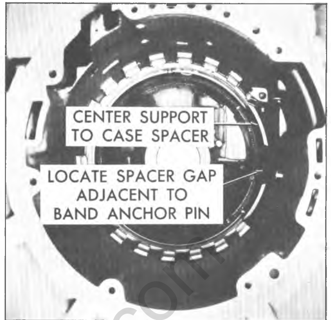
Fig. 129T-A--Installing Center Support to Case Spacer
