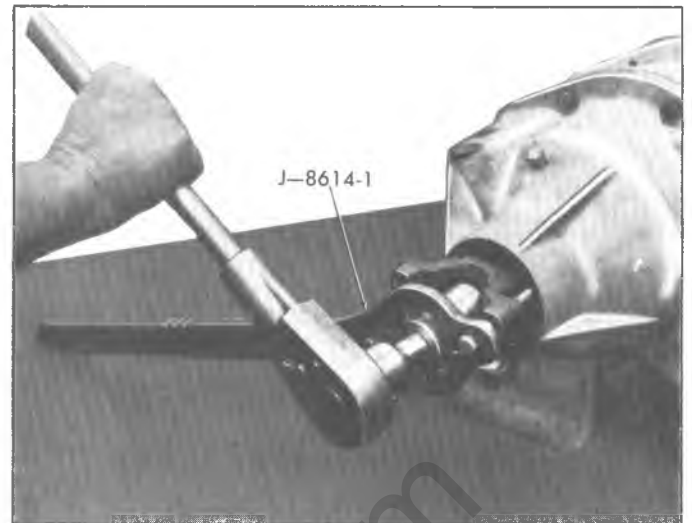
Fig. 4F—Removing Rear Output Shaft Flange Nut
