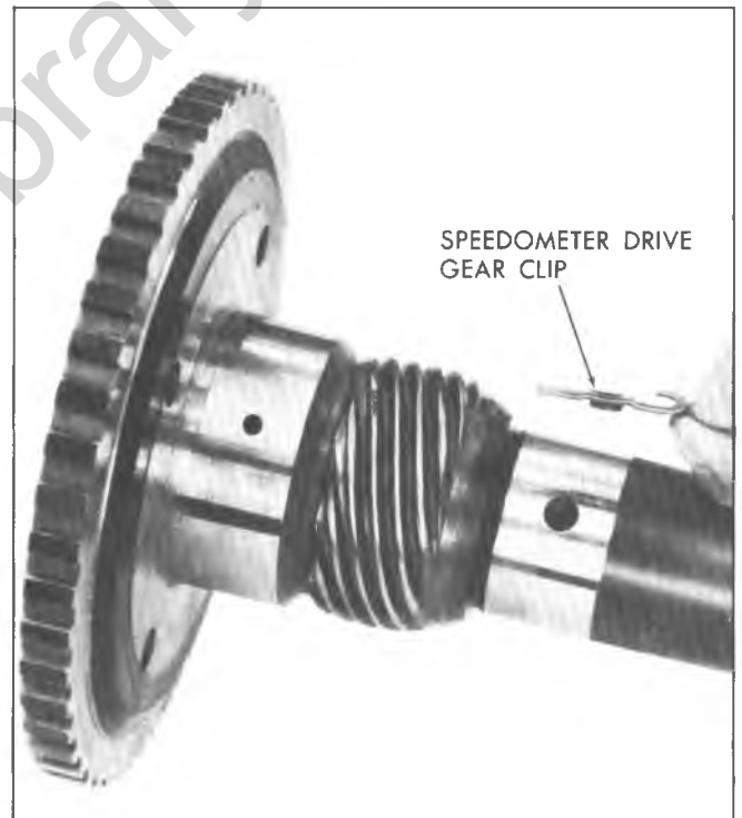
Fig. 47T--Installing Speedometer Drive Gear Clip
