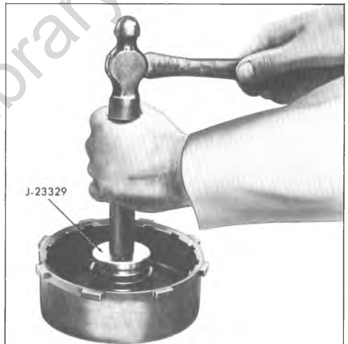
Fig. 102M--Installing Direct Clutch Drum Bushing
