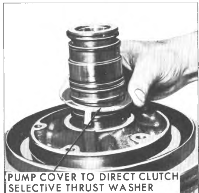
Fig. 104M--Pump Cover to Direct Clutch Selective Thrust Washer
