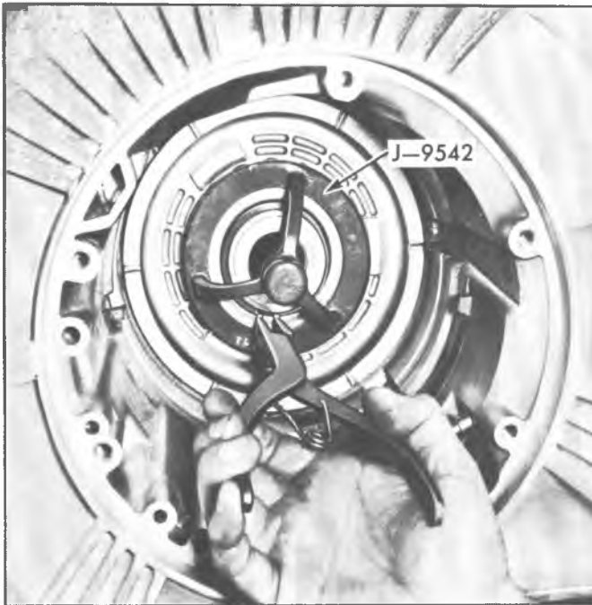
Fig. 8PG--Removing Rear Piston Spring Retainer Snap Ring
