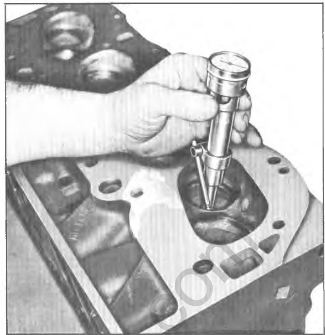
Fig. 24—Measuring Valve Seat Concentricity
