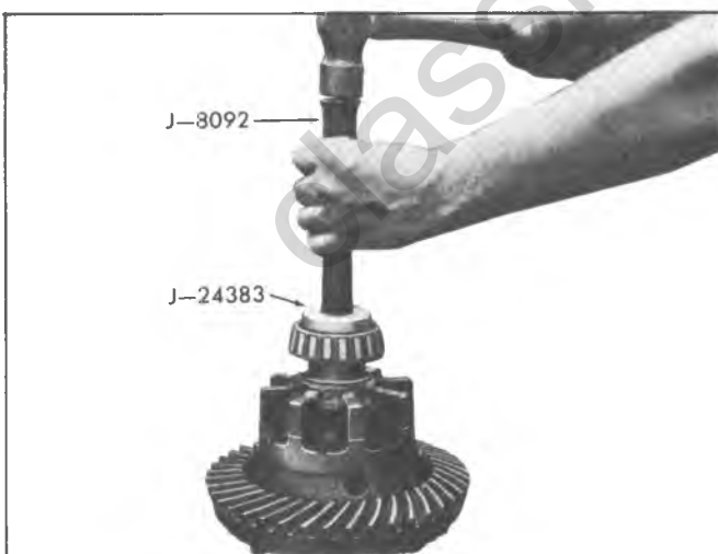
Fig. 7F—Installing Side Bearing
