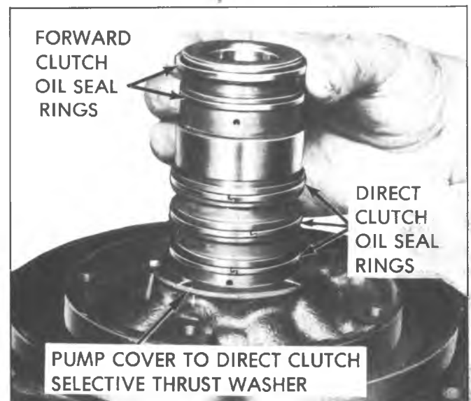
Fig. 58M--Pump Hub Oil Seal Rings
