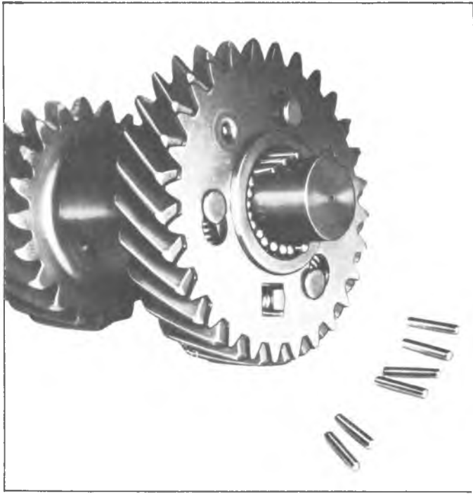
Fig. 19X--Loading Countergear Bearings
