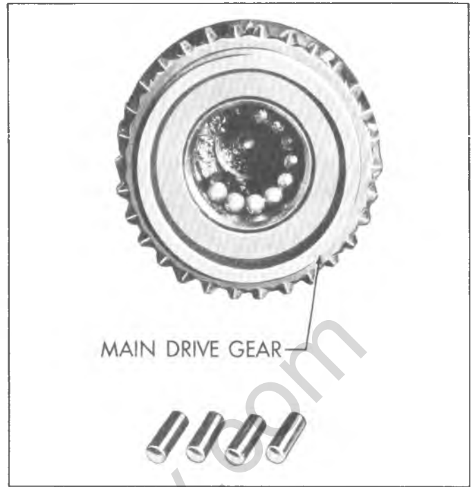
Fig. 20X--Loading Mainshaft Pilot Bearings
