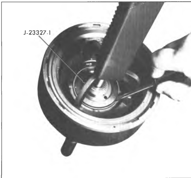
Fig. 80M--Compressing Forward Clutch Piston Return Seat
