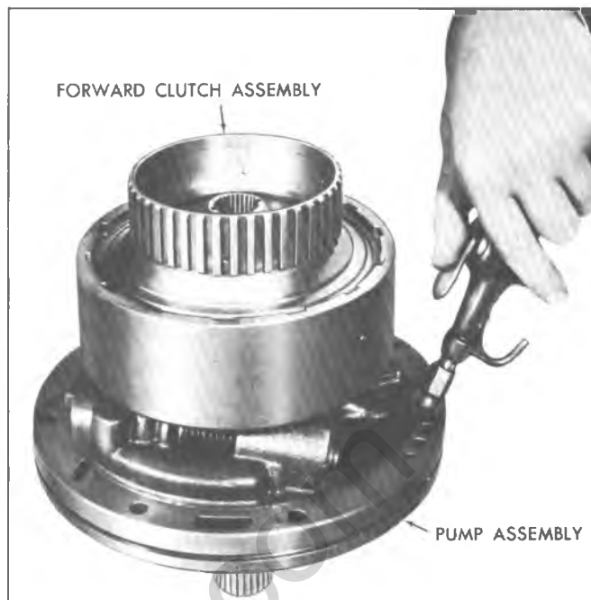
Fig. 77T--Air Checking Forward Clutch Assembly
