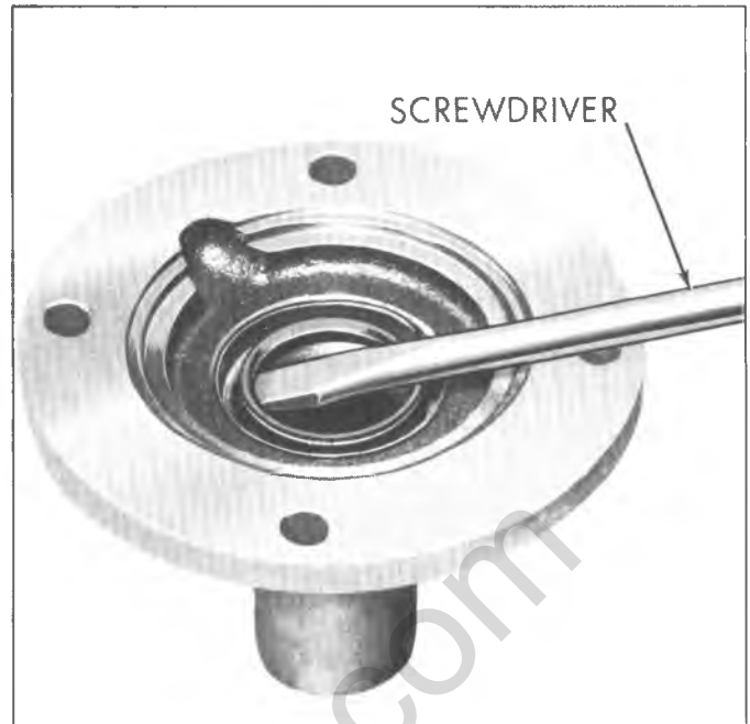
Fig. 14X-Removing Bearing Retainer Oil Seal
