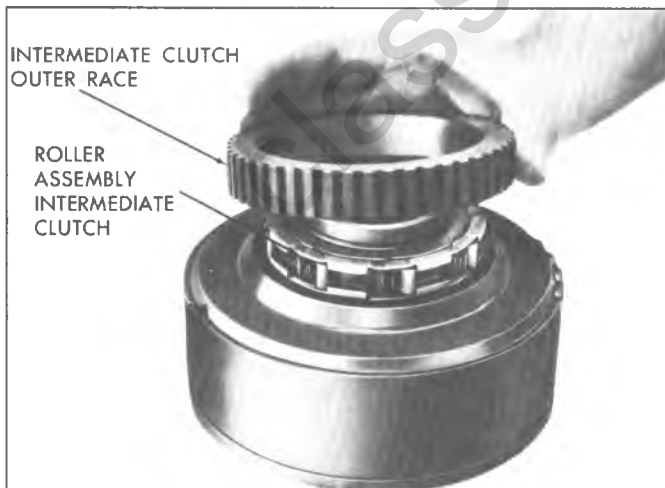
Fig. 92TA--Installing Intermediate Clutch Outer Race to Direct Clutch
