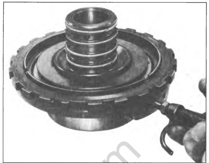
Fig. 104T—Air Checking Intermediate Clutch Piston
