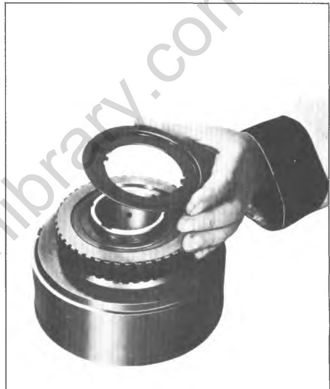
Fig. 94T--Installing Intermediate Clutch Retainer
