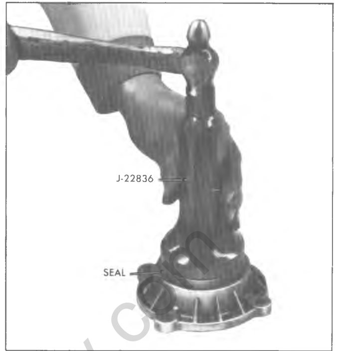
Fig. 16C-Installing Front Output Bearing Retainer Seal
