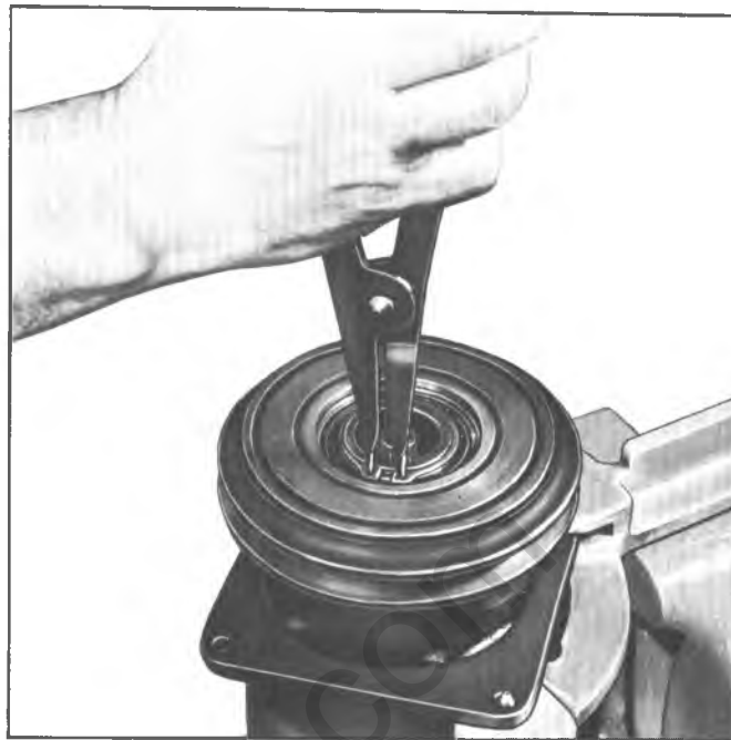
Fig. 6--Removing Pulley and Bearing Assembly Retainer Ring
