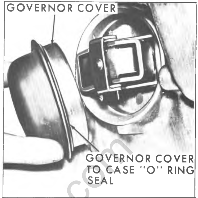
Fig. 7M--Governor Cover and "O" Ring Seal
