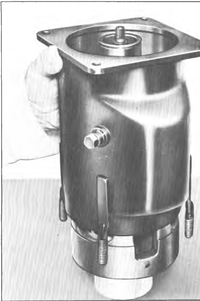
Fig. 27--Installing Shell Over Internal Mechanism
