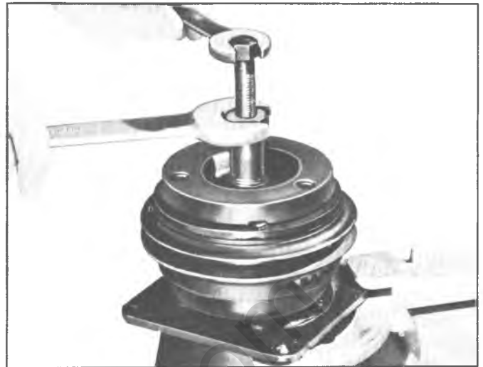
Fig. 3-Removing Hub and Drive Plate Assembly
