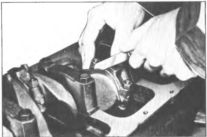
Fig. 45—Measuring Connecting Rod Side Clearance (In-Line)
