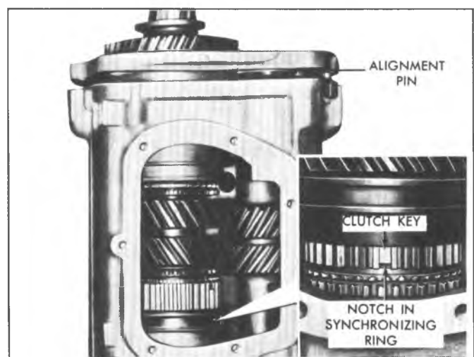
Fig. 18B-Installing Mainshaft Assembly
