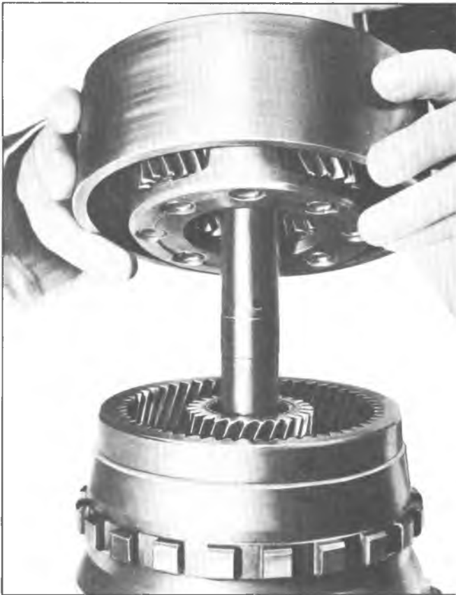
Fig. 121T--Installing Reaction Carrier
