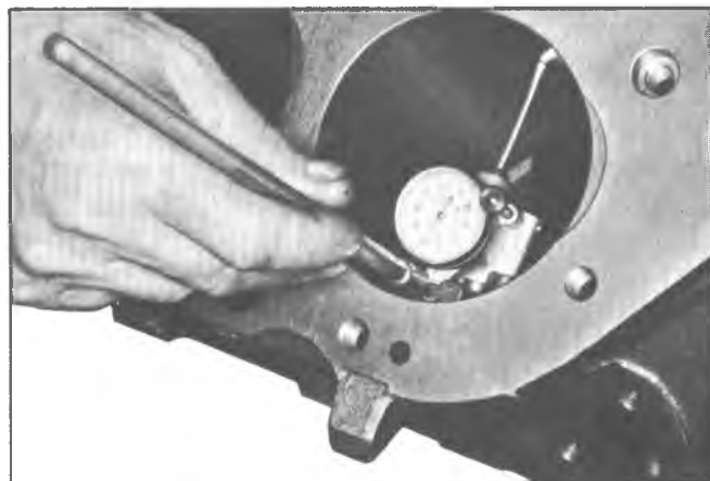
Fig. 69—Measuring Cylinder Bore
