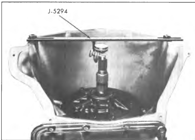
Fig. 105M--Checking End Play for Proper Thrust Washer Selection
