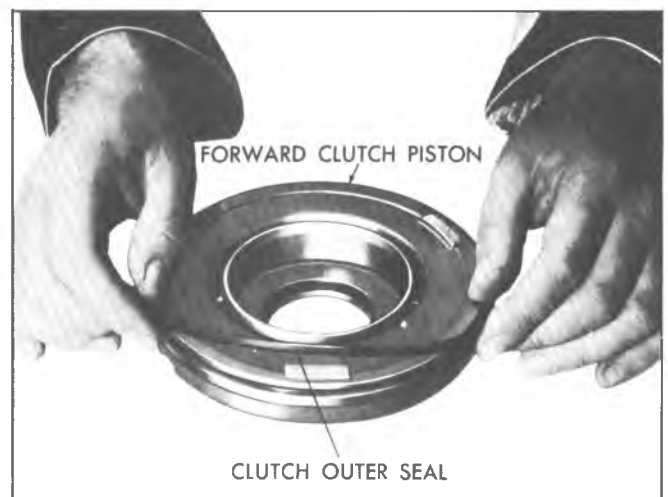
Fig. 71T--Removing Forward Clutch Piston Outer Seal
