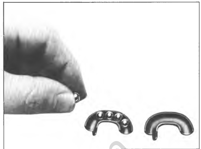
Fig. 13--Filling Ball Guides--Corvette
