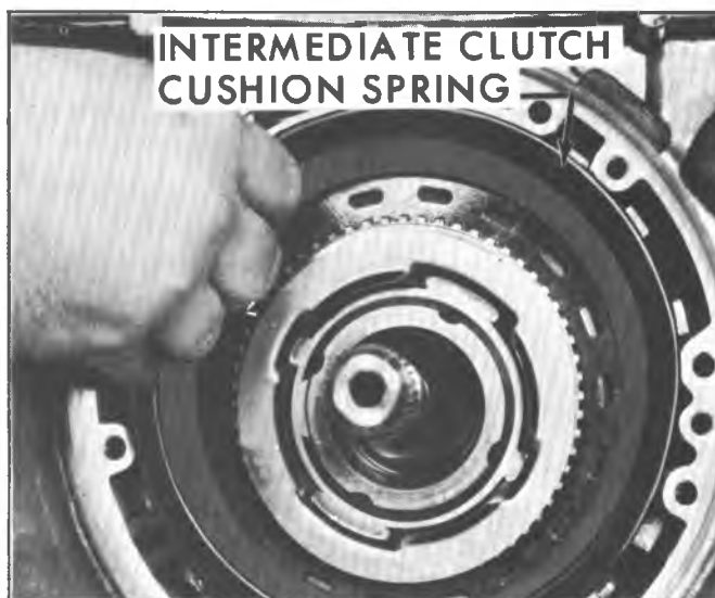
Fig. 28M--Removing Intermediate Clutch Cushion Spring
