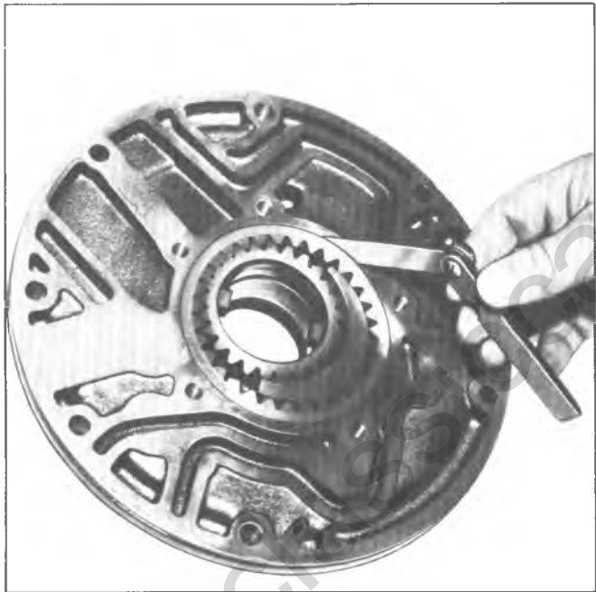
Fig. 17PG--Checking Driven Gear to Pump Body Clearance
