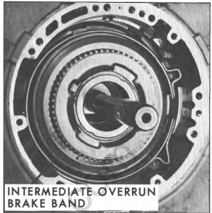
Fig. 31M--Removing Intermediate Overrun Brake Band
