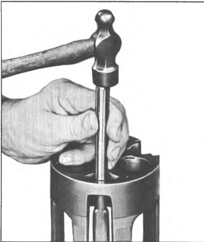
Fig. 18--Unseating Discharge Crossover Tube
