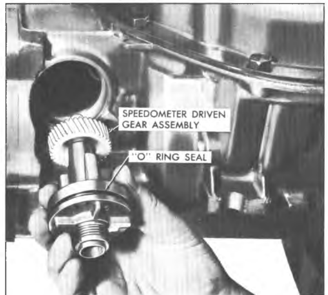
Fig. 155T--Installing Speedometer Driven Gear and Sleeve
