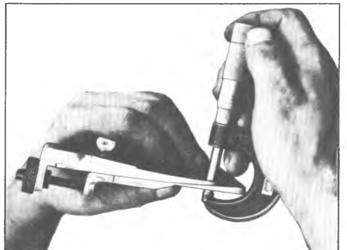
Fig. 10C—Measuring Gauge Plate Thickness
