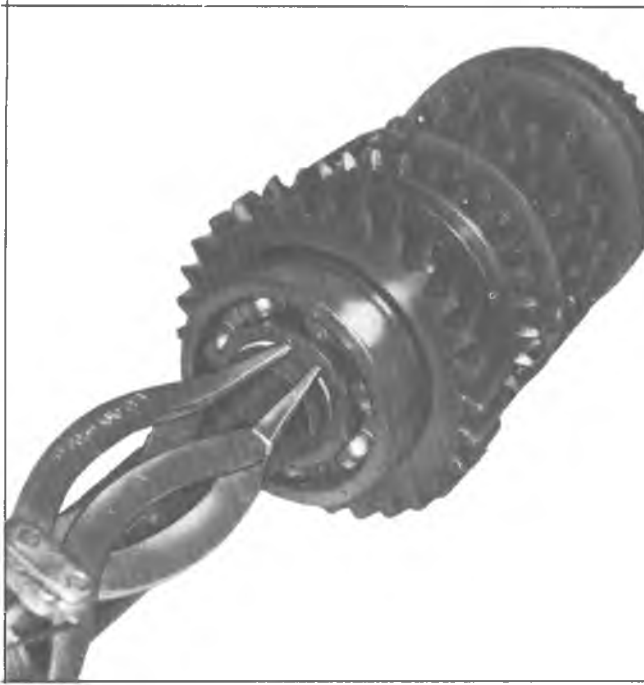
Fig. 8X-Rear Bearing to Mainshaft Snap Ring
