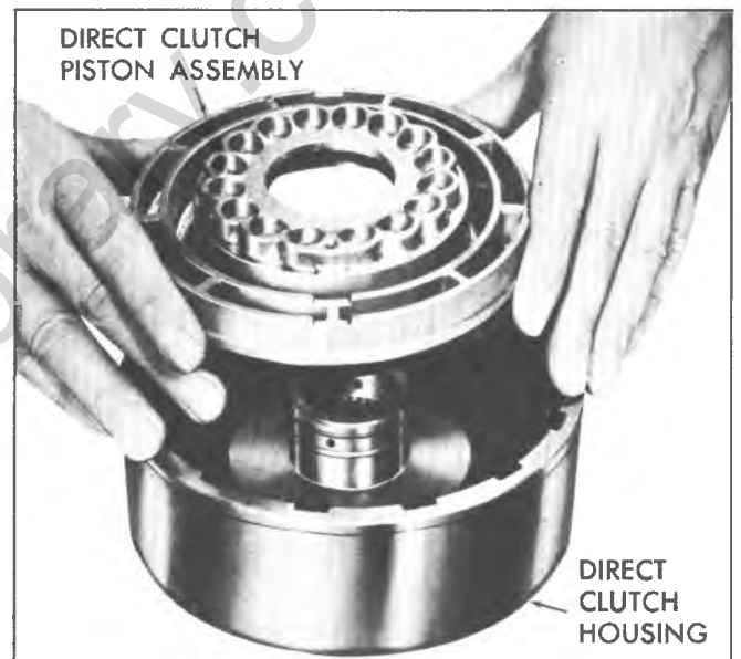
Fig. 82T--Removing Direct Clutch Piston Assembly
