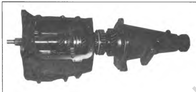
Fig. 3X--Removing Clutch Gear and Mainshaft
