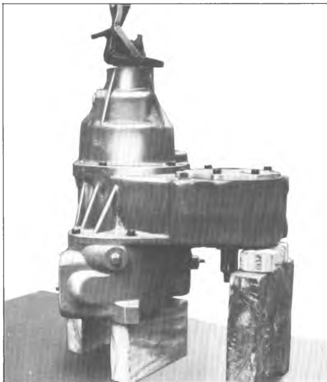
Fig. 6F—Positioning Transfer Case for Disassembly
