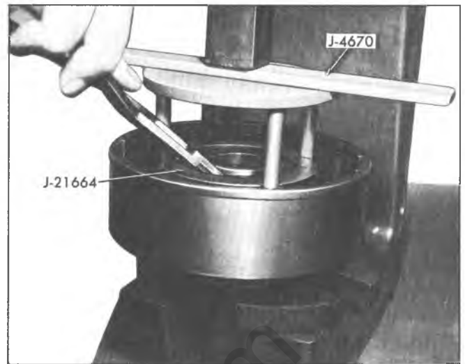
Fig. 81T--Removing or Installing Direct Clutch Snap Ring
