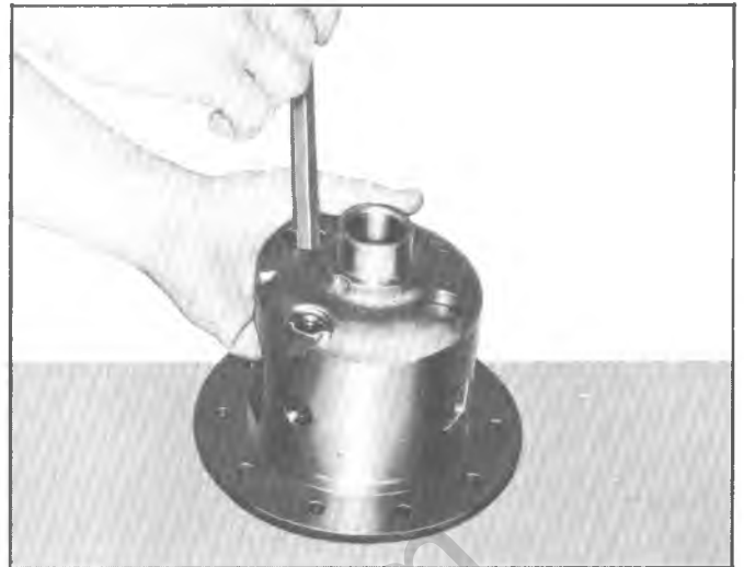
Fig. 9D—Removing Side Gear
