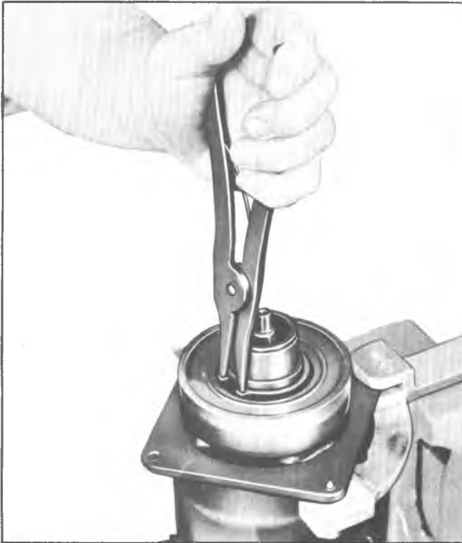
Fig. 8-Removing Coil Housing Retainer Ring
