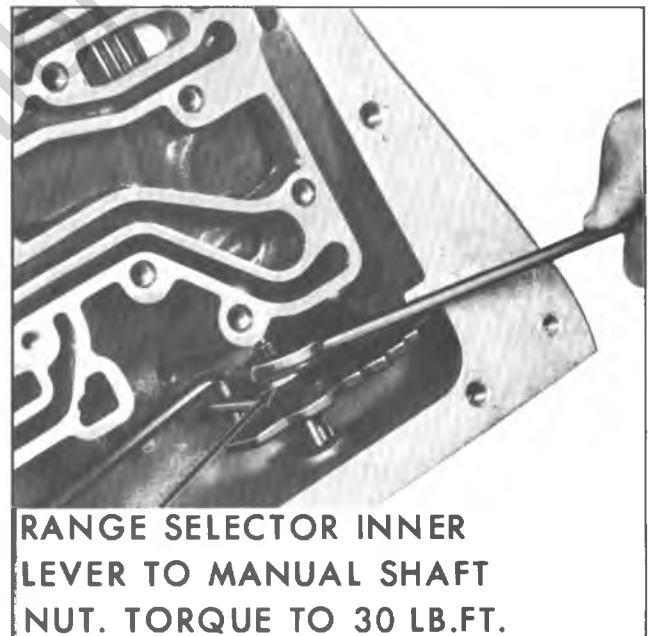
Fig. 19M--Loosening Nut Holding Range Selector Inner Lever to Manual Shaft
