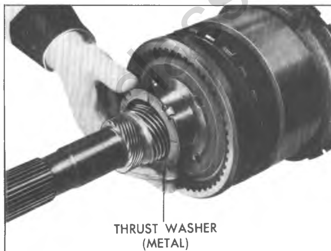
Fig. 126T--Installing Case to Output Shaft Thrust Washer
