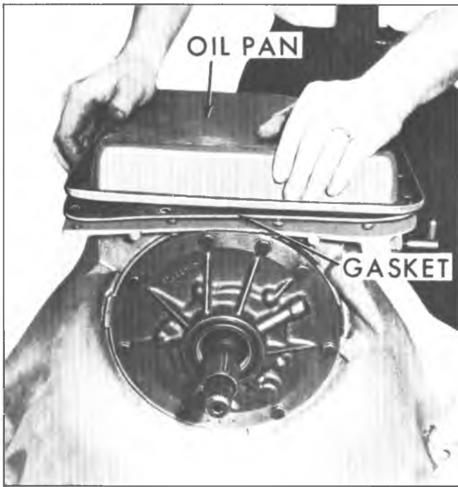
Fig. 9M--Removing Transmission Oil Pan
