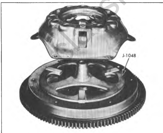
Fig. 11E--Gauge Plate Position
