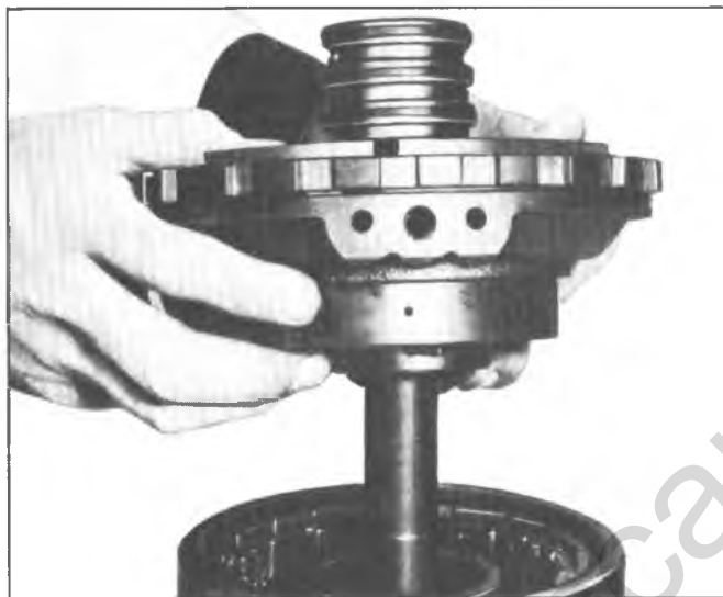
Fig. 125T--Installing Center Support to Reaction Carrier
