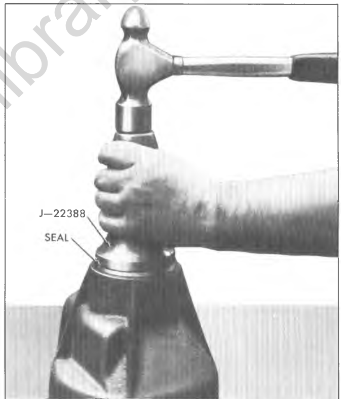
Fig. 19F—Installing Rear Output Housing Seal
