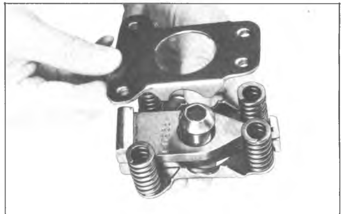
Fig. 13D—Installing Spring Pack Compression Tool (Corvette)
