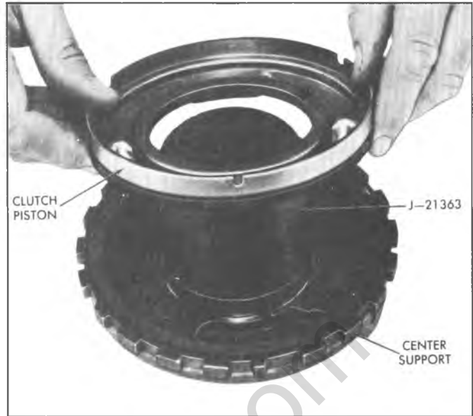
Fig. 102T--Installing Intermediate Clutch Piston
