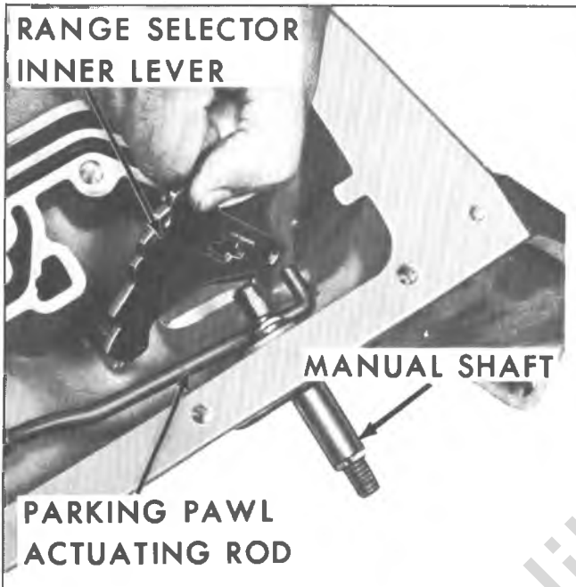
Fig. 20M--Removing Manual Shaft and Inner Lever and Parking Pawl Actuator Rod from Case
