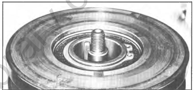
Fig. 4-Drive Plate Key Installed in Keyway
