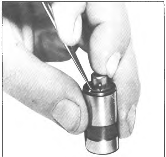
Fig. 32—Installing Ball Check Valve
