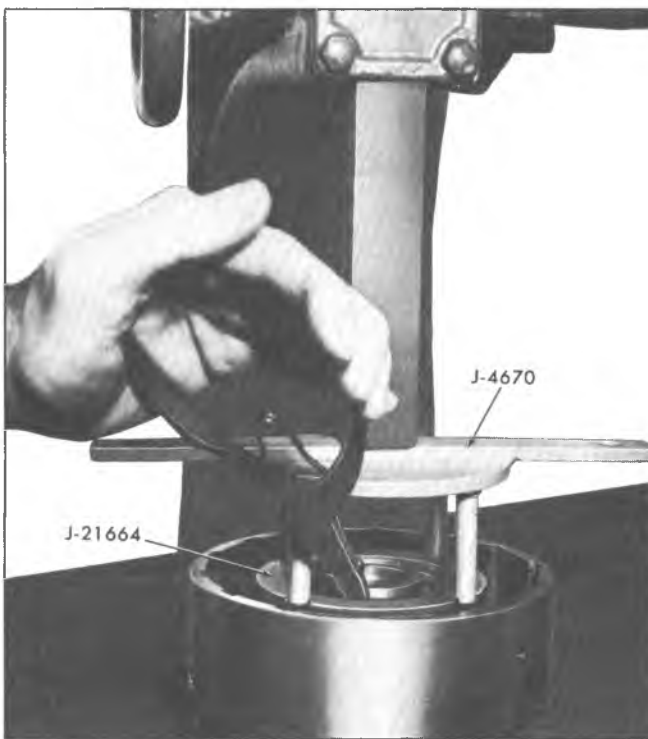
Fig. 70T--Removing Forward Clutch Spring Retaining Snap Ring
