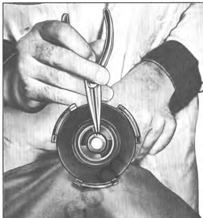
Fig. 9B--Locking or Unlocking Primary Support Plate From Primary Power Piston
