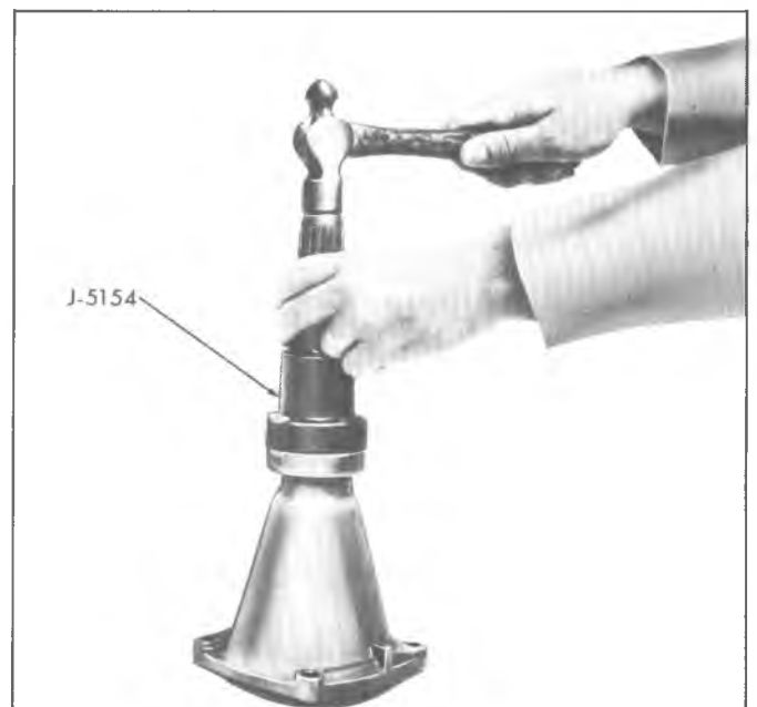
Fig. 106M--Installing Extension Housing Seal
