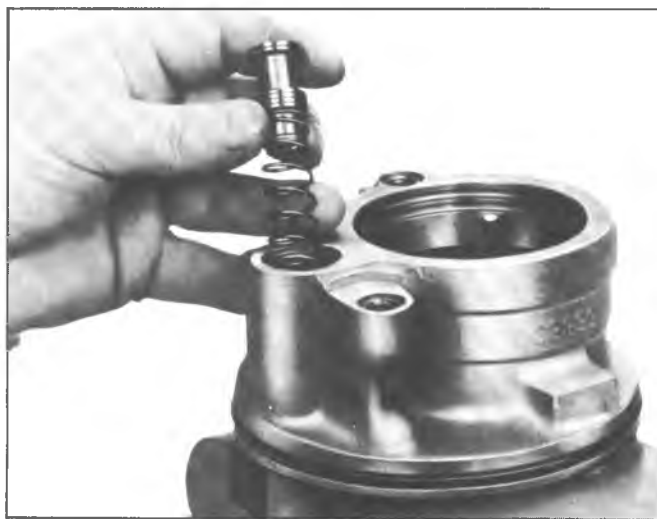
Fig. 30-Installing Flow Control Valve
