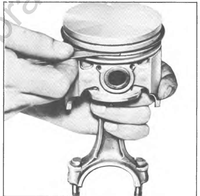
Fig. 58—Measuring Ring Groove Clearance
