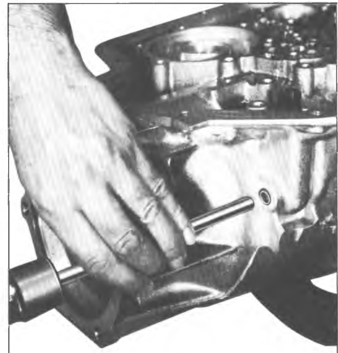
Fig. 127T--Installing Parking Pawl Shaft Cup Plug
