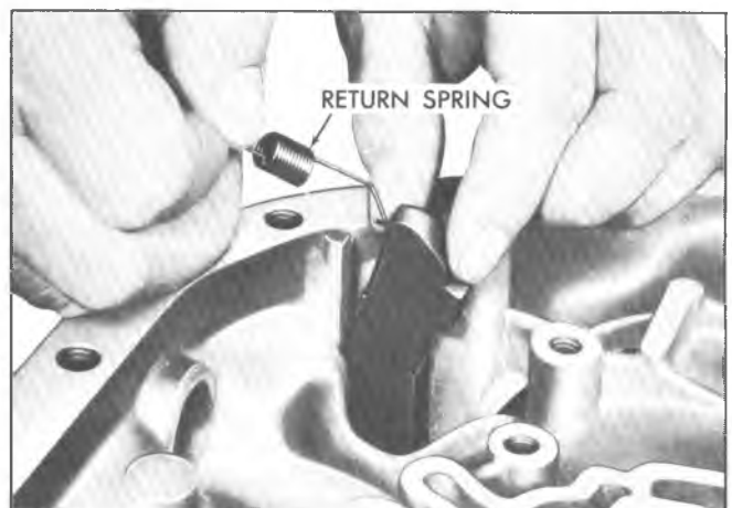
Fig. 20T--Removing Parking Pawl Return Spring
