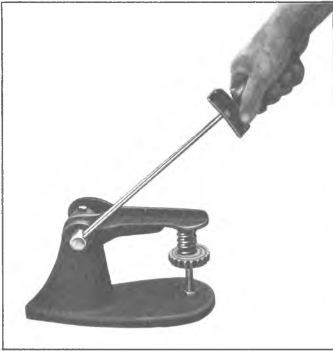
Fig. 17—Checking Valve Spring Tension
