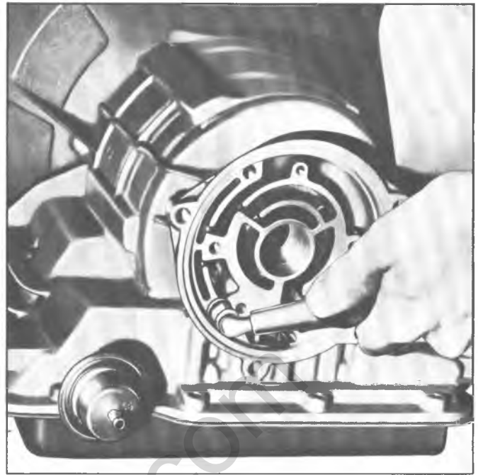
Fig. 9PG--Applying Air to Remove Rear Piston
