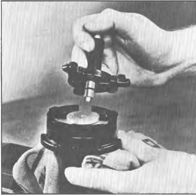
Fig. 12A--Installing Reaction Retainer on Power Piston
