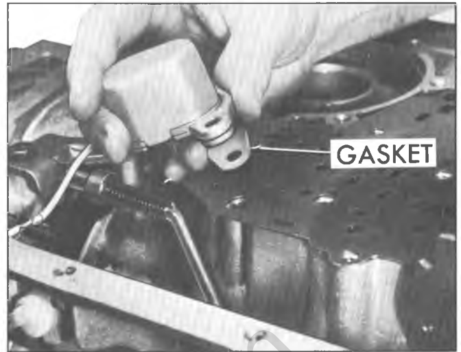
Fig. 14T-Removing Detent Solenoid and Gasket
