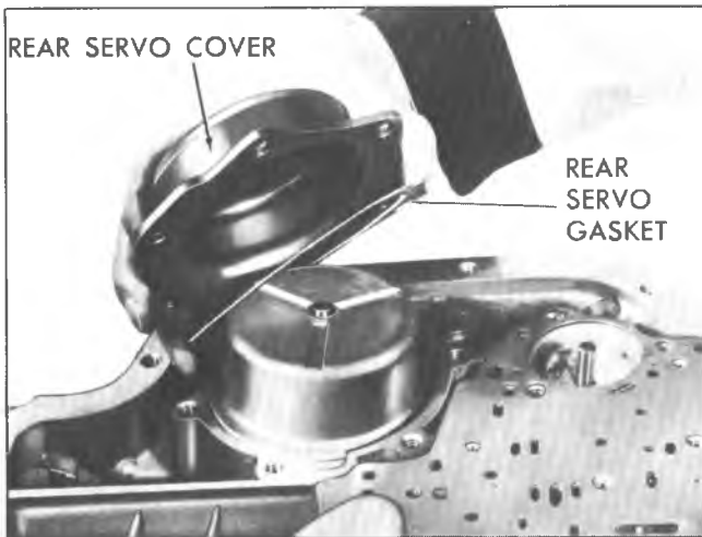
Fig. 149T-Installing Rear Servo Cover and Gasket
