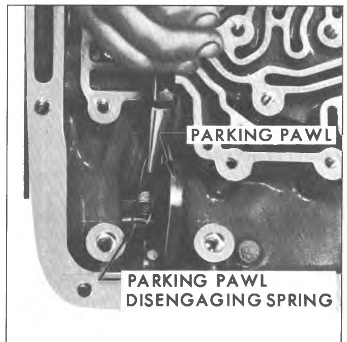
Fig. 23M--Removing Parking Pawl Disengaging Spring
