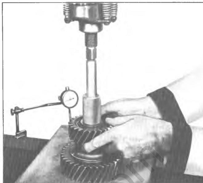
Fig. 11C-Checking Idler Gear End Play
