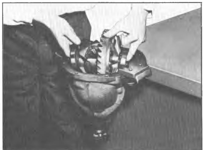
Fig. 8C—Installing Differential Assembly
