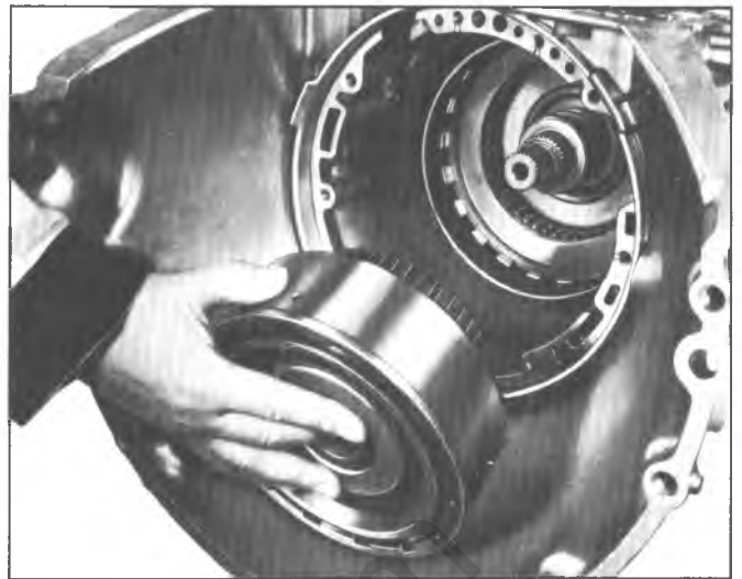
Fig. 29T--Removing Direct Clutch Assembly
