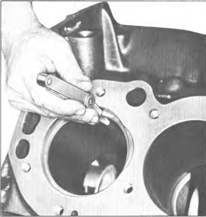
Fig. 55—Measuring Ring Gap
