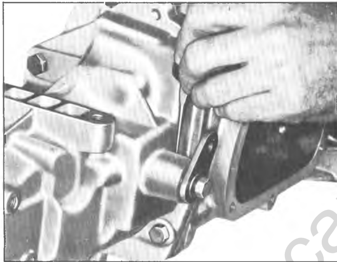
Fig. 4B--Removing Reverse Shifter Shaft Lock Pin
