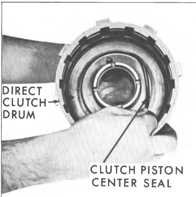
Fig. 74M--Removing Direct Clutch Piston Center Seal
