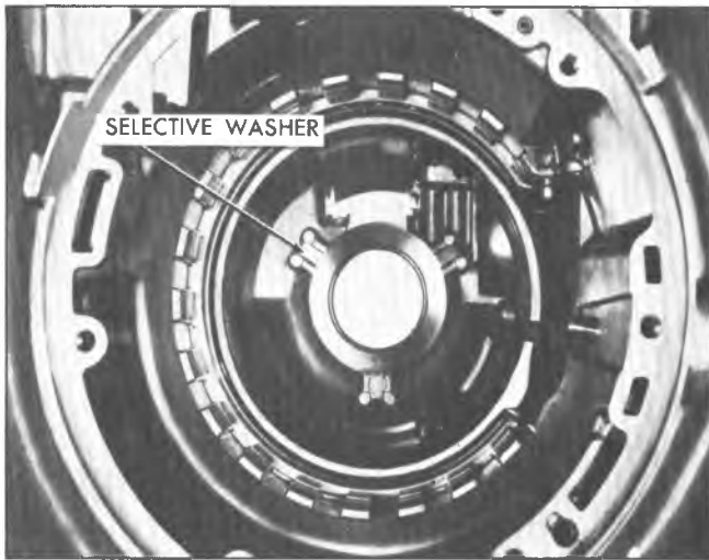
Fig. 37T-Removing Selective Washer
