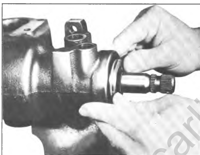
Fig. 56--Installing Valve Body
