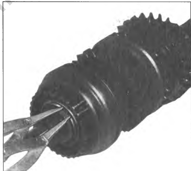
Fig. 7X--Third and Fourth Synchronizer Snap Ring
