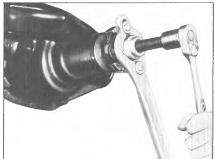
Fig. 13B—Drive Pinion Flange Removal
