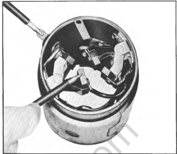
Fig. 6S-Field Coil Open Circuit Test
