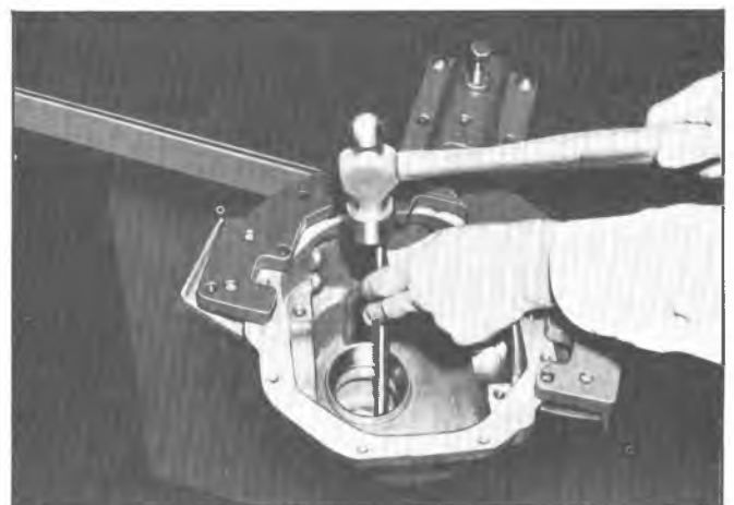
Fig. 16C—Removing Pinion Bearing Cup
