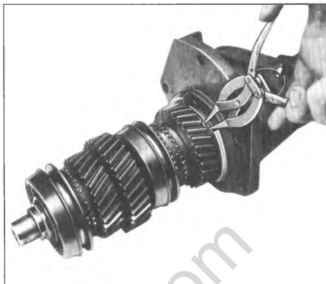
Fig. 3G--Removing Rear Extension From Mainshaft
