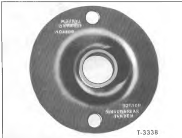
Figure 8—Electric Shift Unit Seal Markings
