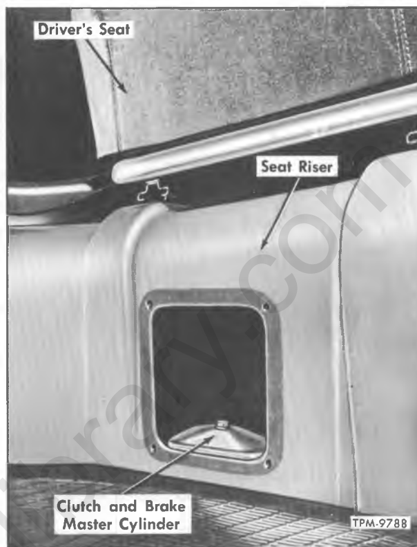
Figure 10—Access to Master Cylinder
