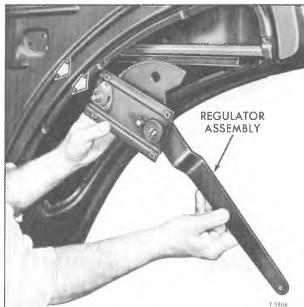
Figure 19—Lowering Regulator from Door
