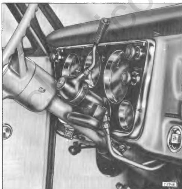
Figure 16—Trailer Brake Hand Control Valve Installed
