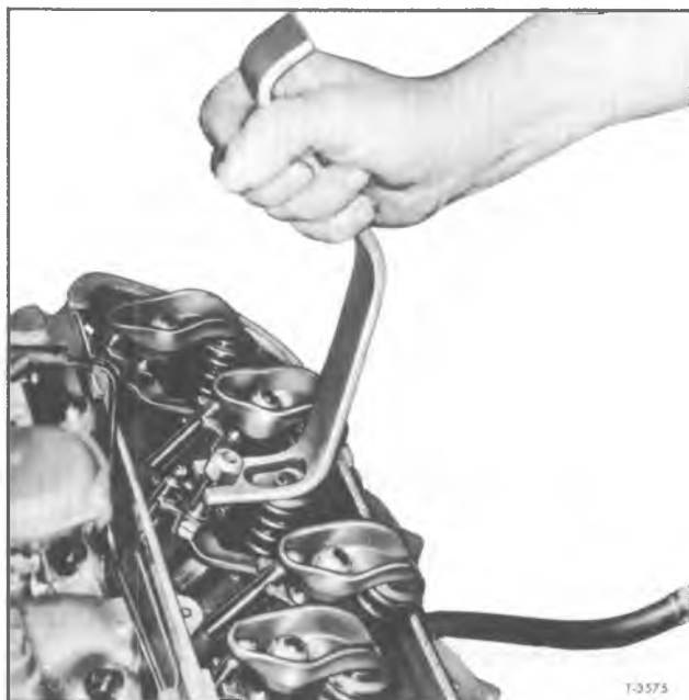
Figure 31 — Compressing Valve Spring on V8 Engine
