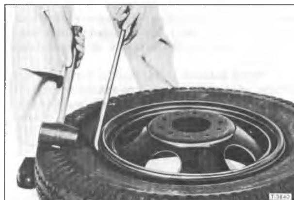
Figure 19—Starting Side Ring Removal
