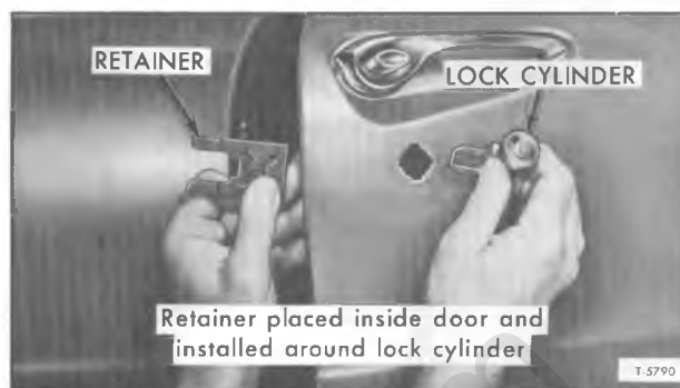
Figure 14—Door Lock Cylinder Replacement
