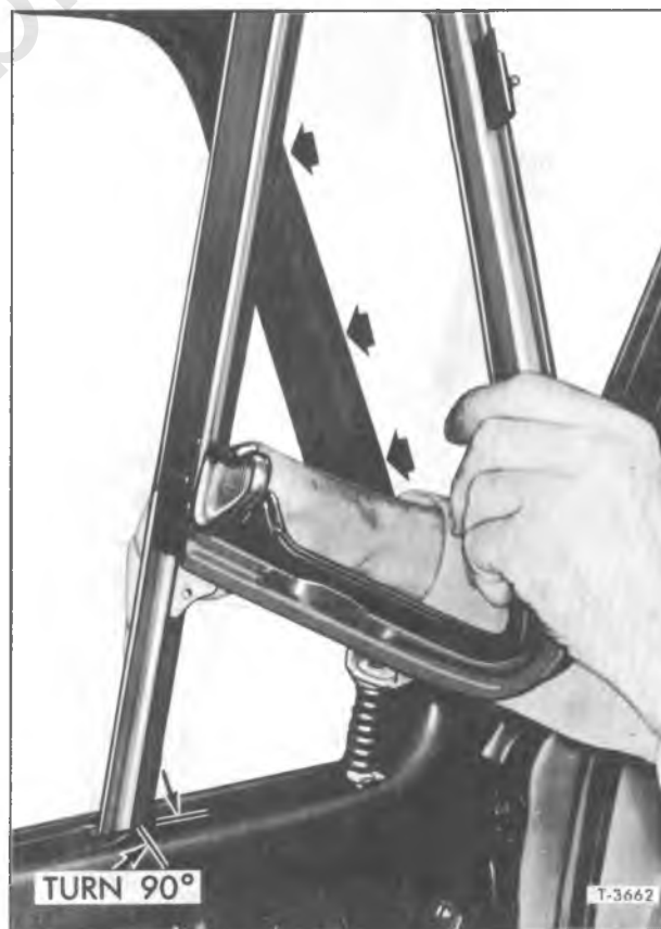
Figure 20—Vent Window Assembly Removal
