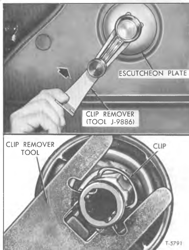
Figure 15—Disengaging Door Inside Handle
