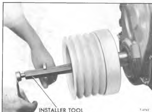
Figure 39—Installing Damper Assembly (Typical)
