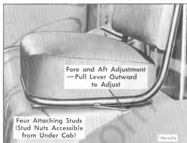
Figure 5—Driver's Seat Mounting and Adjustment
