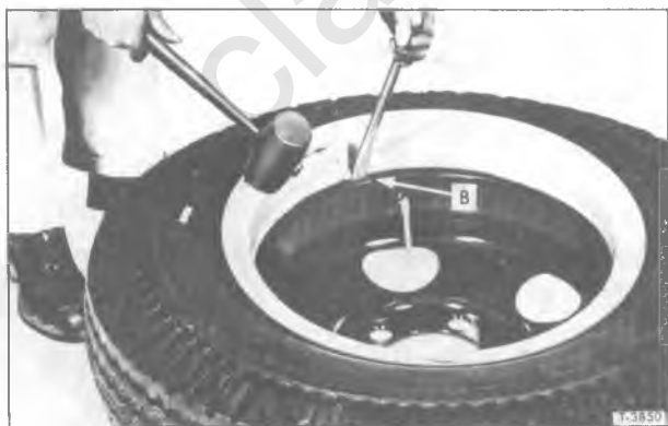
Figure 15—Engaging Side Ring Over Rim Gutter
