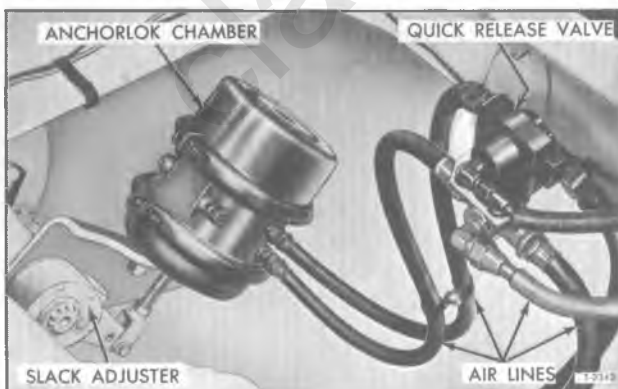
Figure 19—Anchorlok Brake Chamber Installed
