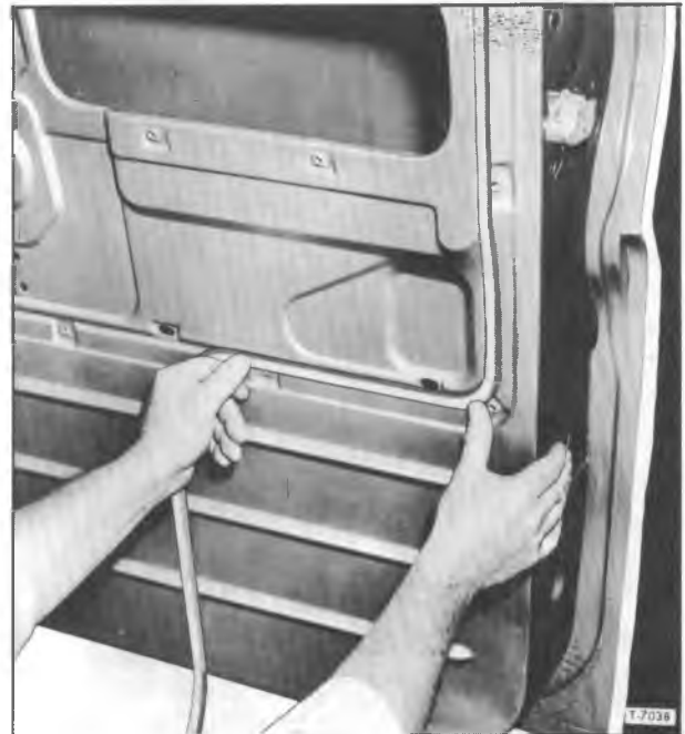
Figure 24—Installing Trim Panel Seal
