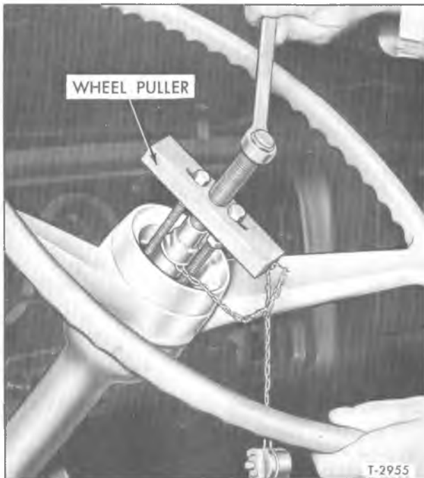
Figure 13—Steering Wheel Removal (Typical)
