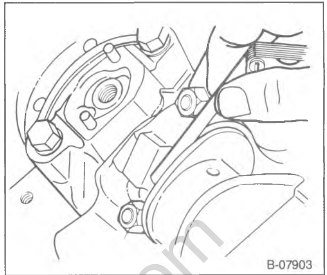
Figure 32—Measuring Connecting Rod Side Clearance
