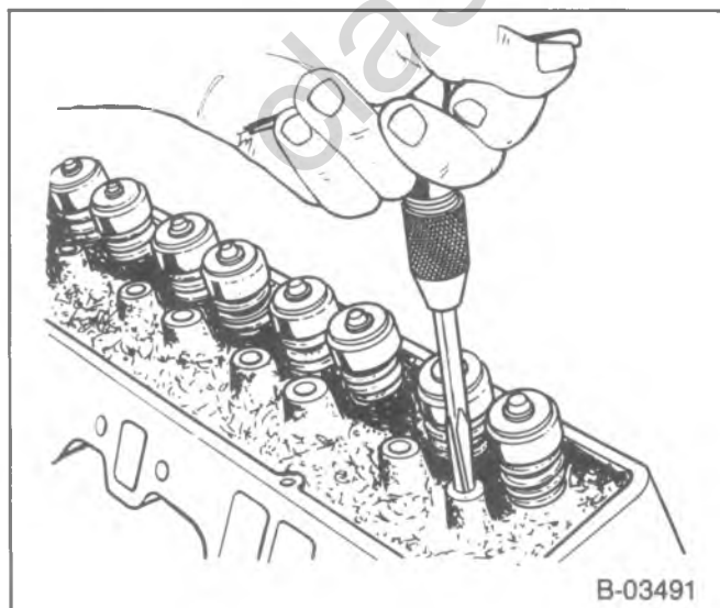
Figure 12—Reaming the Rocker Arm Stud Bore (Typical)
