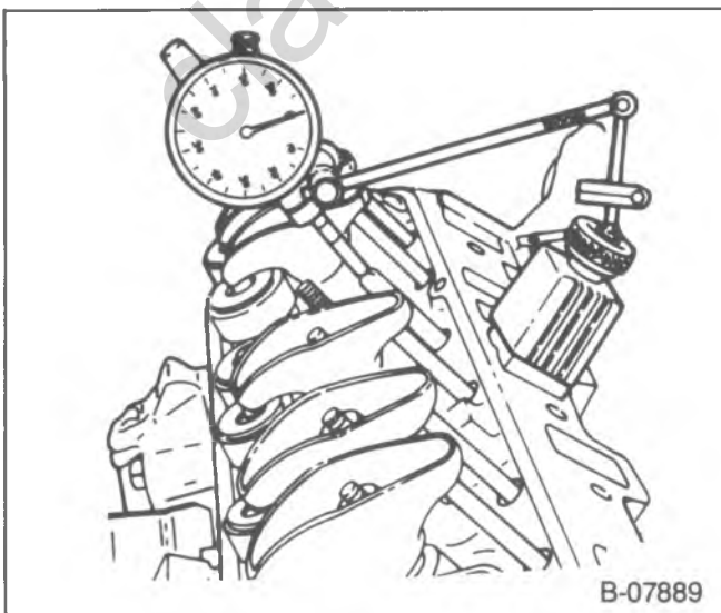
Figure 24—Measuring Camshaft Lobe Lift
