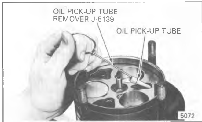
Fig. 1D-28 Removing A-6 Oil Pick-Up Tube
