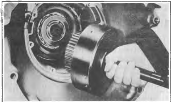
Figure 400-41 Removing Forward Clutch Assembly
