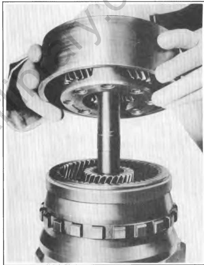
Figure 400-93 Installing Reaction Carrier to Output Carrier
