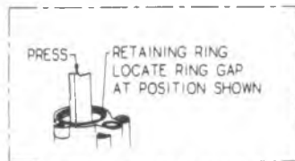
POSITIONING OF RETAINING RING.
