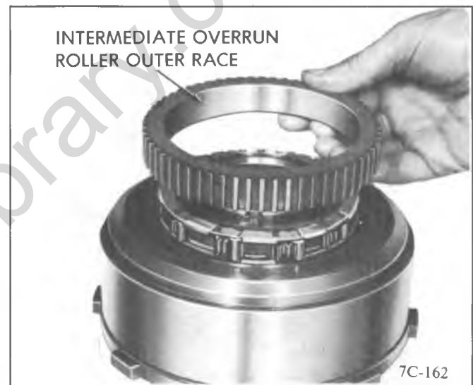
Figure 350C-77 Roller Clutch Outer Race
