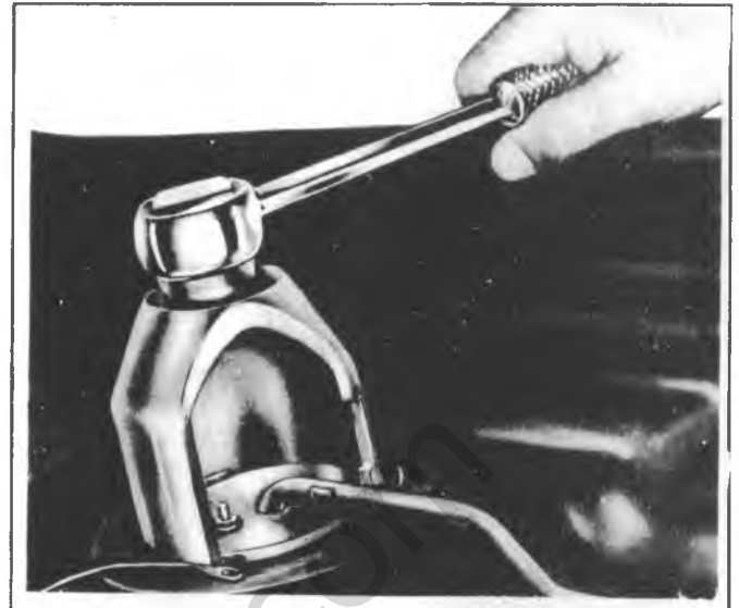
Fig. 6C-20--Removing Meter Assembly
