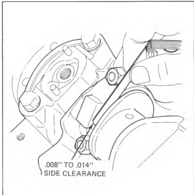
Fig. 45--Measuring Connecting Rod Side Clearance
