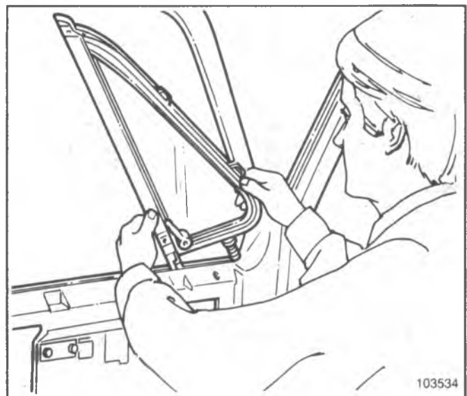
Fig. 2D-29--Removing Ventilator Assembly
