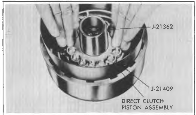
Figure 400-73 Installing Direct Clutch Piston
