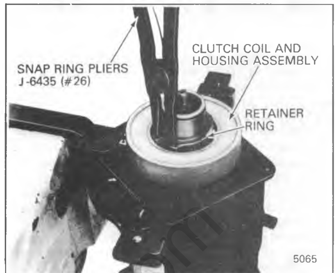
Fig. 1D-15 Removing A-6 Coil Housing Retainer Ring
