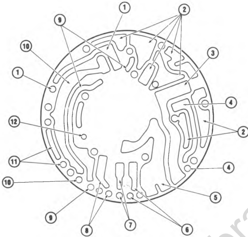
IDENTIFICATION OF OIL CHANNELS IN PUMP COVER
