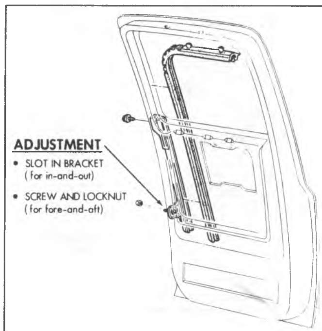
Fig. 2D-45--Glass Run Channel Adjustment
