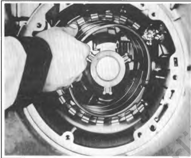
Figure 400-102 Installing Rear Band Assembly
