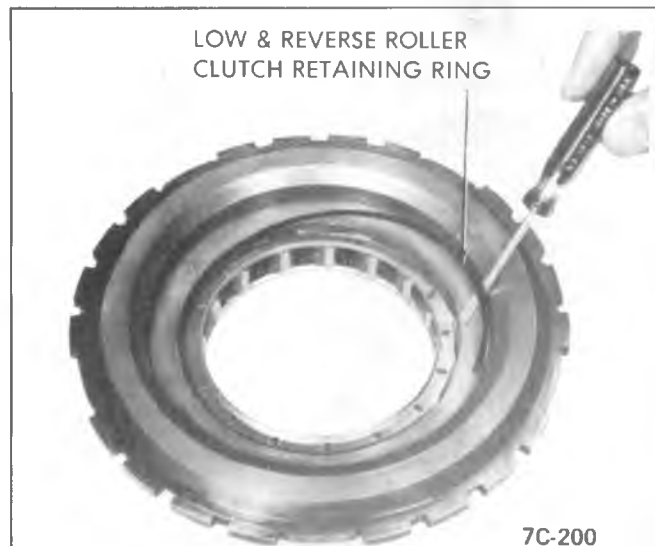
Figure 350C-108 Install Roller Clutch Retaining Ring
