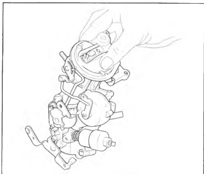
Fig. 6C1-27--Installing Air Horn
