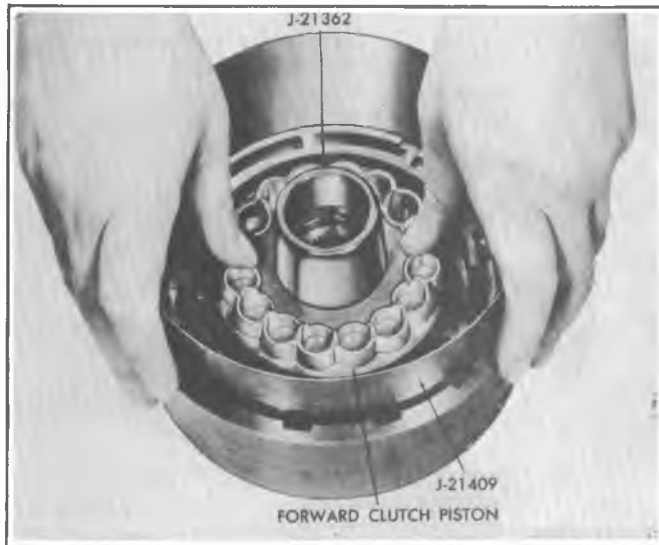
Figure 400-67 Installing Forward Clutch Piston
