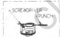
REMOVE RETAINING RING
