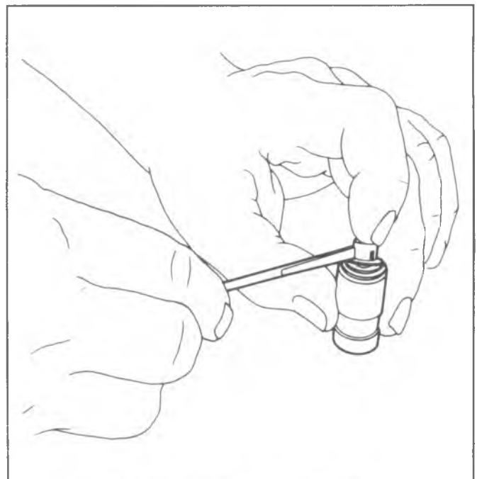
Fig. 18--Removing Ball Check Valve
