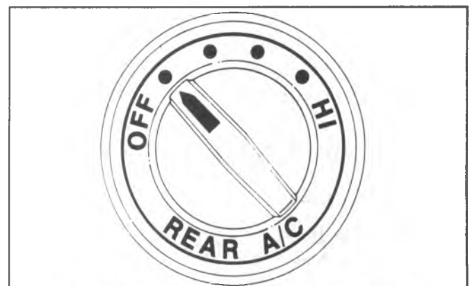
Fig. 1B-41--Blower Switch (C-K Overhead System)
