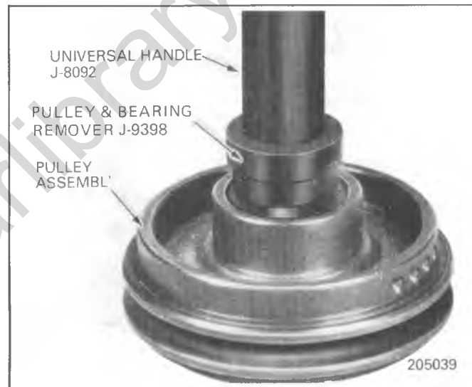
Fig. 1D-13 Removing Bearing From A-6 Pulley Asm.
