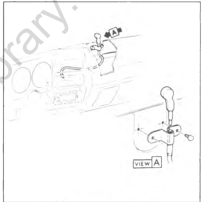
Fig. 9-16R--Antenna Lead (C-K Models)
