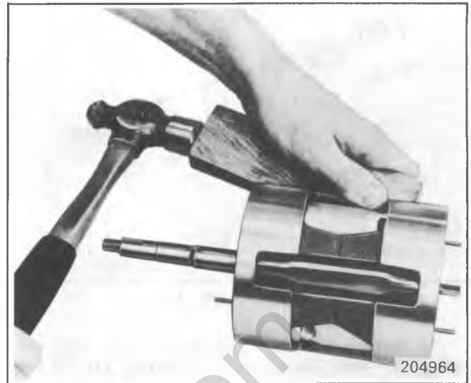
Fig. 1D-31 Separating A-6 Cylinder Halves
