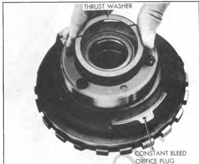
Figure 400-47 Removing Center Support to Reaction Carrier Thrust Washer
