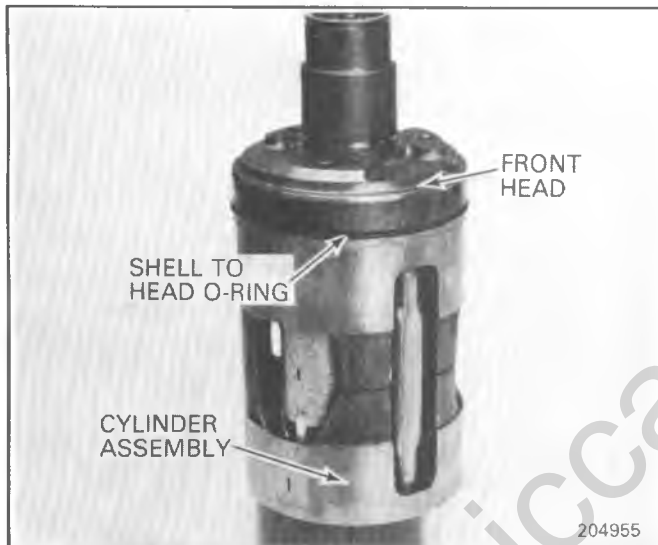
Fig. 1D-66 A-6 Shell-To-Front Head O-Ring Installation
