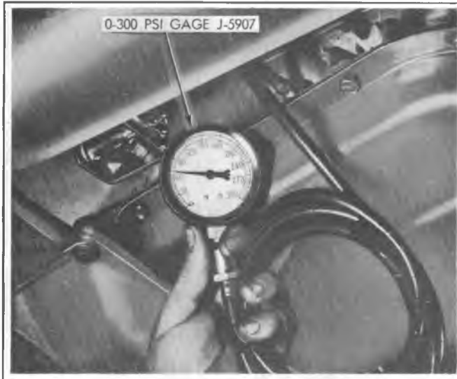
Figure 400-6 Oil Pressure Test Gage
