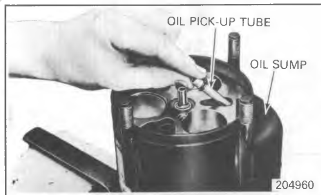
Fig. 1D-64 Installing A-6 Oil Pick-up Tube
