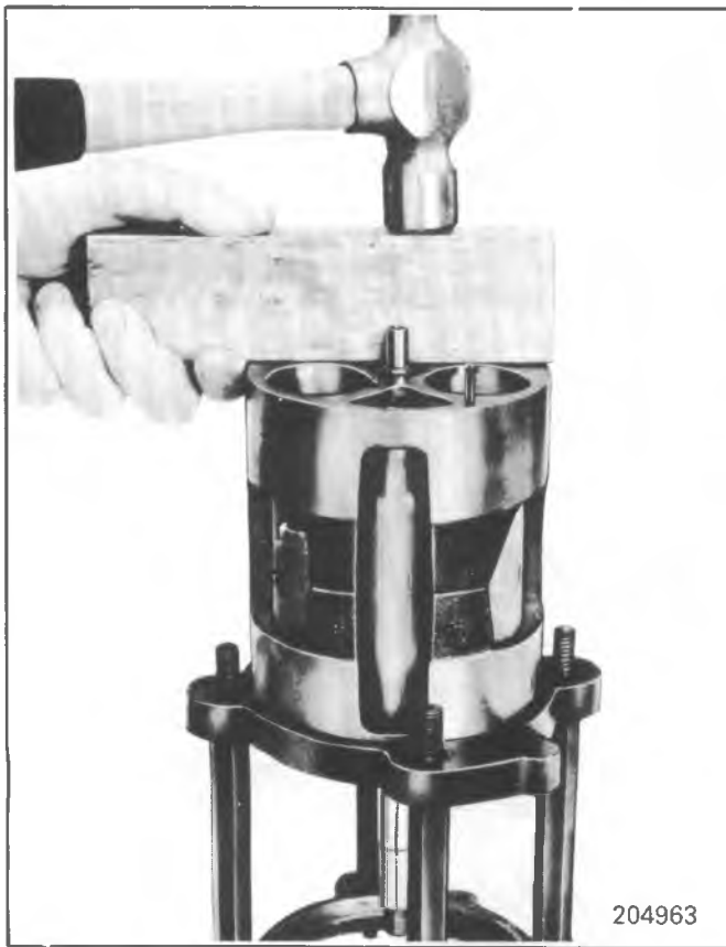
Fig. 1D-39 Assembling A-6 Cylinder Halves
