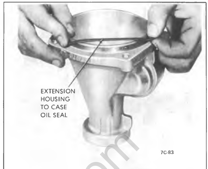
Figure 350C-33 Extension Housing Square Cut Oil Seal
