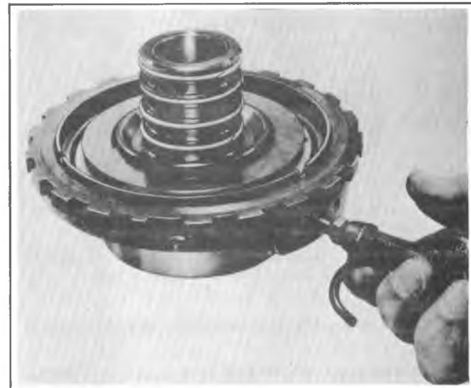
Figure400-83 Air Checking Intermediate Clutch
