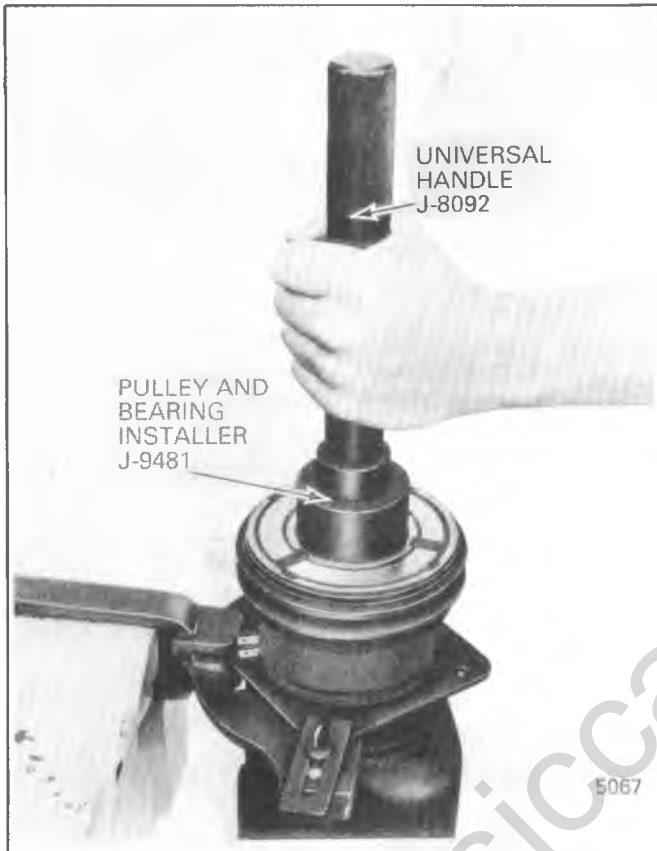
Fig. 1D-11 Installing A-6 Pulley and Bearing Asm.
