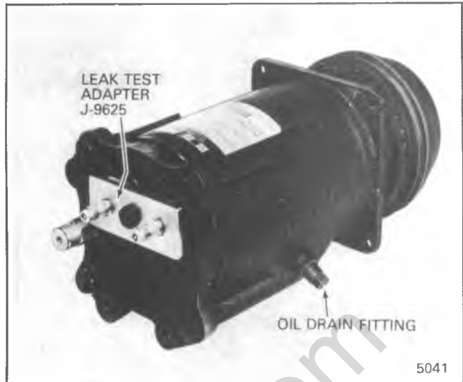
Fig. 1D-22 Leak Testing A-6 Compressor
