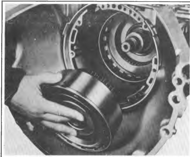
Figure 400-42 Removing Direct Clutch and Intermediate Roller Assembly
