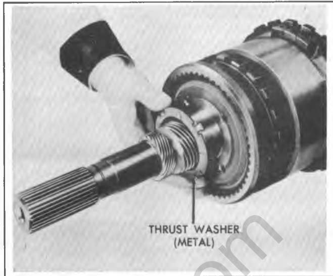
Figure 400-92 Installing Case-to-Output Shaft Metal Thrust Washer
