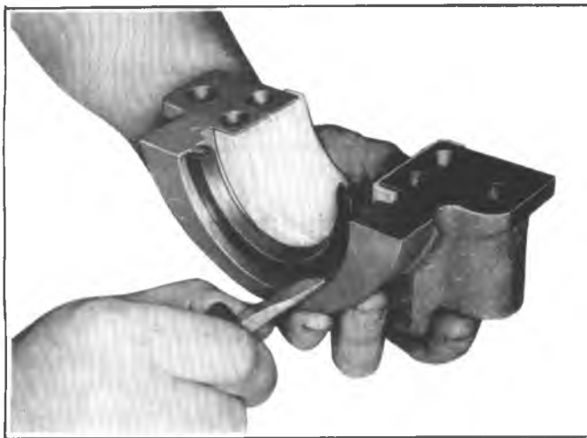
Fig. 6A4-47--Removing Oil Seal - Lower Half
