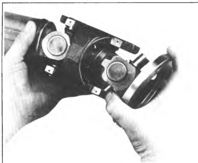
Fig. 4A-32—Reassembling Flange Yoke
