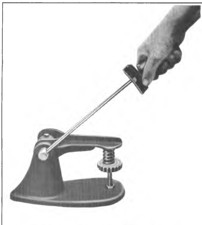
Fig. 6A5-22--Checking Valve Spring Tension
