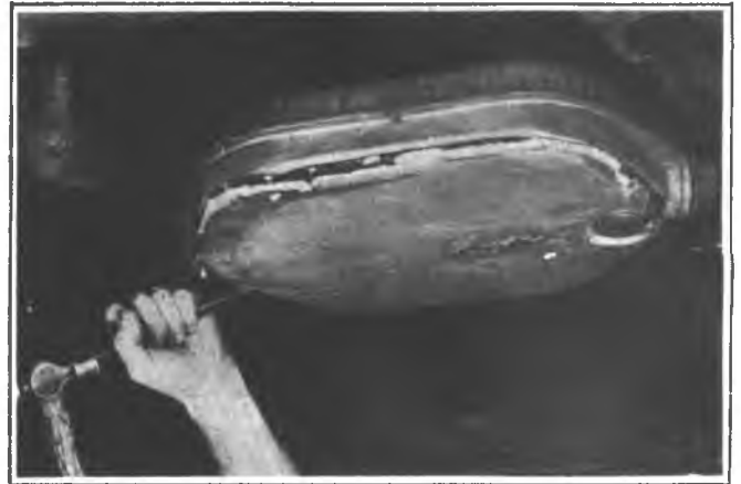
Fig. 6F-11 — Removing Bottom Cover
