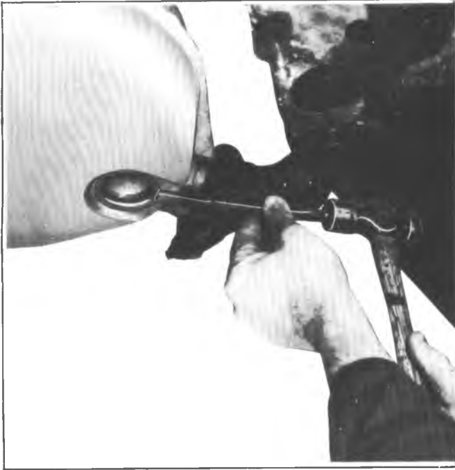
Fig. 6F-5 — Removing Pressed Plug
