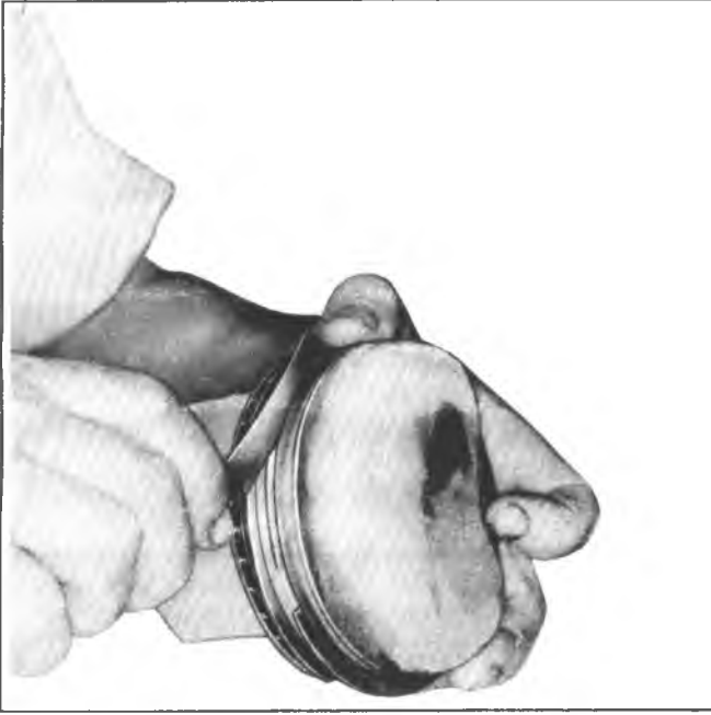
Fig. 6A5-57—Measuring Ring Groove Clearance
