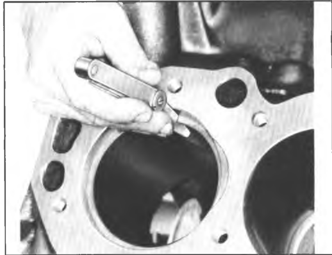
Fig. 6A4-54--Measuring Ring Gap
