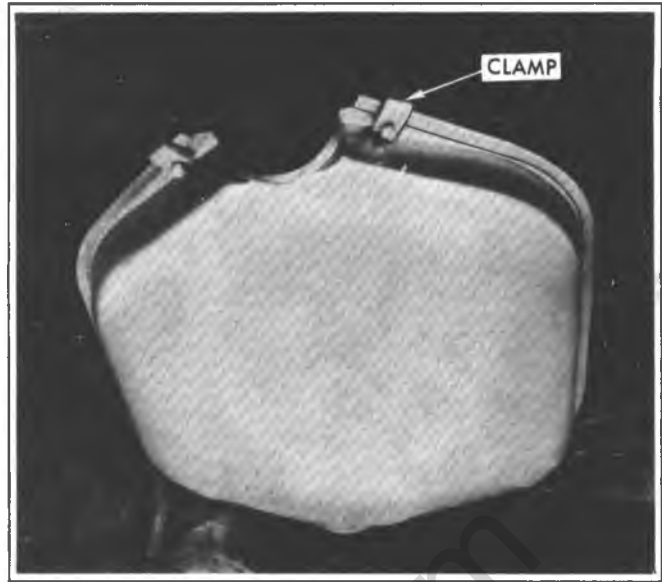
Fig. 6F-16 — Installing Bottom Cover Clamps
