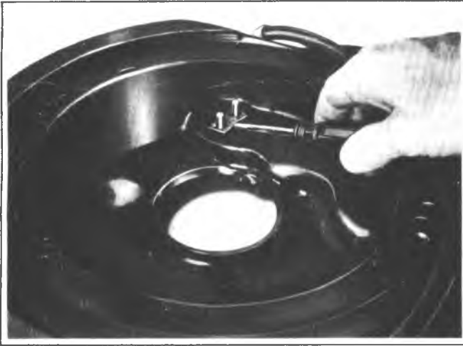
Fig. 6E-23-Removing Sensor Unit
