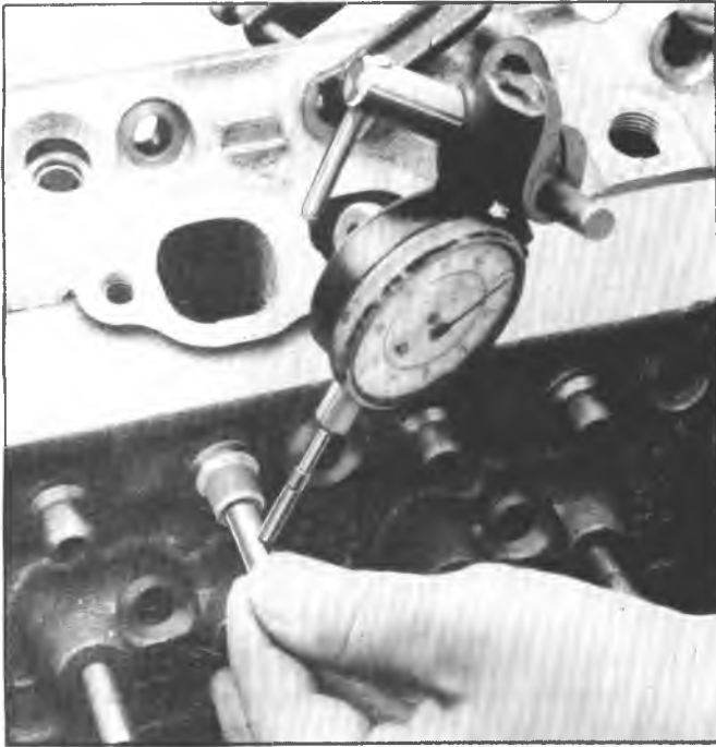
Fig. 6A4-20--Measuring Valve Stem Clearances
