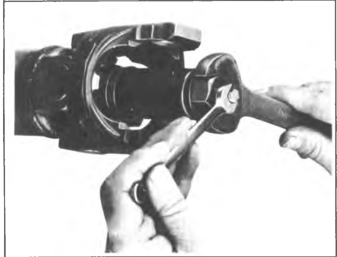
Fig. 4A-29--Removing Centering Ball
