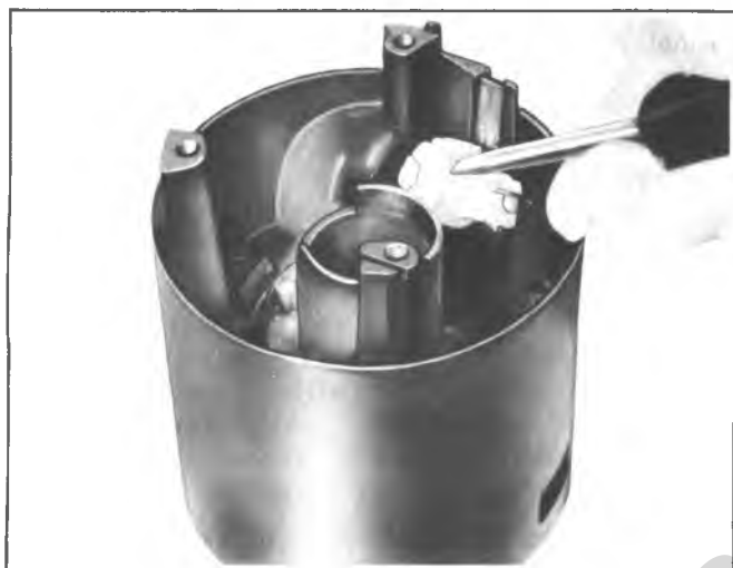
Fig. 3B4-44--Removing Ignition Switch Actuator Sector
