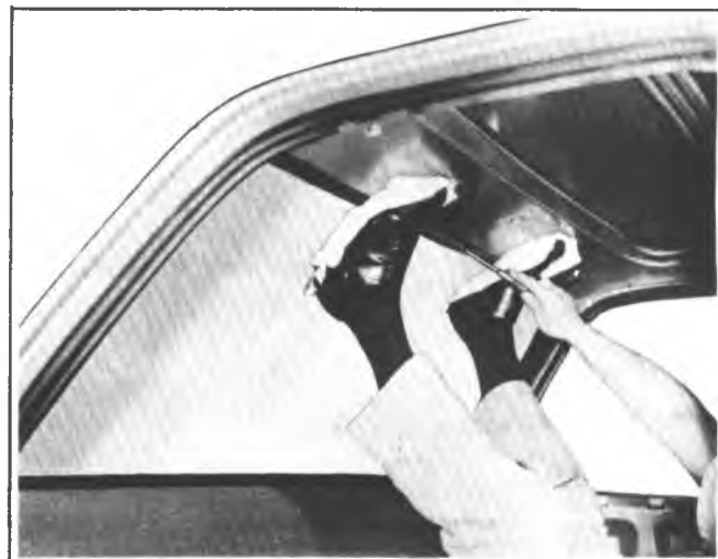
Fig. 2D-14--Applying Pressure to Windshield
