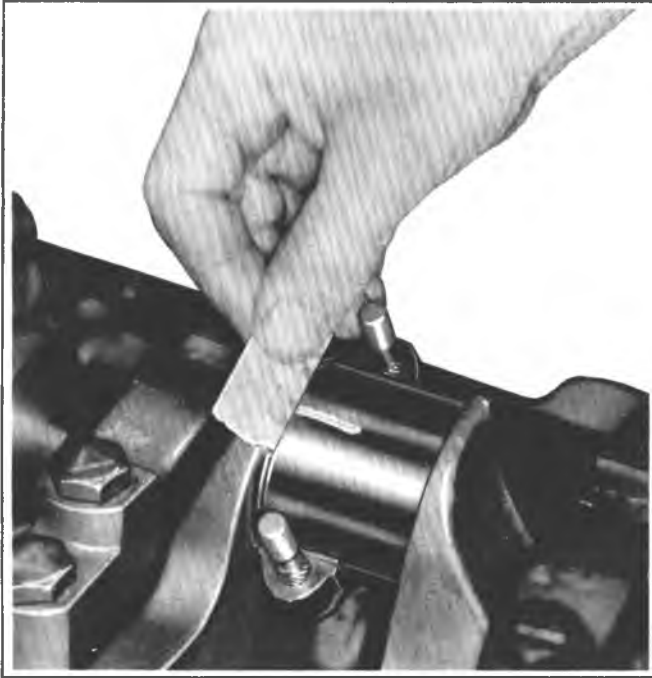
Fig. 6A1-28—Measuring Gaging Plastic
