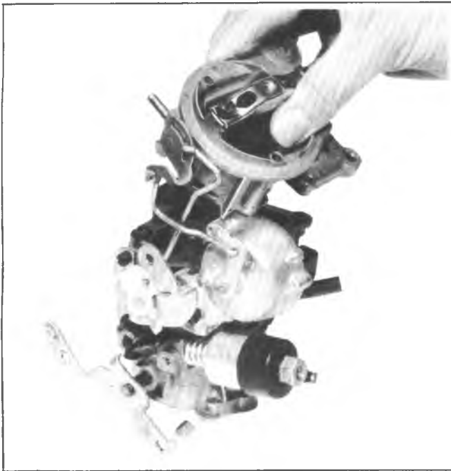
Fig. 6C1-15--Air Horn Removal
