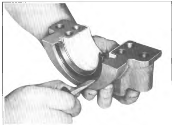
Fig. 6A5-48--Removing Oil Seal - Lower Half
