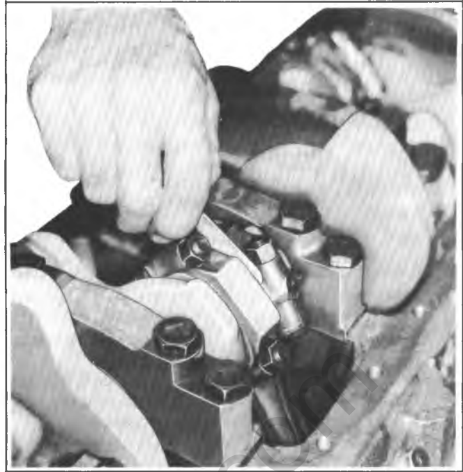
Fig. 6A5-43--Measuring Connecting Rod Side Clearance
