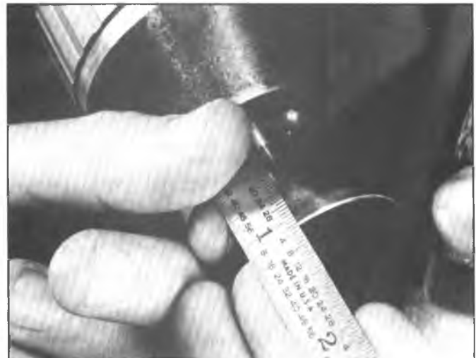
Fig. 6A5-29--Measuring Valve Head
