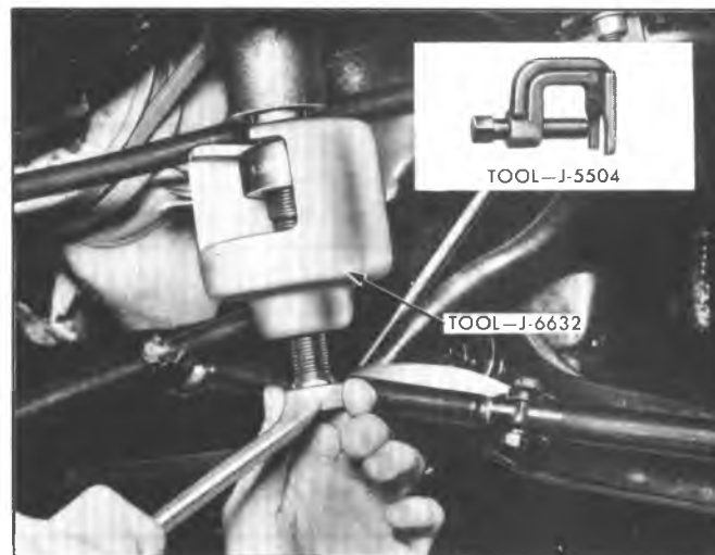
Fig. 3B3-13--Removing Pitman Arm
