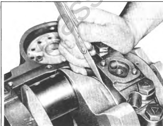
Fig. 6A4-45--Measuring Crankshaft End Play
