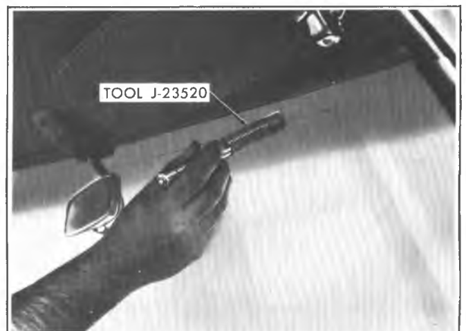
Fig. 9-4R--Testing Windshield Antenna (Typical)
