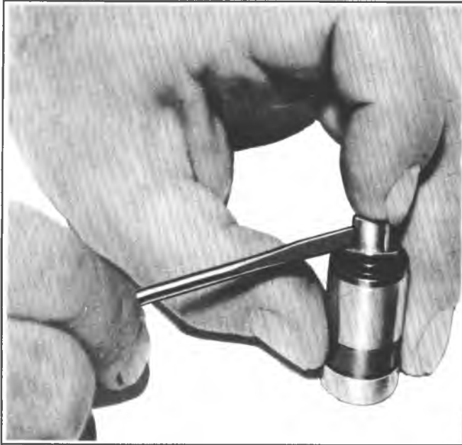
Fig. 6A1-13--Removing Ball Check Valve
