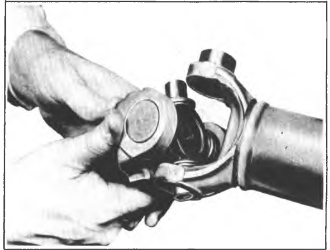
Fig. 4A-14--Installing Trunnion into Yoke
