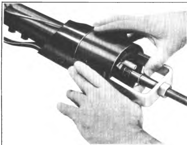
Fig. 3B4-30--Installing Snap Ring
