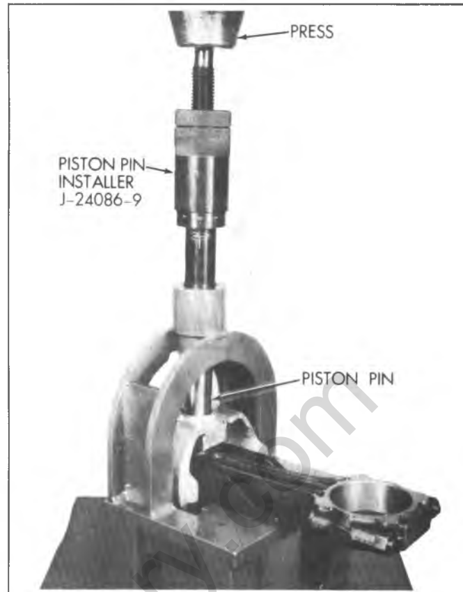
Fig. 6A5-53--Installing Piston Pin
