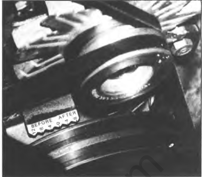
Fig. 6D-26D—Timing Mark - Typical
