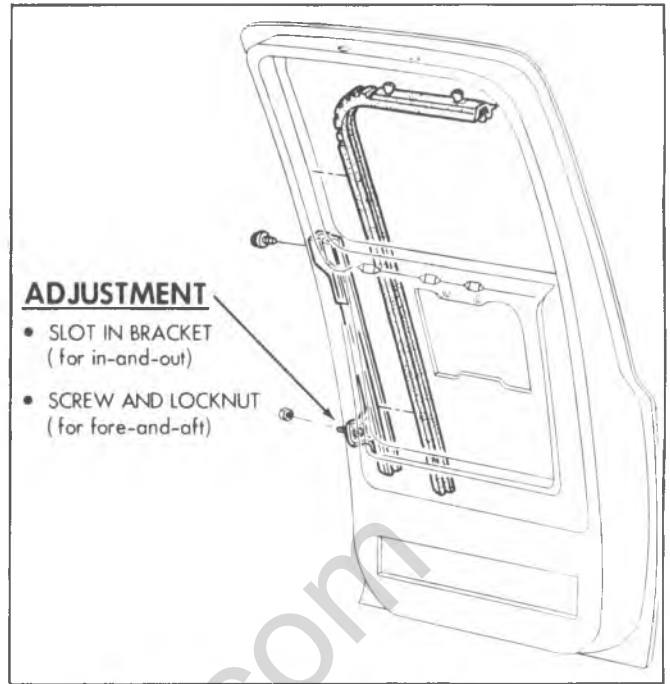
Fig. 2D-45--Glass Run Channel Adjustment
