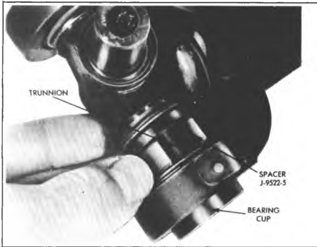
Fig. 4A-12--Using Spacer to Remove Bearing Cup
