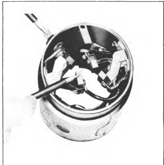
Fig. 6D-13E--Testing Field Coils for Open
