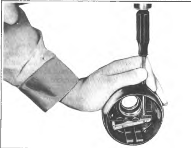
Fig. 3B4-80--Removing Release Lever Pivot Pin
