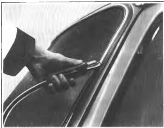
Fig. 2D-19--Installing Reveal Molding
