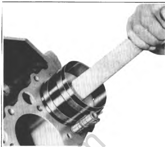
Fig. 6A1-45—Installing Connecting Rod and Piston Assembly
