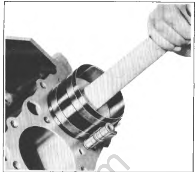
Fig. 6A4-58--Installing Connecting Rod &amp; Piston Assembly
