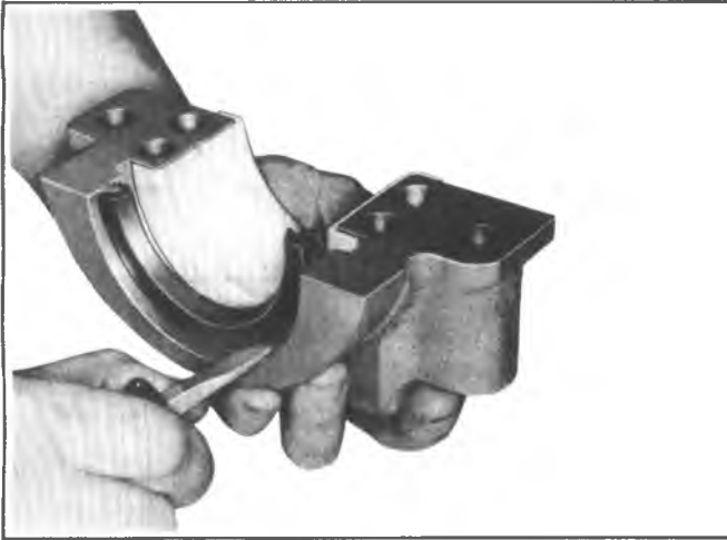
Fig. 6A1-35--Removing Oil Seal Lower Half - Typical
