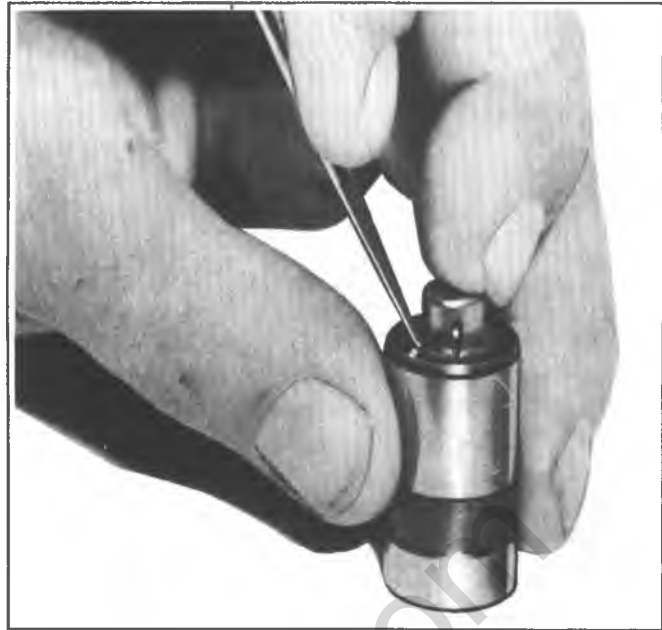
Fig. 6A4-16-Installing Ball Check Valve
