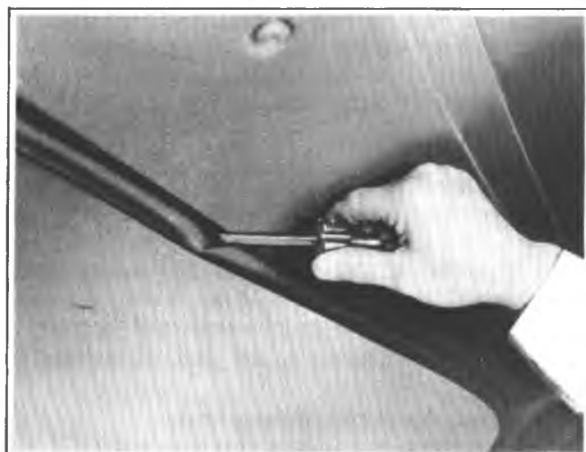
Fig. 2D-15--Assisting Weatherstrip over Flange
