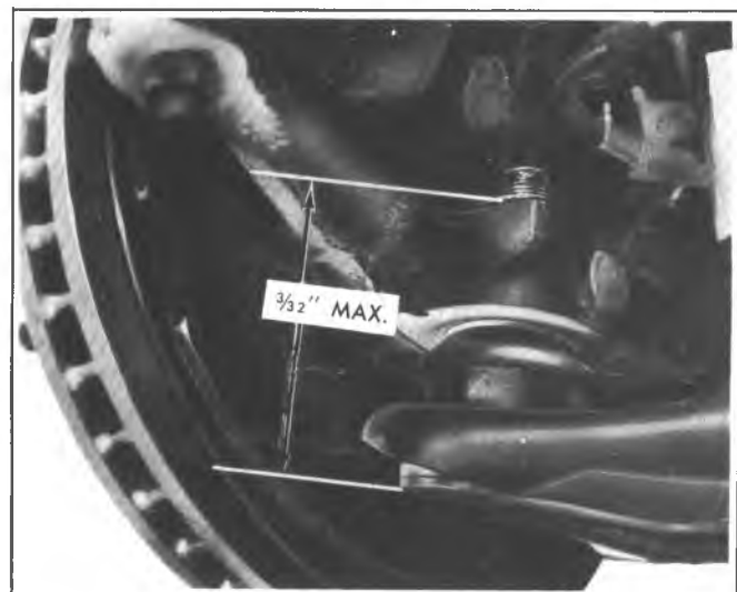
Fig. 3C-29—Checking Lower Ball Joint
