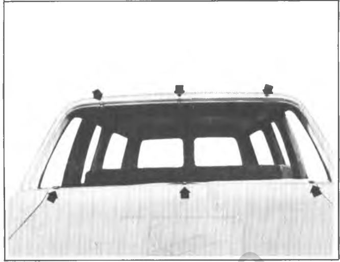
Fig. 2D-17--Checking Windshield Opening
