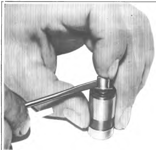
Fig. 6A5-15--Removing Ball Check Valve
