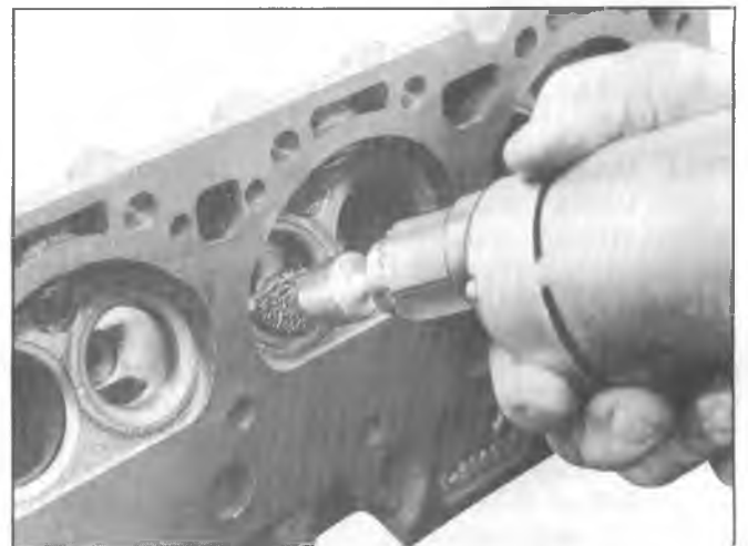
Fig. 6A4-19--Cleaning Combustion Chambers
