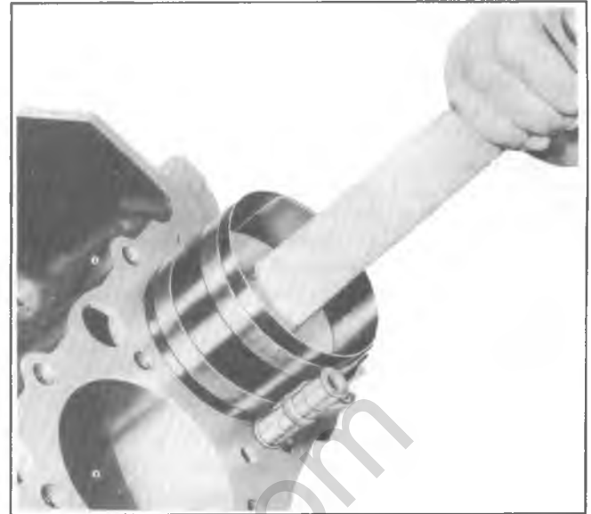
Fig. 6A4-58--Installing Connecting Rod &amp; Piston Assembly
