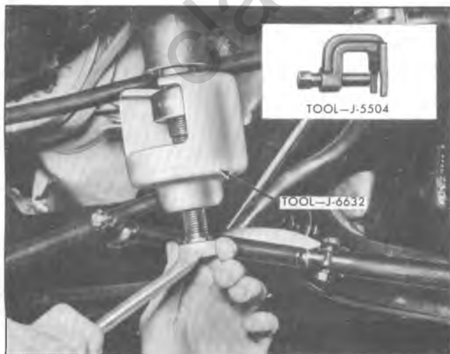
Fig. 3B2-4--Removing Pitman Arm
