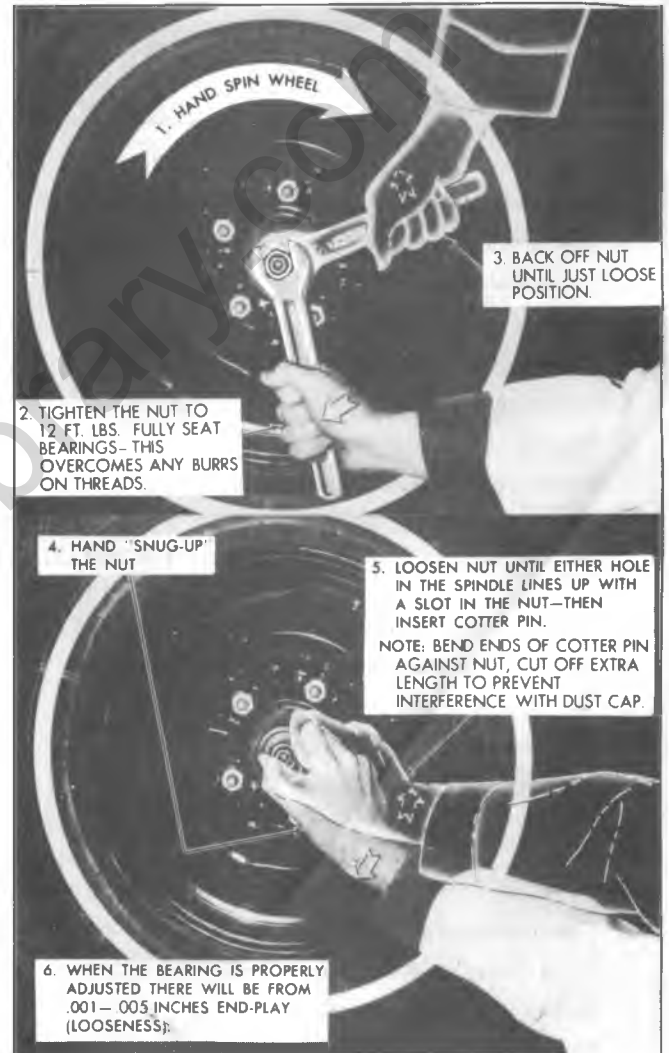
Fig. 3C-3—Wheel Bearing Adjustment
