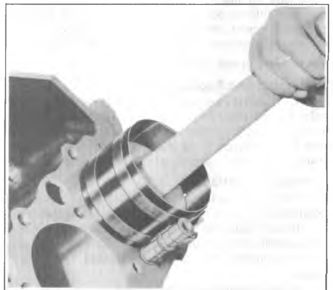
Fig. 6A1-45--Installing Connecting Rod and Piston Assembly
