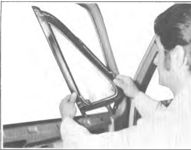
Fig. 2D-29--Removing Ventilator Assembly
