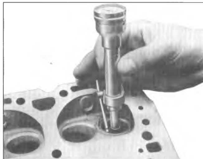
Fig. 6A4-29--Measuring Valve Seat Concentricity
