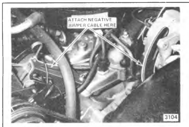
Fig. 6D-6B—Negative Jumper Cable Connection
