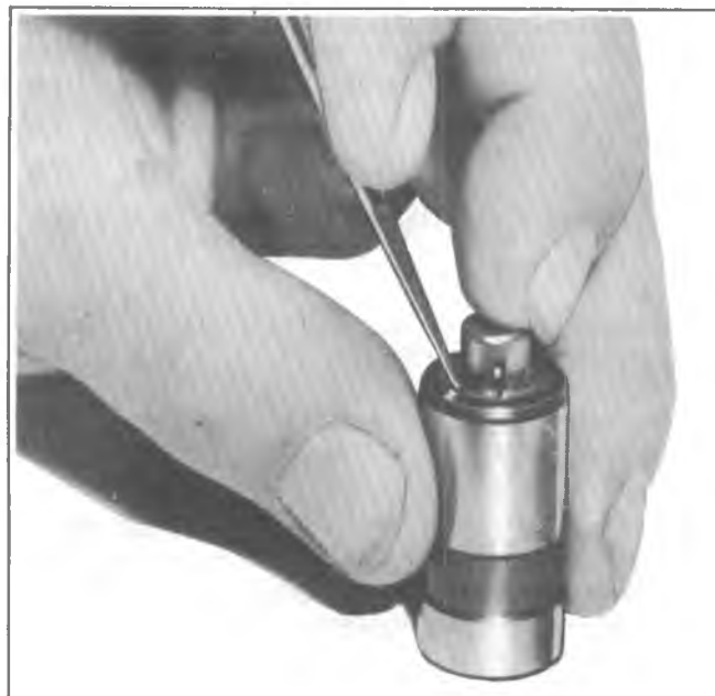
Fig. 6A4-16--Installing Ball Check Valve
