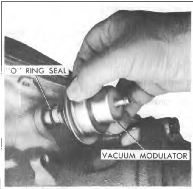
Fig. 7A-19--Removing Vacuum Modulator
