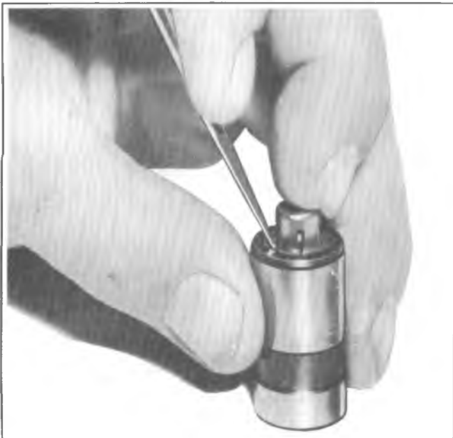
Fig. 6A1-14--Installing Ball Check Valve
