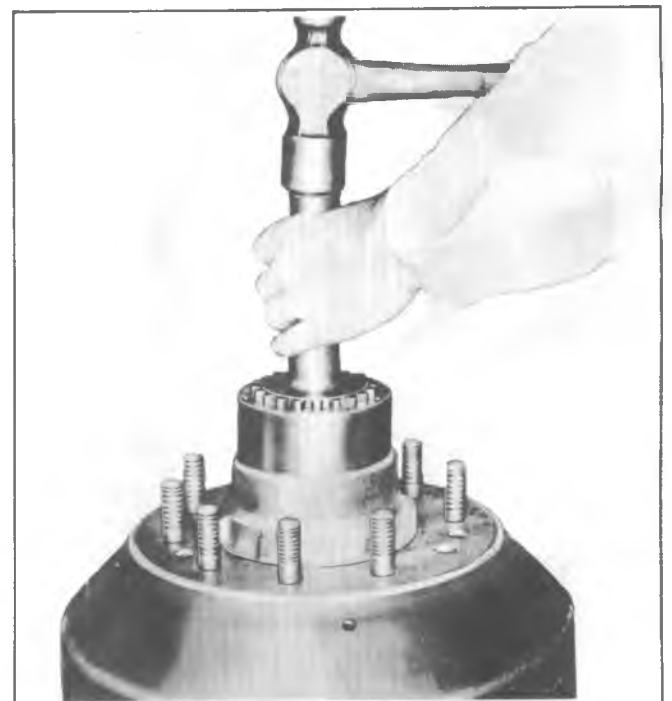
Fig. 4B-38--Removing Hub Outer Bearing
