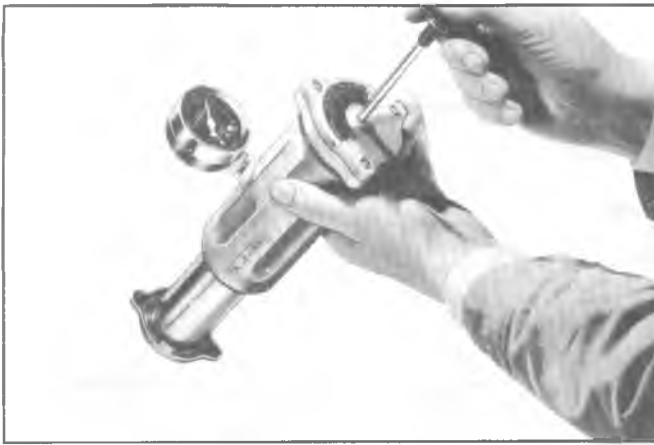
Fig. 6B-5--Pressure Checking Radiator Cap
