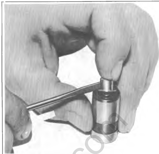
Fig. 6A4-15--Removing Ball Check Valve
