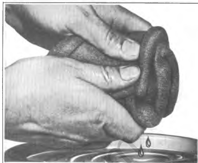
Fig. 6E-14-Cleaning Polywrap Band
