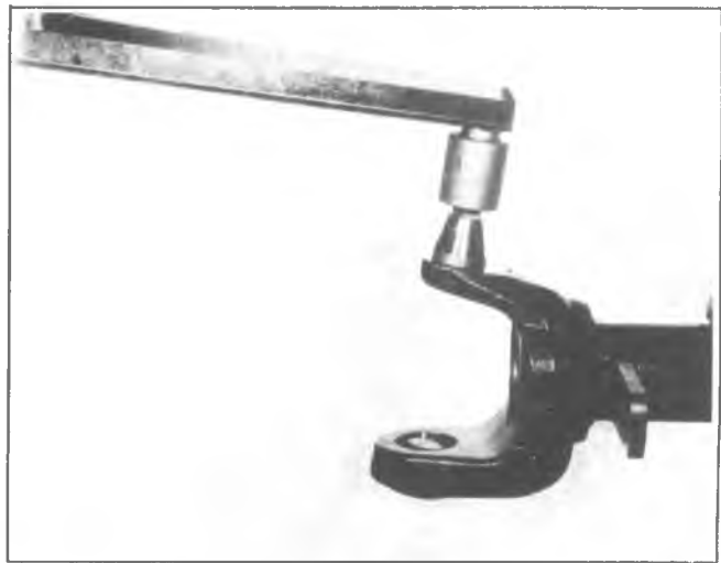
Fig. 3C-28K--Installing Upper King-Pin
