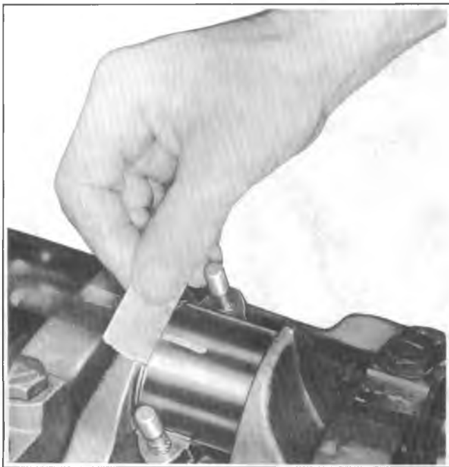
Fig. 6A5-42--Measuring Gaging Plastic
