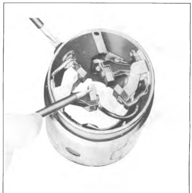
Fig. 6D-13E--Testing Field Coils for Open
