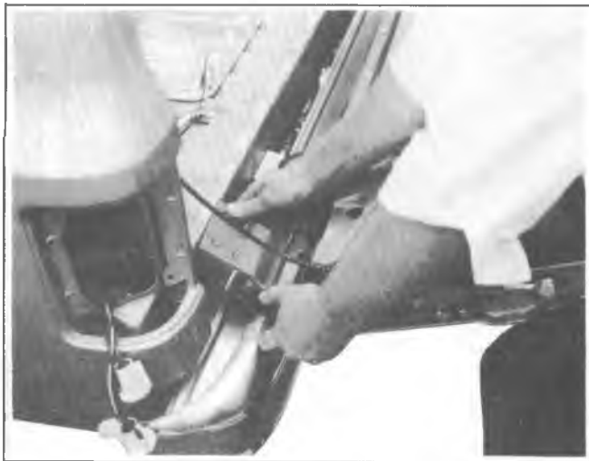
Fig. 2D-63--Pulling Hinge Away From Body (16)
