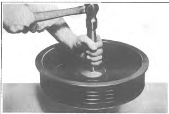
Fig. 4B-39--Installing Hub Inner Bearing Cup
