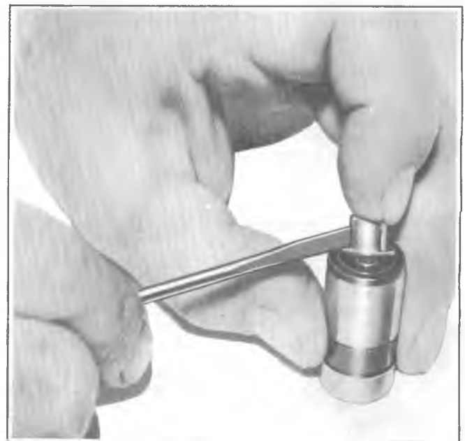
Fig. 6A1-13--Removing Ball Check Valve
