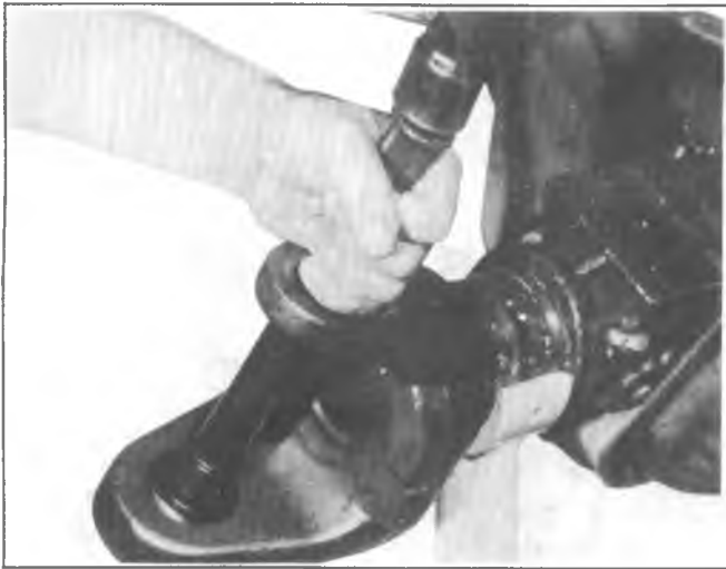
Fig. 3C-25K--Removing Cup, Cone and Seal
