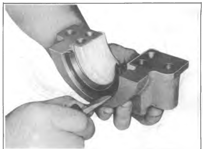
Fig. 6A4-47--Removing Oil Seal - Lower Half
