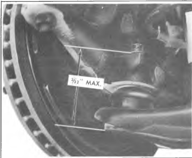
Fig. 3C-29—Checking Lower Ball Joint
