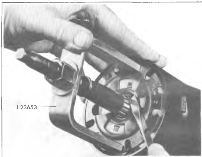
Fig. 3B4-26--Removing Lock Plate Retaining Ring
