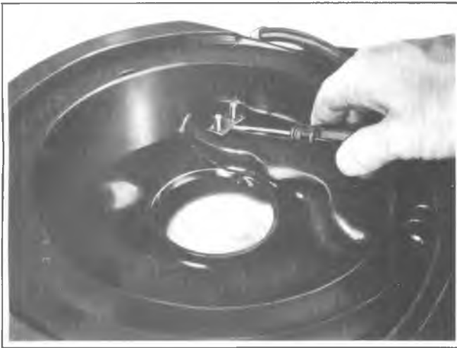
Fig. 6E-23-Removing Sensor Unit
