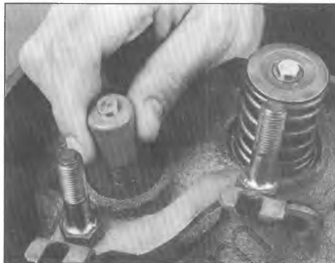
Fig. 6A5-13--Installing Valve Stem Oil Seal
