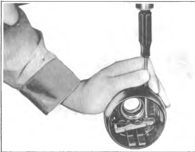
Fig. 3B4-80--Removing Release Lever Pivot Pin
