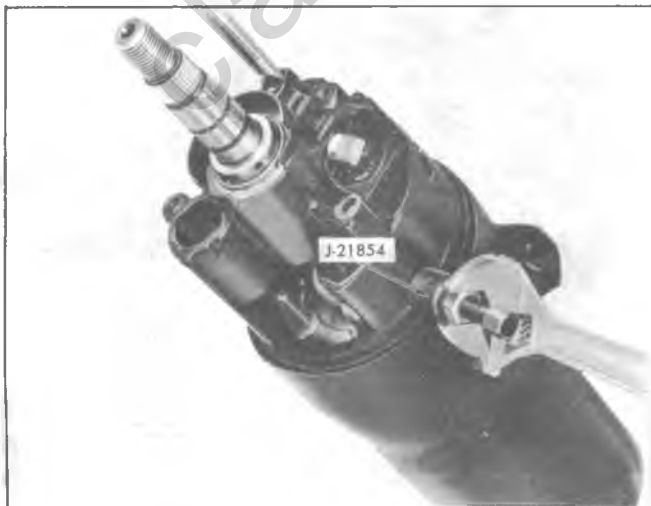
Fig. 3B4-51--Removing Bearing Housing Pivot Pins
