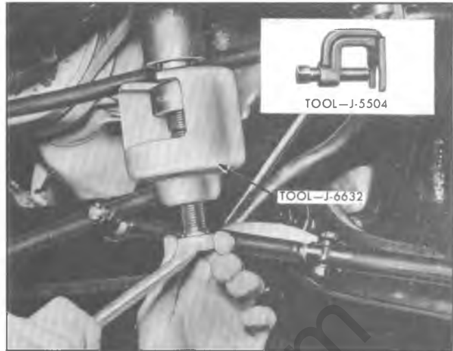
Fig. 3B2-9--Removing Pitman Arm-Typical
