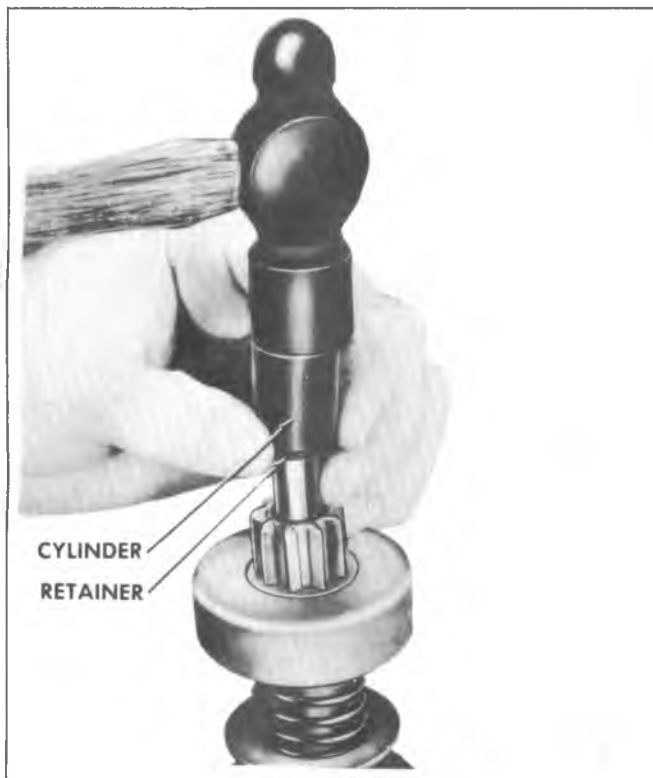
Fig. 6D-10E--Removing Retainer From Snap Ring
