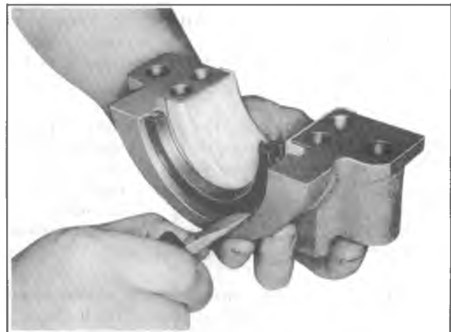
Fig. 6A5-48--Removing Oil Seal - Lower Half
