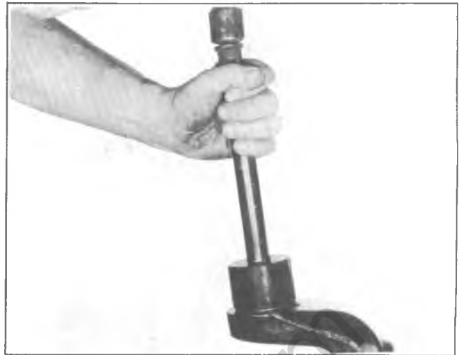
Fig. 3C-27K--Installing Oil Seal
