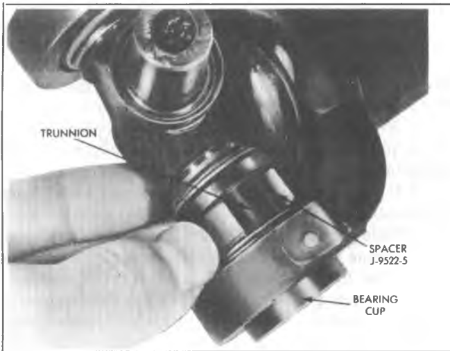
Fig. 4A-12--Using Spacer to Remove Bearing Cup
