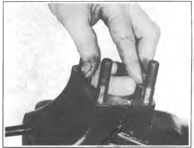
Fig. 3C-23K--Removing Tapered Bushing
