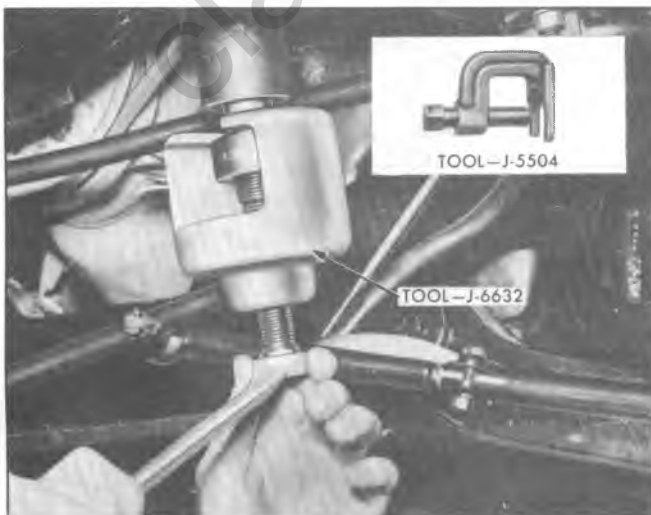
Fig. 3B3-13--Removing Pitman Arm
