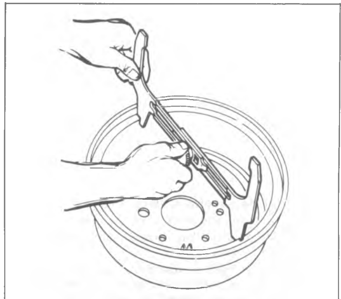
Fig. 5-45—Measuring Brake Drum I.D.
