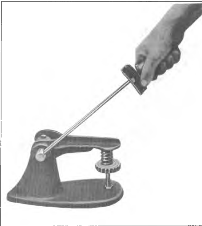
Fig. 6A1-16--Checking Valve Spring Tension
