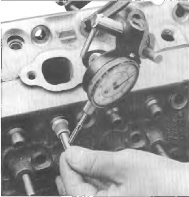
Fig. 6A4-20—Measuring Valve Stem Clearances
