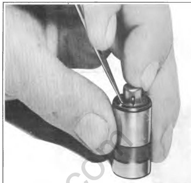
Fig. 6A5-16--Installing Ball Check Valve
