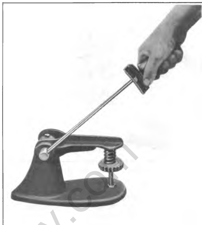
Fig. 6A5-22--Checking Valve Spring Tension
