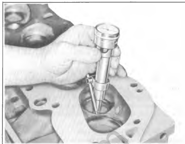
Fig. 6A5-28--Measuring Valve Seat Concentricity
