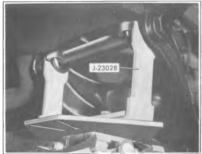
Fig. 3C-17--Removing Coil Spring with Tool J-23028
