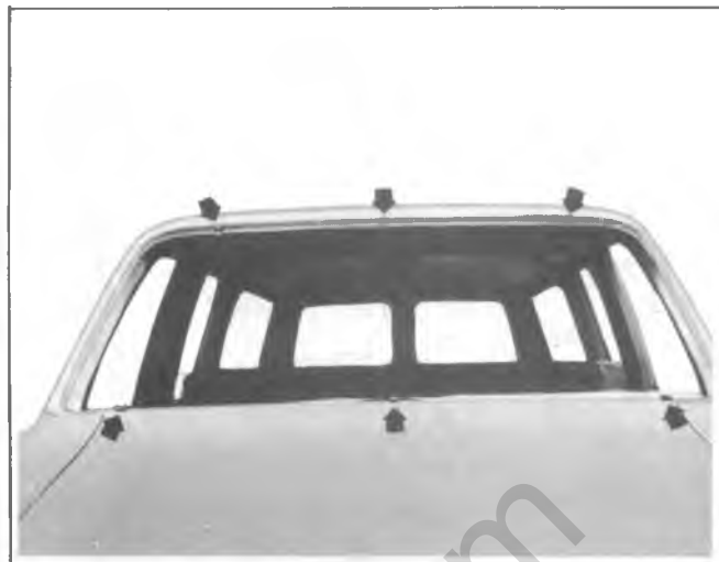
Fig. 2D-17--Checking Windshield Opening
