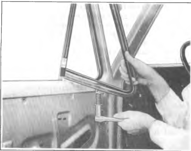
Fig. 2D-111--Adjusting Ventilator Tension
