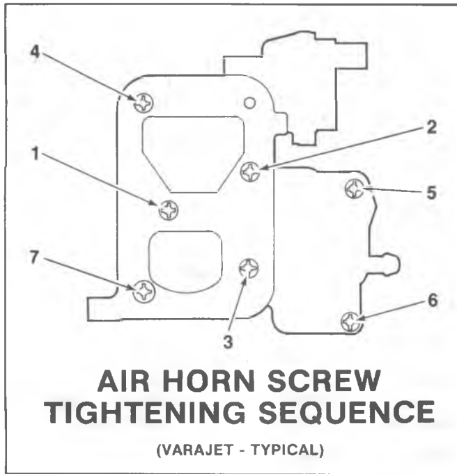
Fig. 6C2-39—Air Horn Tightening Sequence
