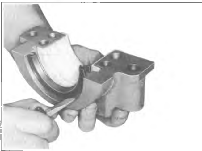
Fig. 6A1-35--Removing Oil Seal Lower Half - Typical
