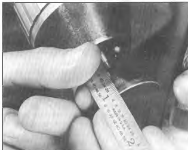
Fig. 6A5-29--Measuring Valve Head
