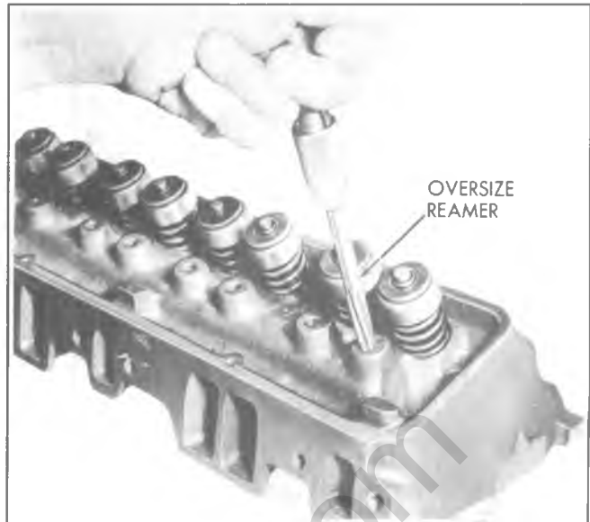
Fig. 6A1-19--Reaming Rocker Arm Stud Bore - Typical
