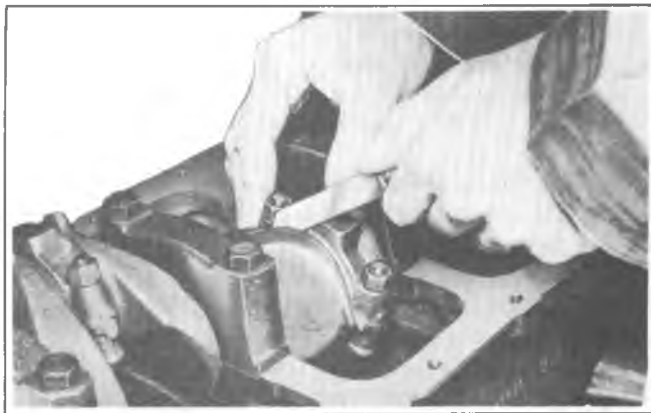
Fig 6A1-29--Measuring Connecting Rod Side Clearance
