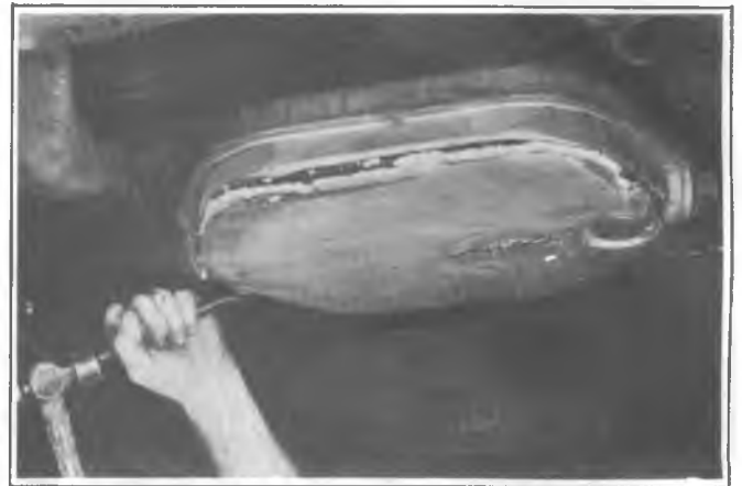
Fig. 6F-14--Removing Bottom Cover
