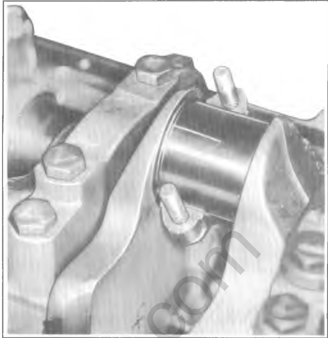
Fig. 6A1-27--Gaging Plastic on Crankpin
