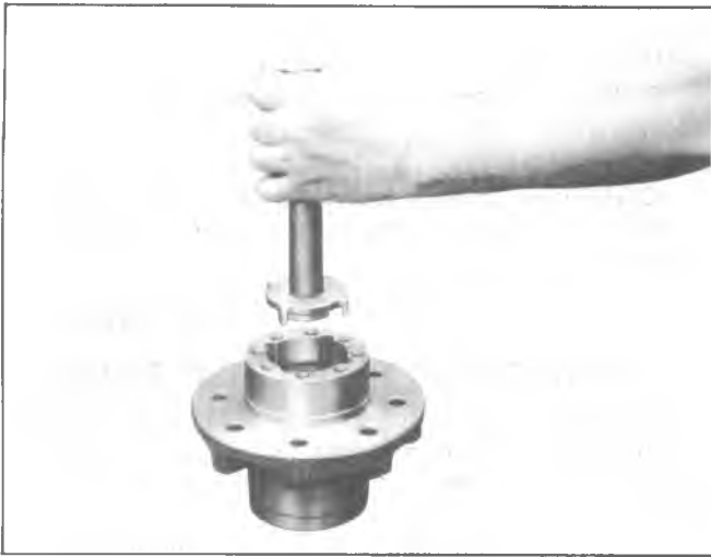
Fig. 4B-33--Removing Outer Bearing and Cup
