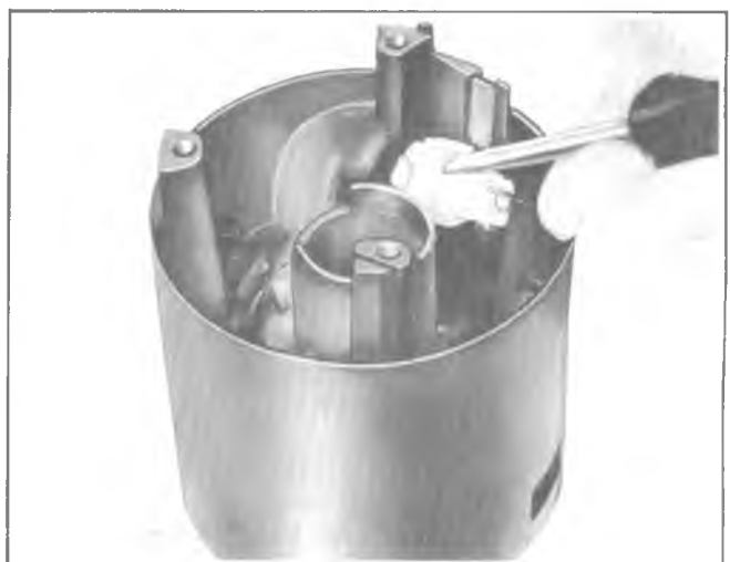
Fig. 3B4-44--Removing Ignition Switch Actuator Sector
