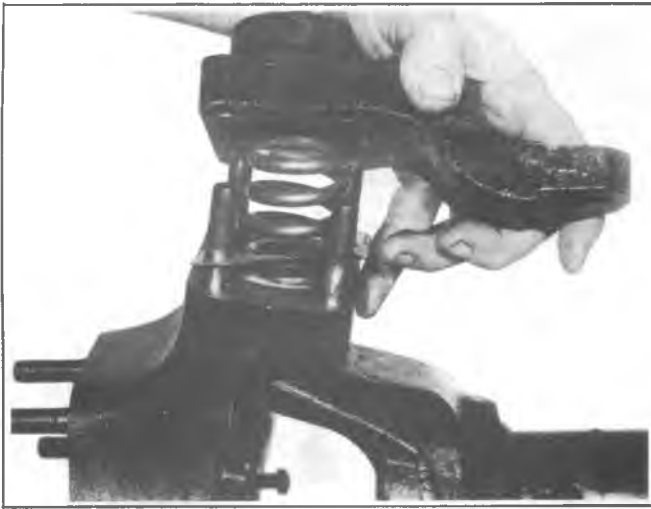
Fig. 3C-21K--Removing Cap, Spring and Gasket
