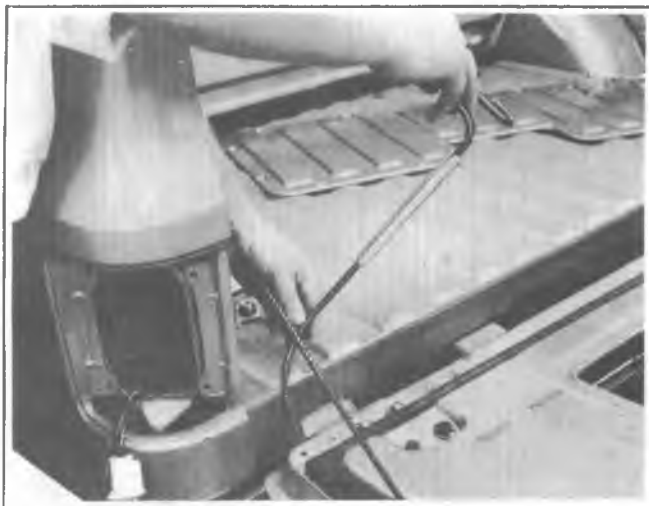
Fig. 2D-67--Removing Torque Rod (16)
