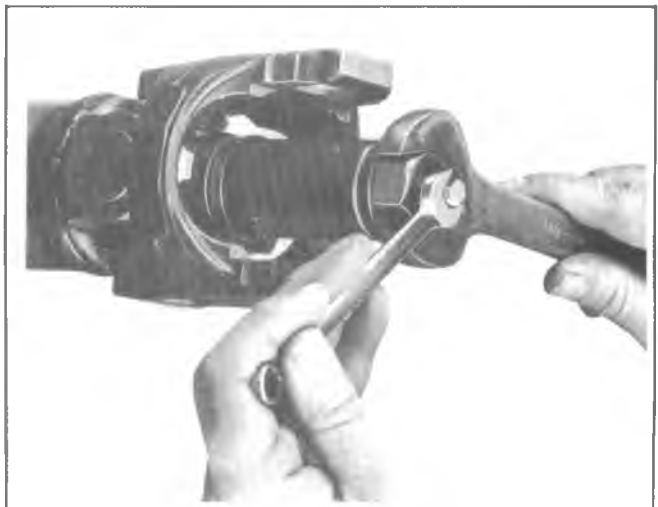
Fig. 4A-29--Removing Centering Ball
