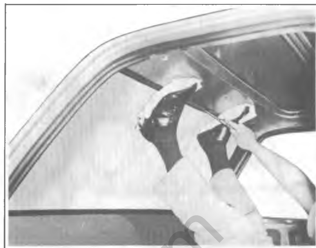
Fig. 2D-14--Applying Pressure to Windshield
