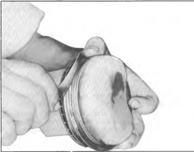
Fig. 6A4-57--Measuring Ring Groove Clearance
