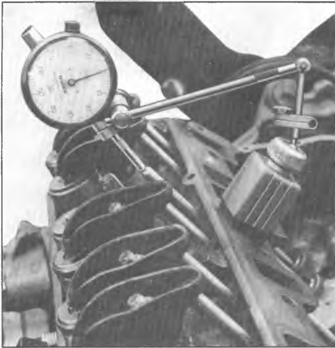
Fig. 6A4-33--Measuring Camshaft Lobe Lift
