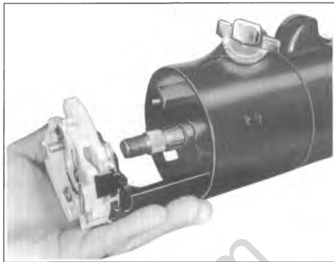
Fig. 3B4-28--Removing Directional Signal Switch Assembly
