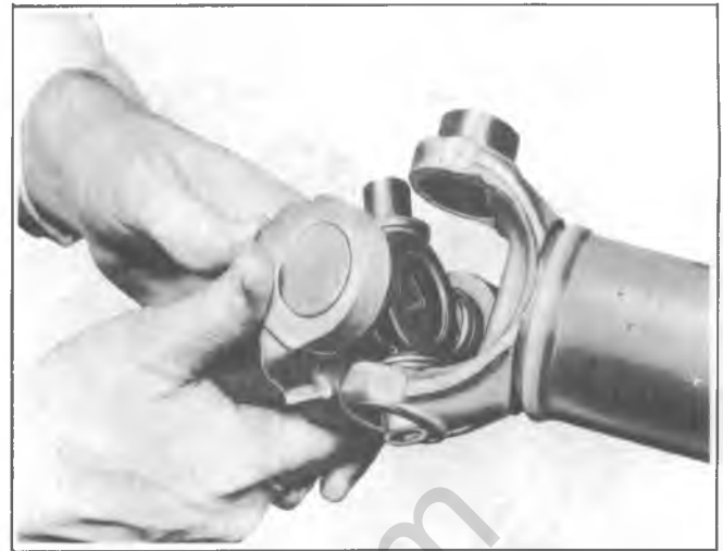
Fig. 4A-14--Installing Trunnion into Yoke
