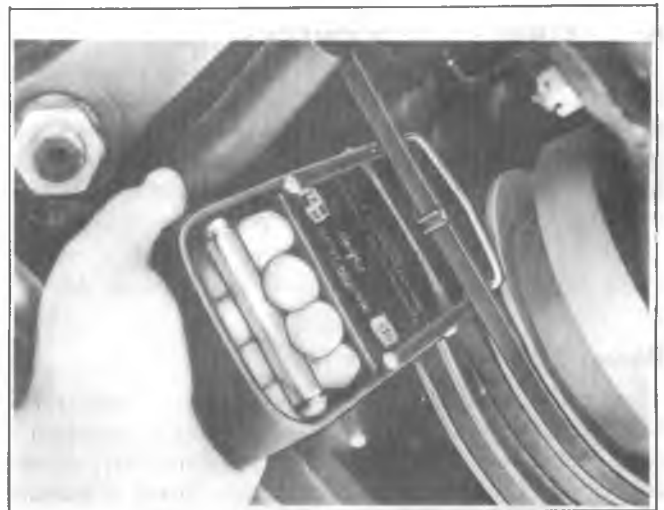
Fig. 3B3-11--Checking Belt Tension with J-23600
