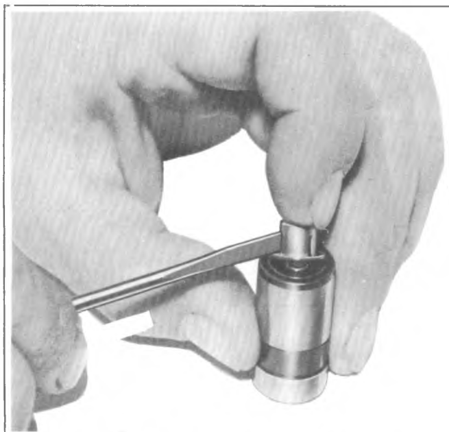
Fig. 6A2-18--Removing Ball Check Valve
