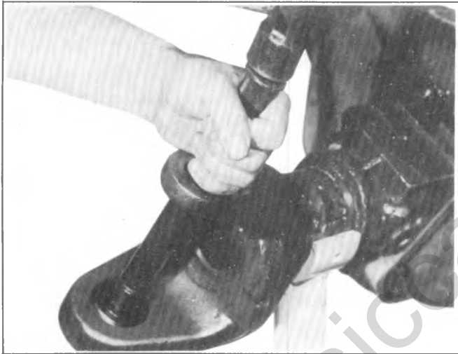
Fig. 3C-24K--Removing Cup, Cone and Seal
