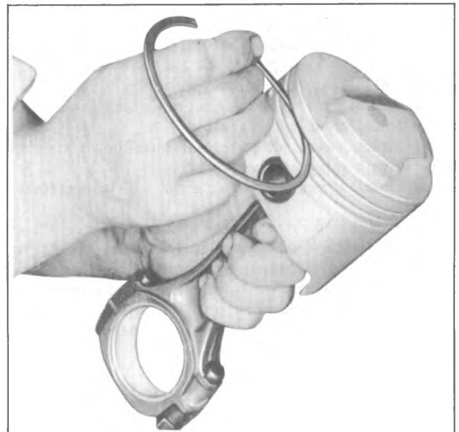
Fig. 6A2-69--Checking Ring in Groove
