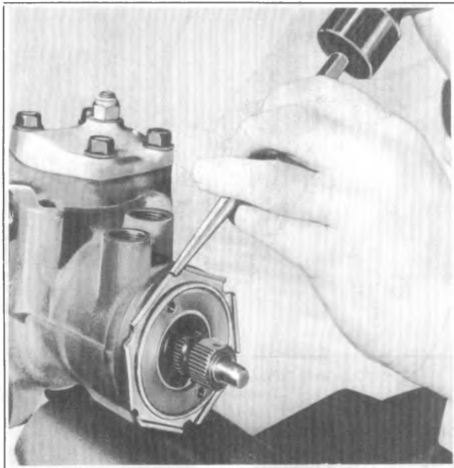
Fig. 3B-35--Loosening Lock Nut
