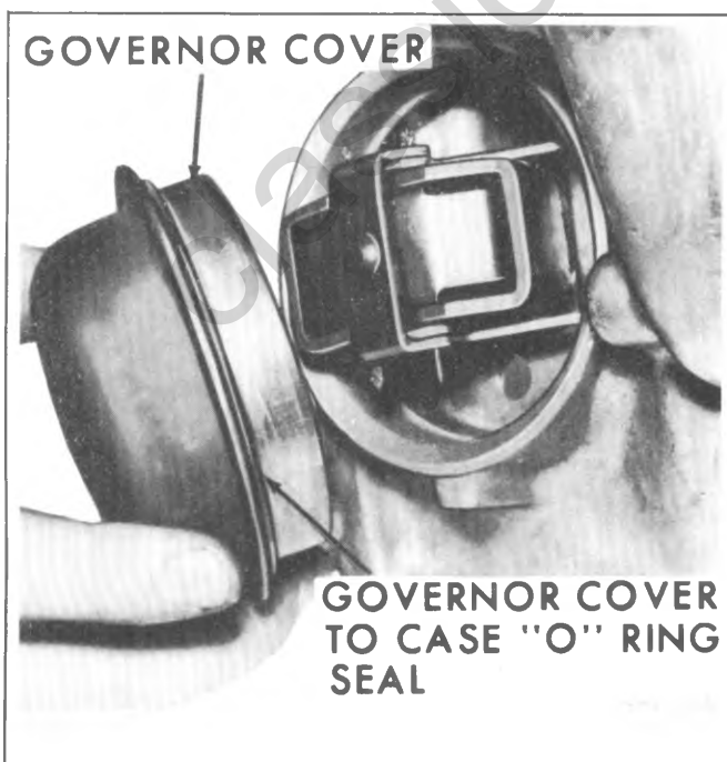
Fig. 7A-18--Governor Cover and O-Ring Seal
