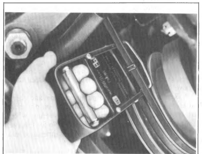
Fig. 3B-42--Checking Belt Tension with J-23600
