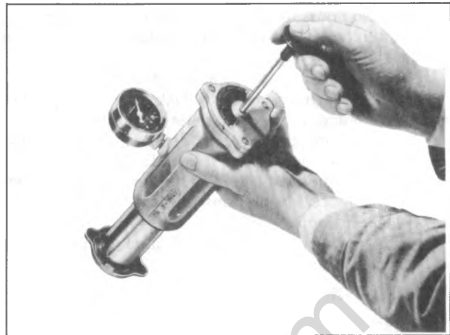
Fig. 6B-4--Pressure Checking Radiator Cap
