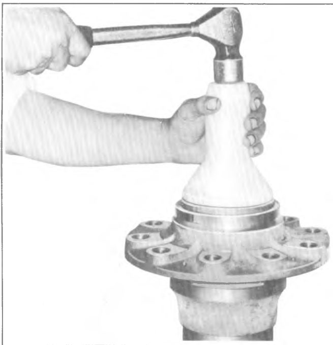
Fig. 4B-40--Installing Hub Oil Seal
