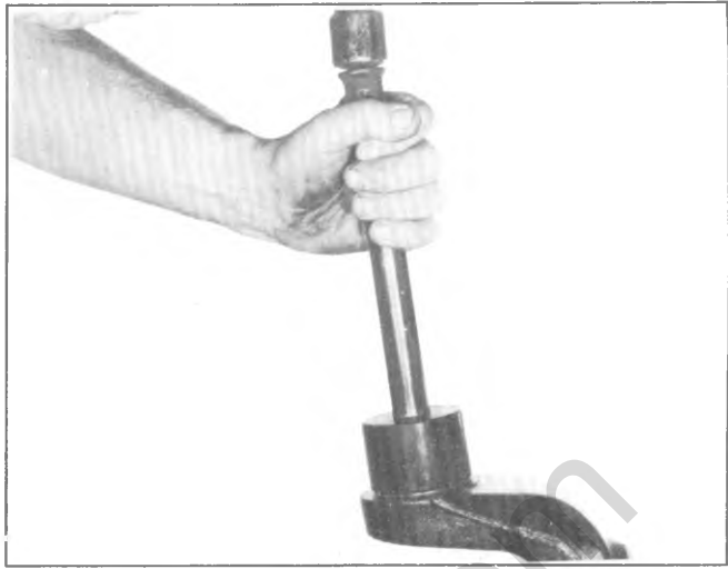
Fig. 3C-26K--Installing Oil Seal
