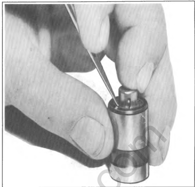
Fig. 6A1-14--Installing Ball Check Valve
