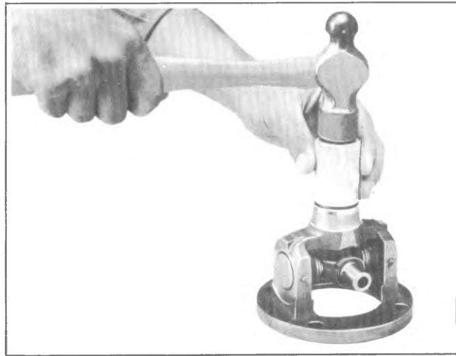
Fig. 4A-31--Installing Centering Ball Seal
