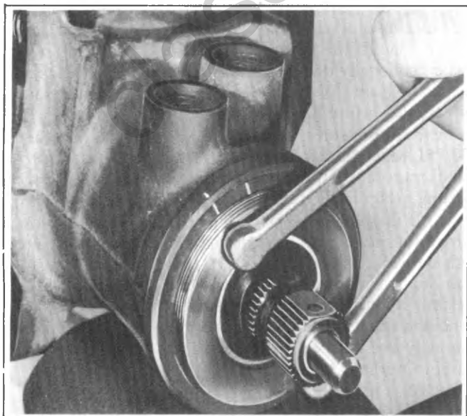
Fig. 3B-40--Align Hole With Second Mark
