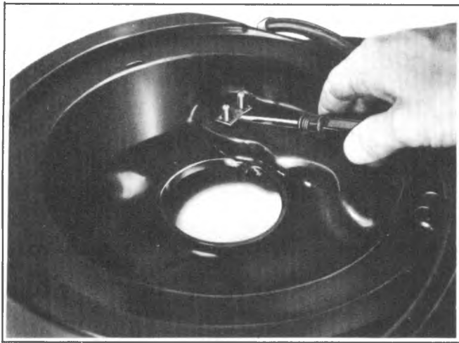
Fig. 6E-37--Removing Sensor Unit
