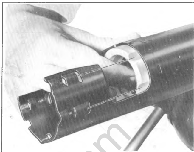
Fig. 3B-73--Installing Gearshift Housing Lower Bearing
