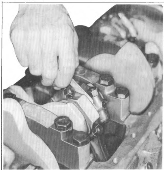
Fig. 6A2-55--Measuring Connecting Rod Side Clearance
