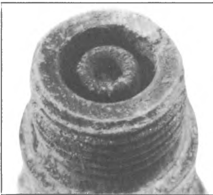
Insufficient Installation Torque
