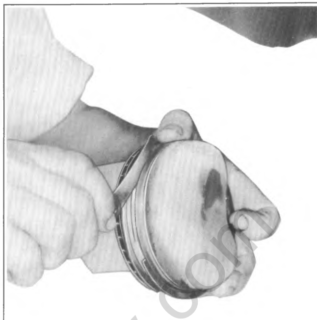
Fig. 6A1-44--Measuring Ring Groove Clearance
