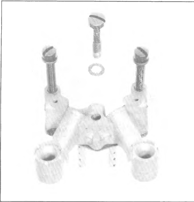
Fig. 6C1-24--Venturi Cluster Assembly
