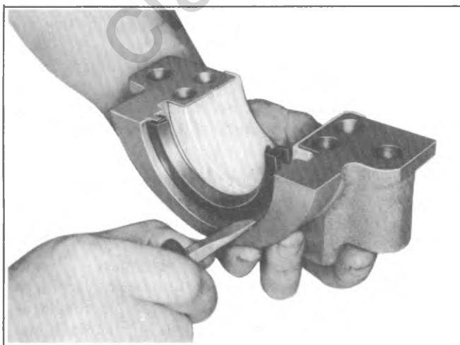
Fig. 6A2-60--Removing Oil Seal - Lower Half
