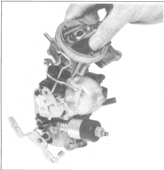
Fig. 6C-18--Air Horn Removal
