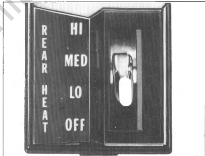
Fig. 1A-18--Auxiliary Heater Control
