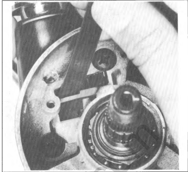
Fig. 3B-56--Lock Cylinder Removal
