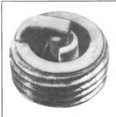
Heat Shock Failure
