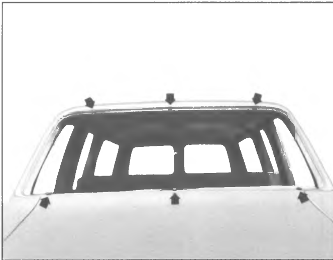
Fig. 2D-17-Checking Windshield Opening
