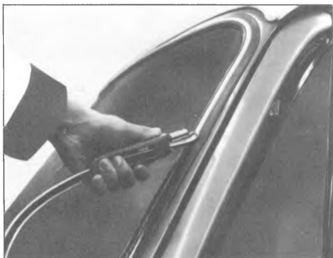
Fig. 2D-19--Installing Reveal Molding
