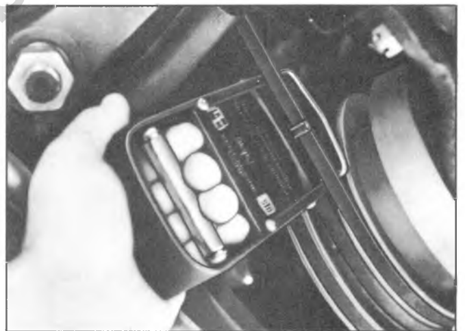
Fig. 3B-42--Checking Belt Tension with J-23600
