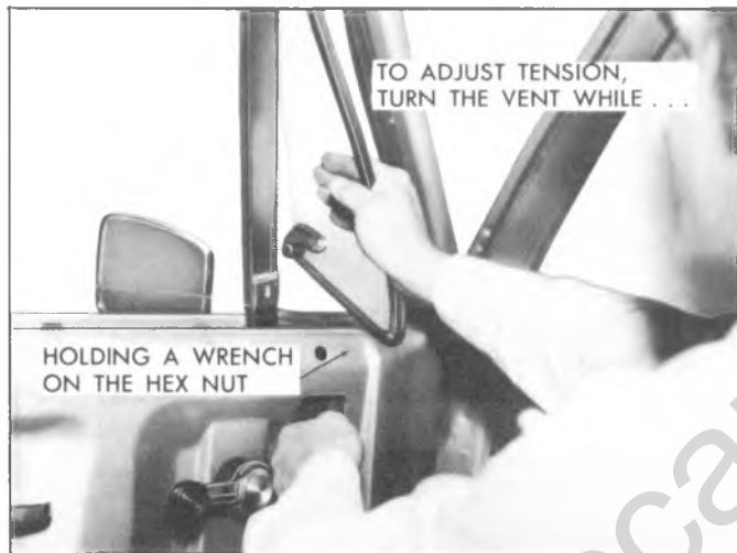
Fig. 2D-29--Adjusting Tension
