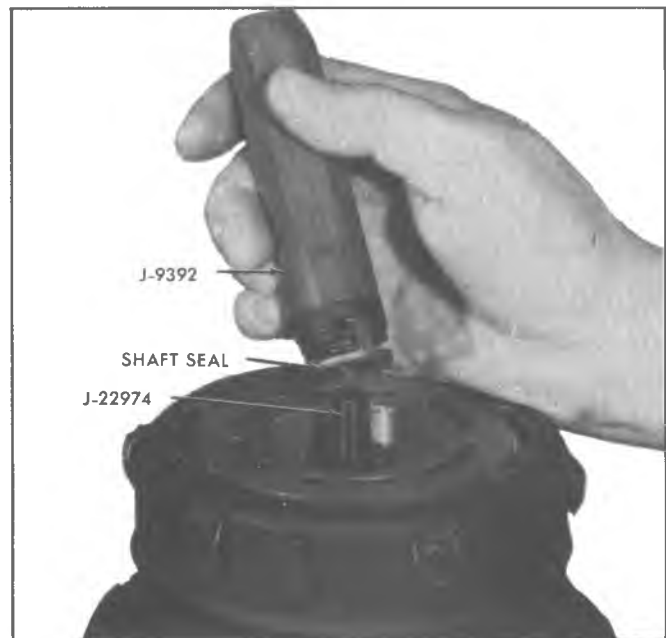
Fig. 8—Removing Shaft Seal
