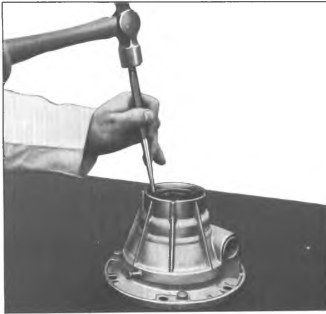
Fig. 6F—Removing Rear Output Shaft Front Bearing
