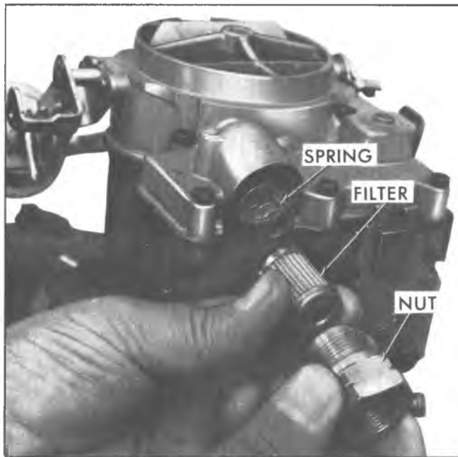
Fig. 34—Fuel Filter Replacement
