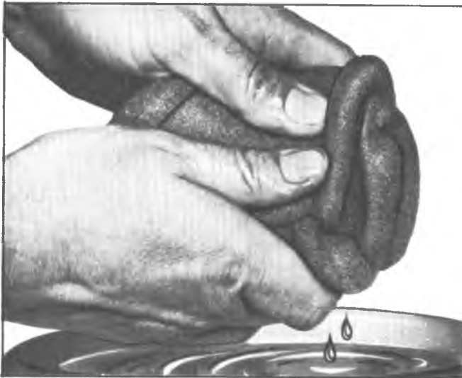
Fig. 70—Cleaning Polywrap Band
