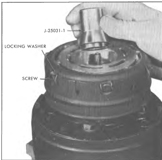
Fig. 11—Installing Rotor and Bearing Puller Guide
