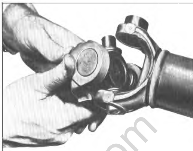
Fig. 4—Installing Trunnion into Yoke
