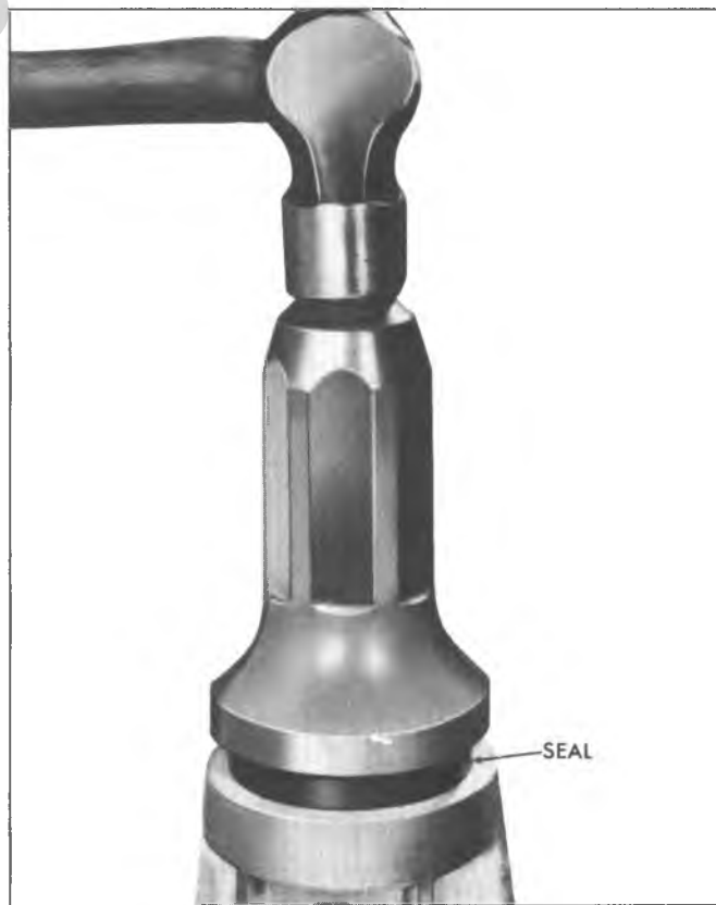
Fig. 15B—Installing Extension Oil Seal (Typical)
