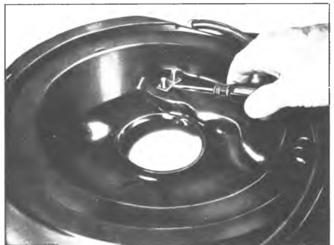
Fig. 78—Removing Sensor Unit
