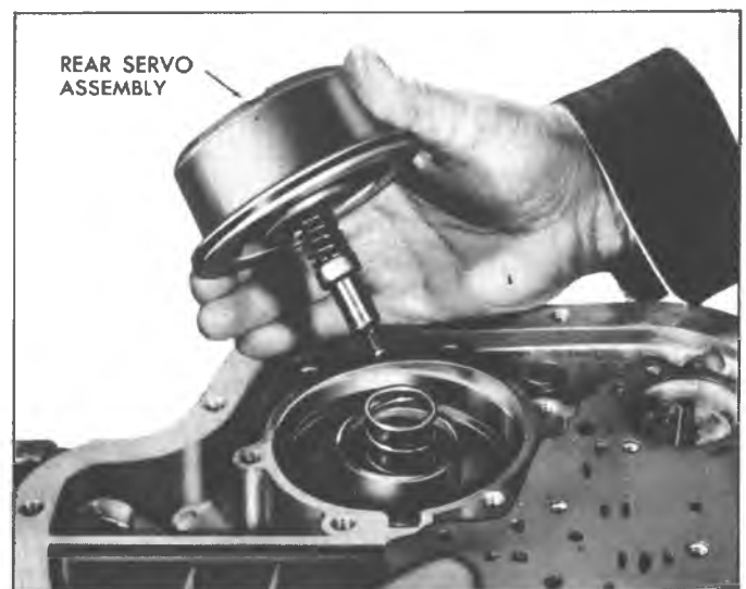
Fig. 1B—Removing Rear Servo Assembly
