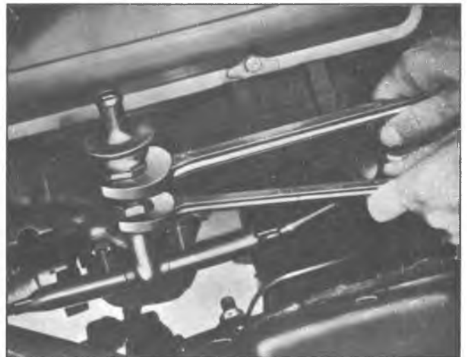
Fig. 21f—Removing Check Valve
