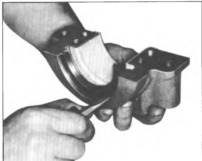
Fig. 10V—Removing Oil Seal (Lower Half)
