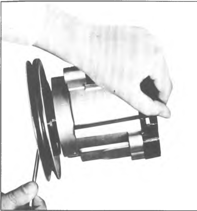
Fig. 16f—Installing Centrifugal Filter
