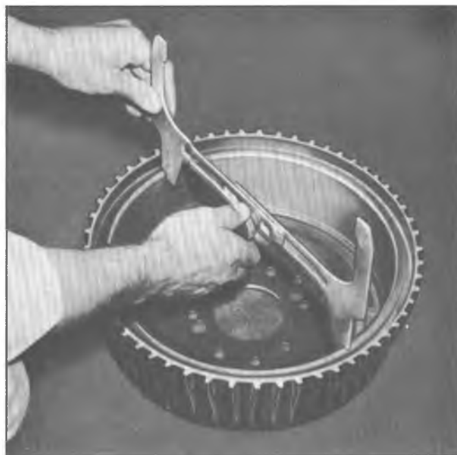
Fig. 39--Using Drum-to-Brake Gauge J-21177 or J-22364
