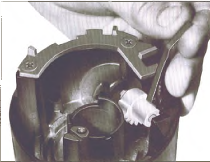
Fig. 70—Installing Rack Preload Spring
