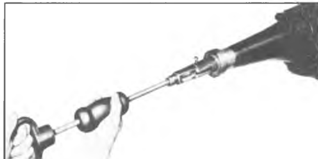
Fig. 27—Removing Mainshaft Rear Oil Seal
