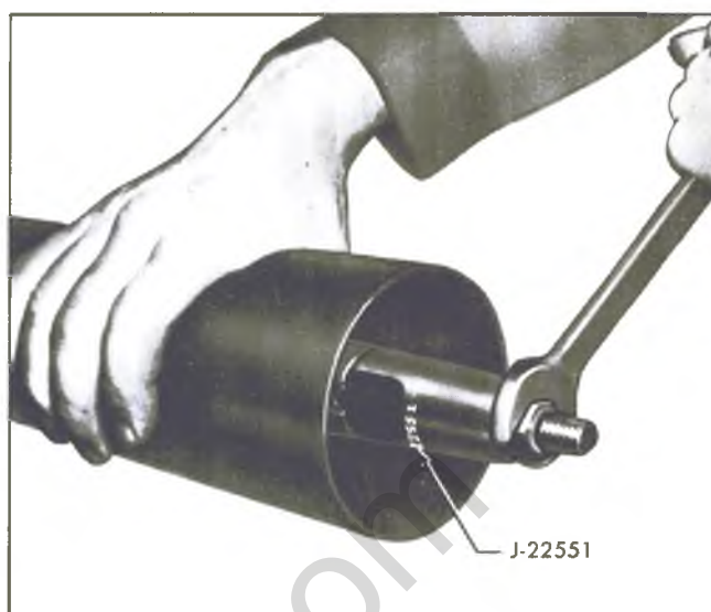
Fig. 97—Removing Shift Tube Assembly
