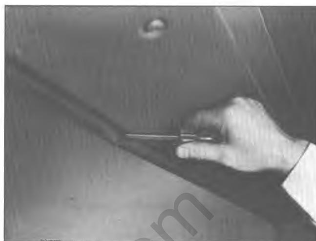
Fig. 15—Assisting Weatherstrip over Flange
