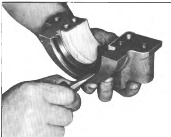
Fig. 11L—Removing Oil Seal (Lower Half) Typical
