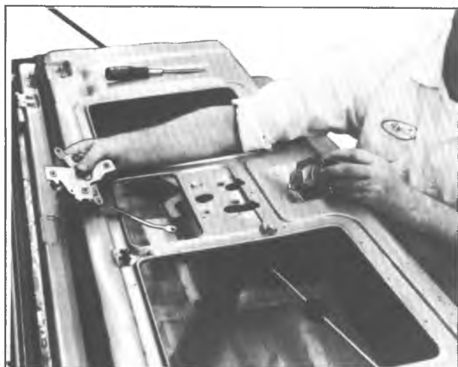
Fig. 64—Removing Control Assembly and Inside Handle
