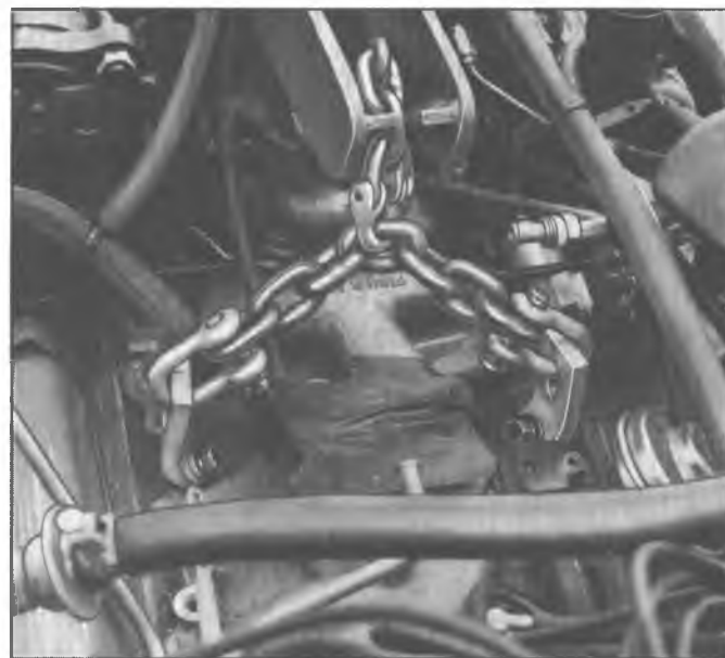
Fig. 3V—Tool J-24680-1 Installed on Engine
