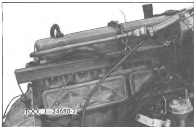
Fig. 3L—Tool J-24680-2 Installed on Engine
