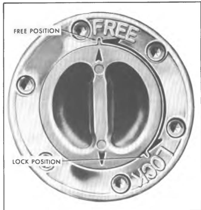
Fig. 53—Hub Key Position — Typical
