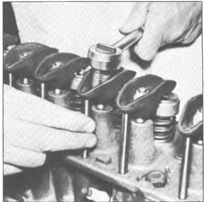
Fig. 21—Valve Adjustment (L6 Engine)
