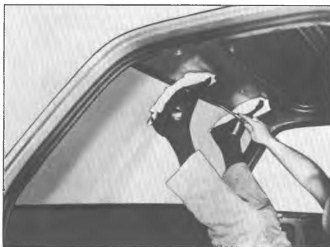
Fig. 14—Applying Pressure to Windshield
