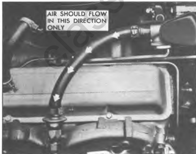
Fig. 20f—Air Flow Through Check Valve
