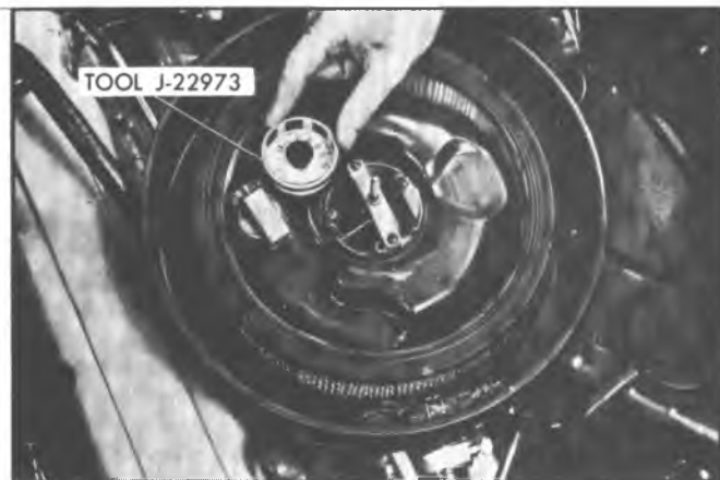
Fig. 12A--Temperature Gauge Installation
