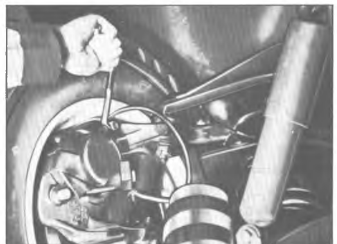
Fig. 29--Bleeding Brakes with Tool J-21472
