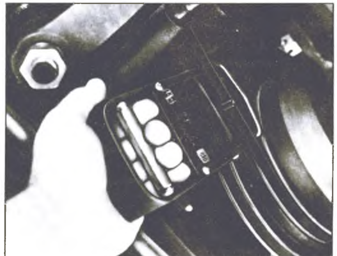
Fig. 40—Checking Belt Tension with J-23600
