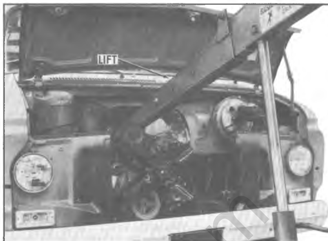
Fig. 4L—Lifting Device Installed to J-24680-2
