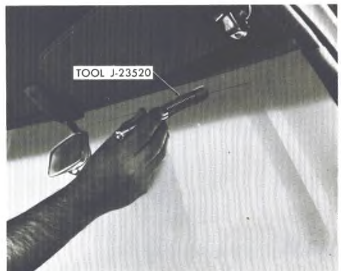
Fig. 7--Testing Windshield Antenna (Typical)
