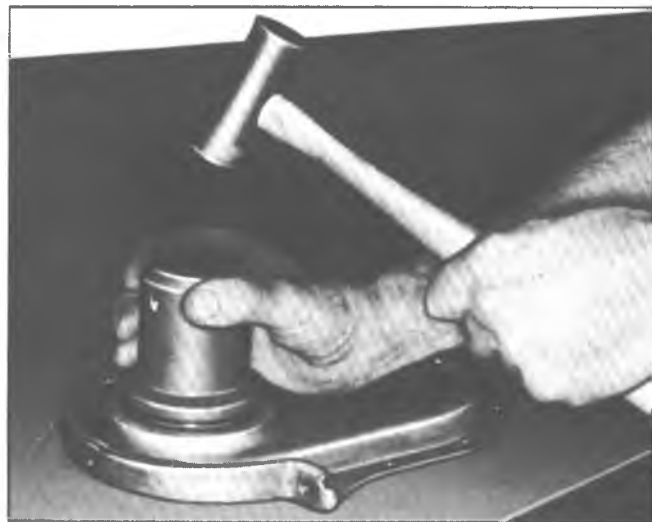
Fig. 19V—Installing Oil Seal (Cover Removed)
