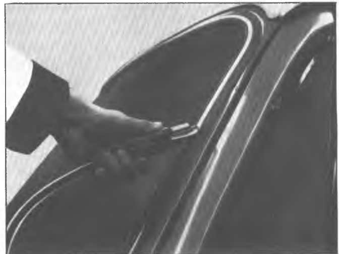
Fig. 19—Installing Reveal Molding
