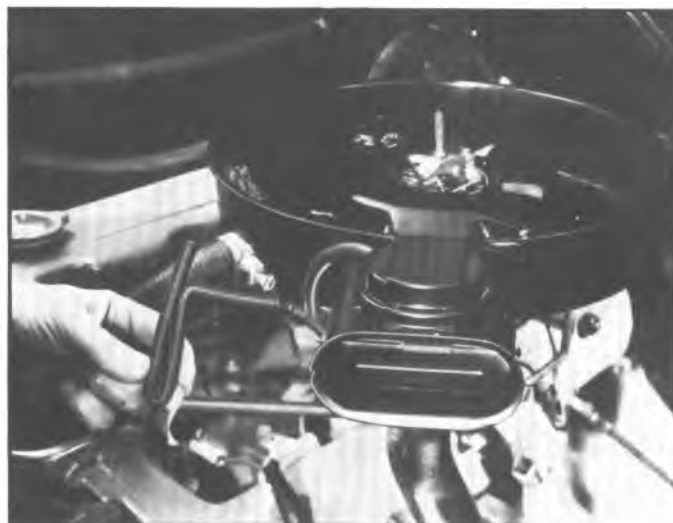
Fig. 8b—Checking Vacuum Diaphragm
