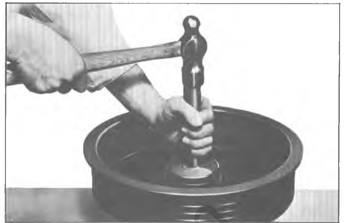
Fig. 75—Installing Hub Inner Bearing Cup
