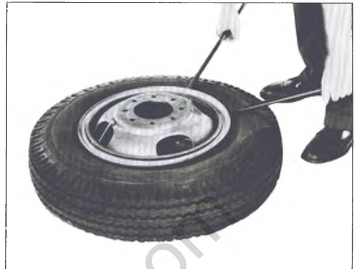
Fig. 5—Loosening First Bead
