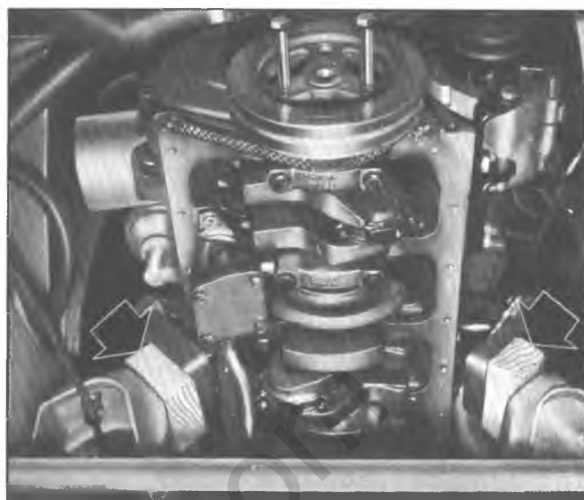
Fig. 8L—Engine Blocked for Oil Pan Removal
