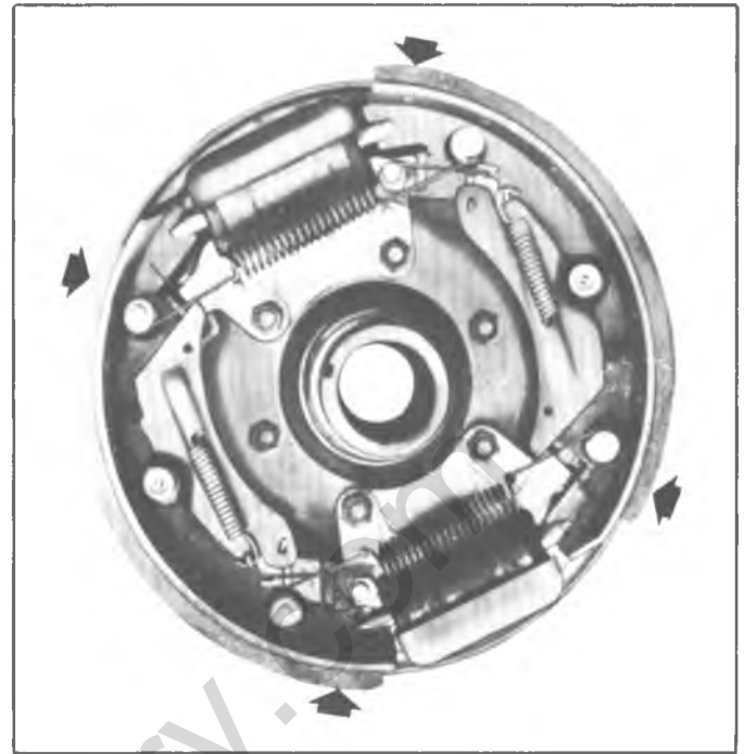
Fig. 79--Measuring Points for Shoe Centering
