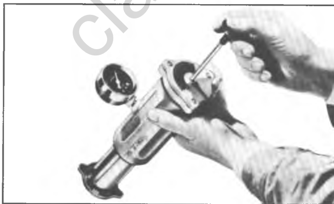
Fig. 10—Pressure Checking Radiator Cap
