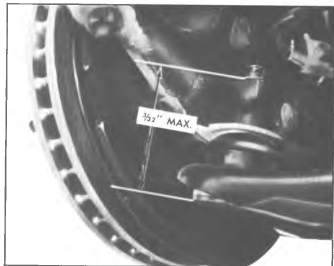
Fig. 35—Checking Lower Ball Joint
