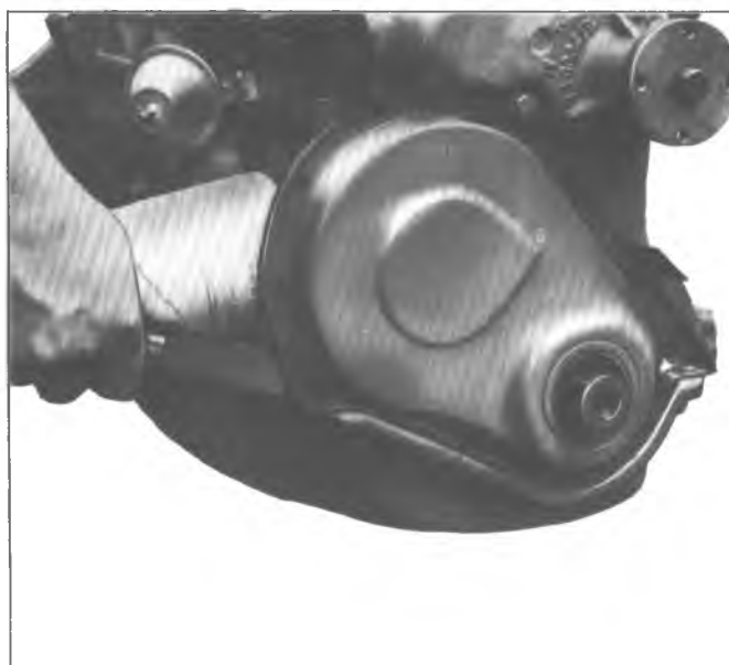
Fig. 18L—Cutting Tabs on Oil Pan Front Seal
