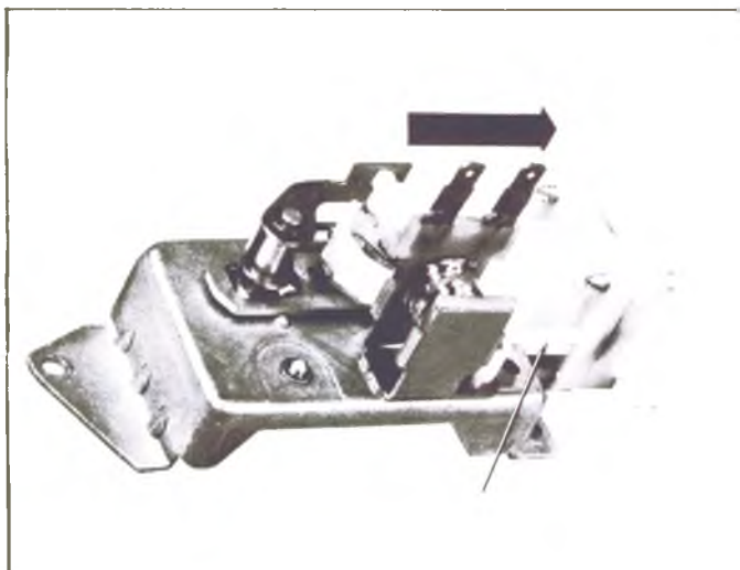
Fig. 48--Releasing Pump From Lockout Position
