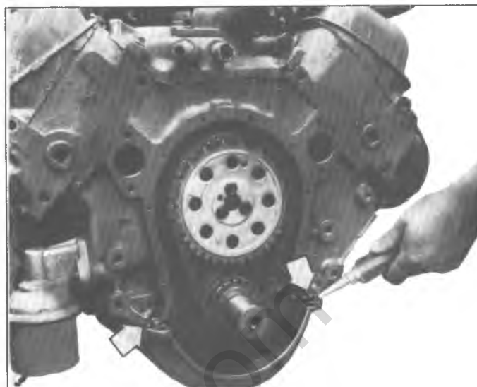
Fig. 18V—Applying Front Cover Sealer
