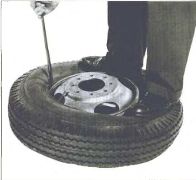
Fig. 11—Applying Second Bead
