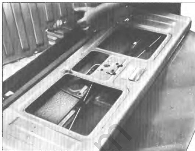
Fig. 58—Removing Access Cover (14)
