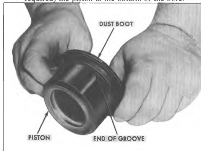
Fig. 61--Installing Boot to Piston
