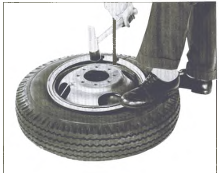
Fig. 13—Forcing Ring into Gutter
