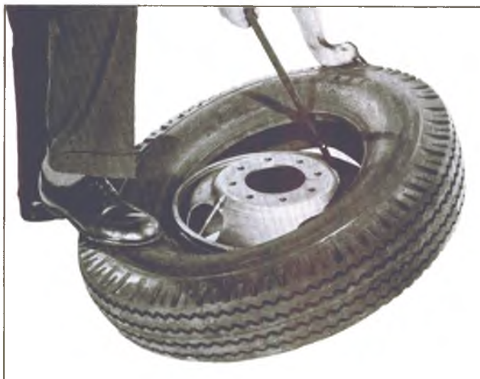
Fig. 10—Mounting First Bead
