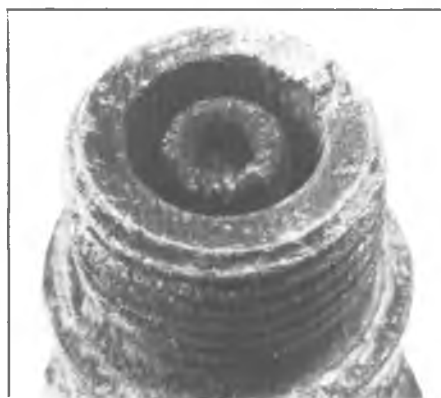
Insufficient Installation Torque
