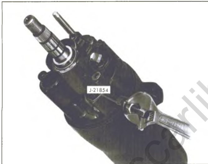
Fig. 75—Removing Bearing Housing Pivot Pins
