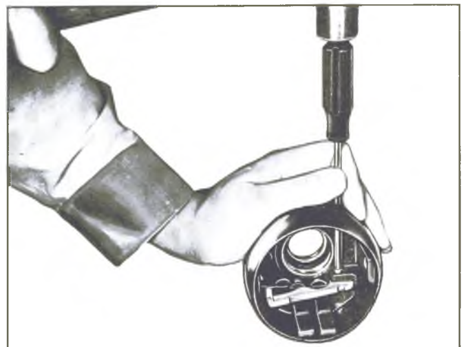
Fig. 94—Removing Release Lever Pivot Pin
