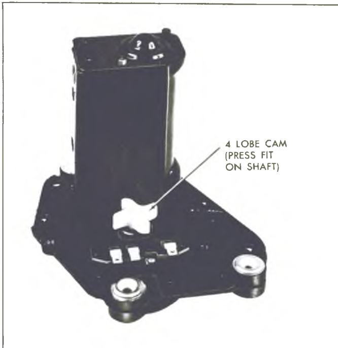
Fig. 44--Washer Pump Drive Cam
