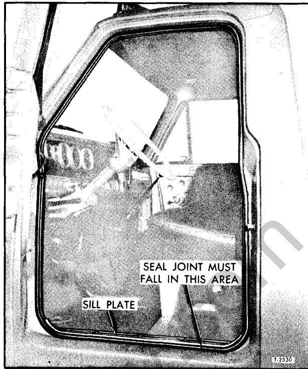
Figure 13—Door Weatherstrip Installed
