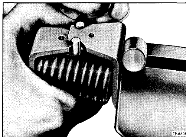
Figure 28—Disassembling Torsion Spring From Lever
