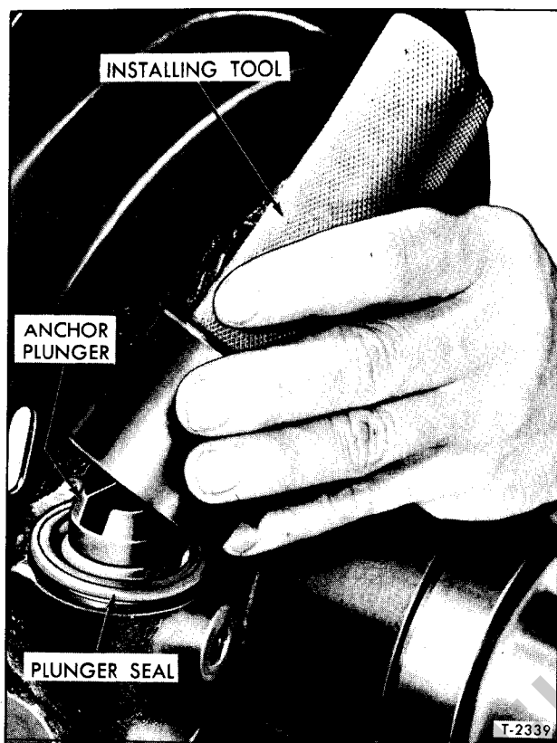
Figure 33—Installing Anchor Plunger and Seal
