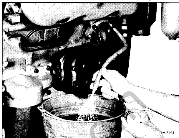
Figure 4—Fuel Flow Test
