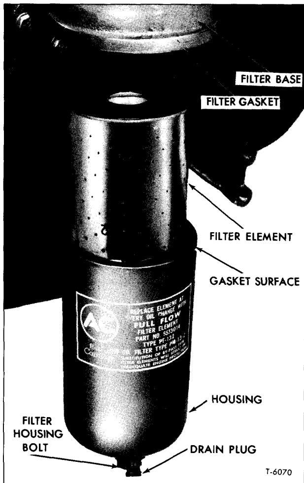
Figure 10—Oil Filter Element (Typical)
