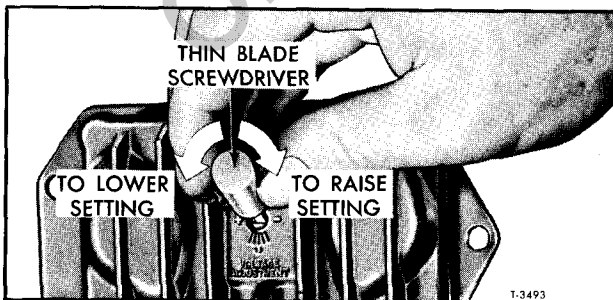
Figure 16—Adjusting Voltage Setting (Typical)
