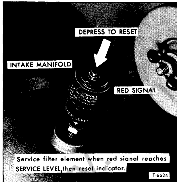
Figure 12—Air Filter Restriction Indicator
