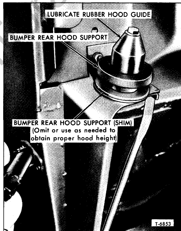
Figure 15—Hood Mounting Adjustment at Cab Cowl (M and C Models Shown)
